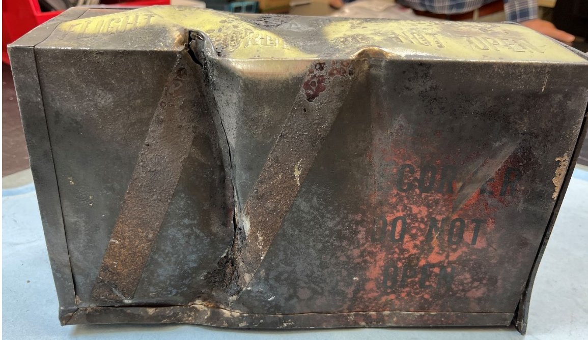
Figure 1. Damaged exterior of CVR.
