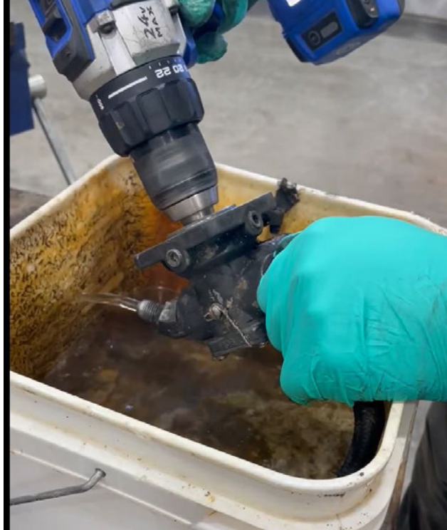
Figure 12 Fuel pump operational test.
