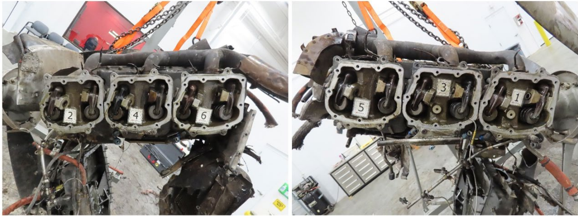
Figure 11 Both sides of engine with valve covers removed.
