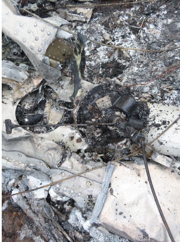
Figure 6 Fuel selector on site.
