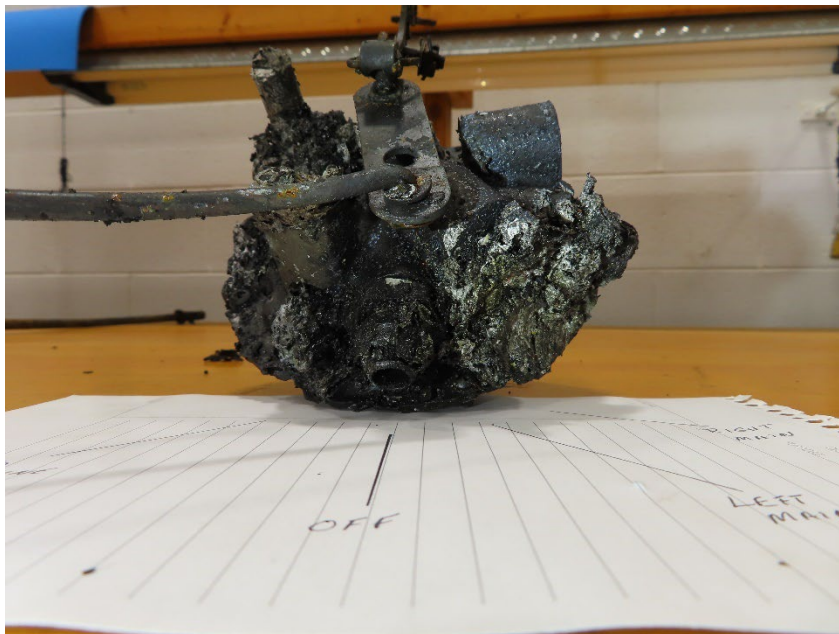
Figure 7 Fuel selector during examination.
