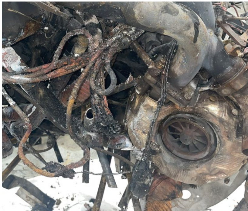
Figure 14 View of turbo prior to removal.
