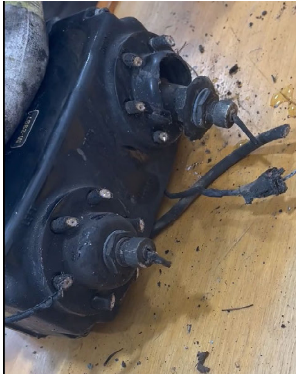
Figure 8 Dual magneto during operational test.
