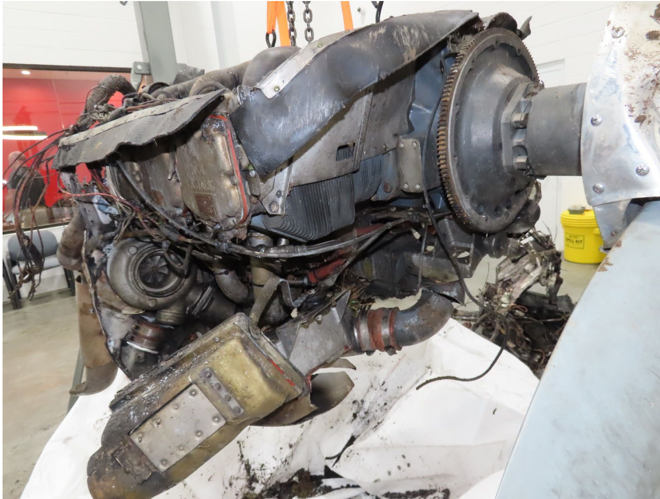
Photograph 7 - Overall engine condition after recovery. Note turbo condition. (NTSB)
