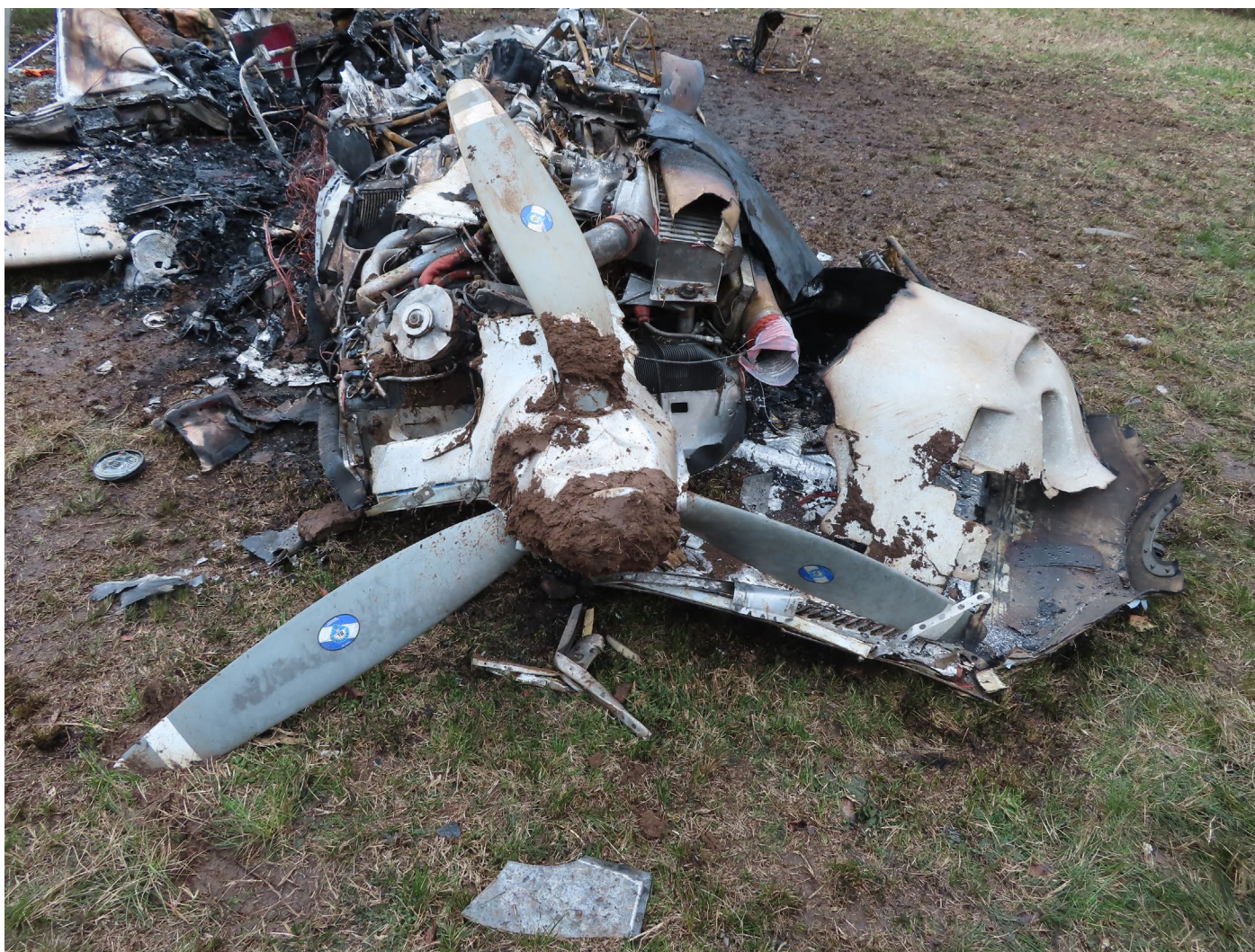
Photograph 6 - Closeup view of propeller damage. (NTSB)
