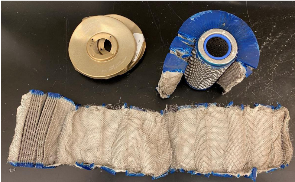
Disassembly of Engine 1 fuel filter soaking
