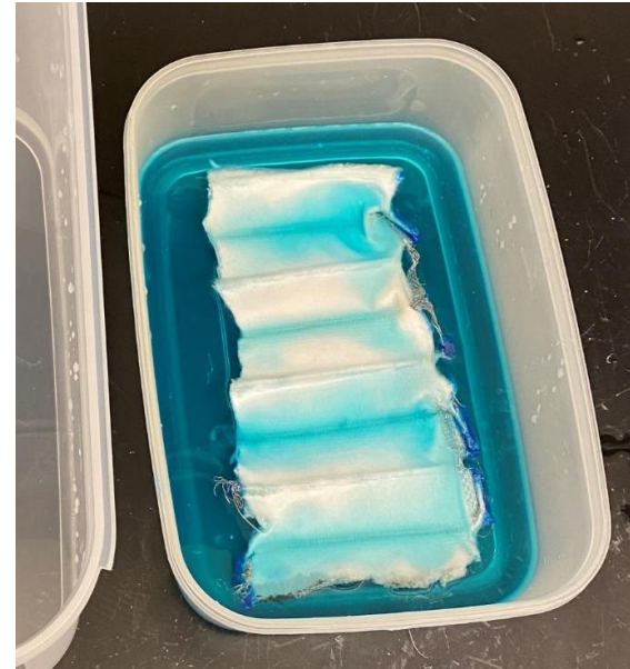
Engine 1 fuel filter soaking in copper sulfate bath
