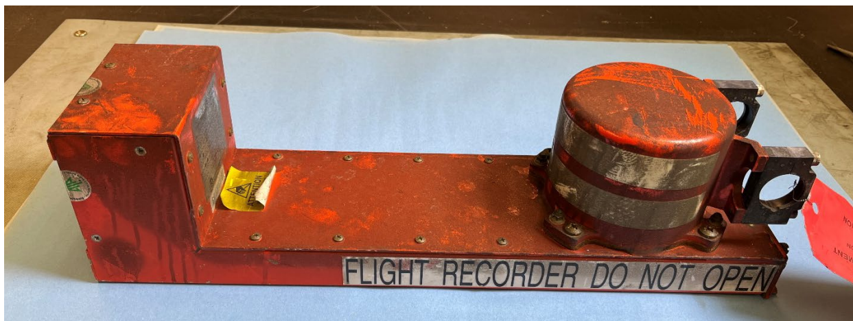
Figure 1. Exterior of flight data recorder exhibiting sooting.
