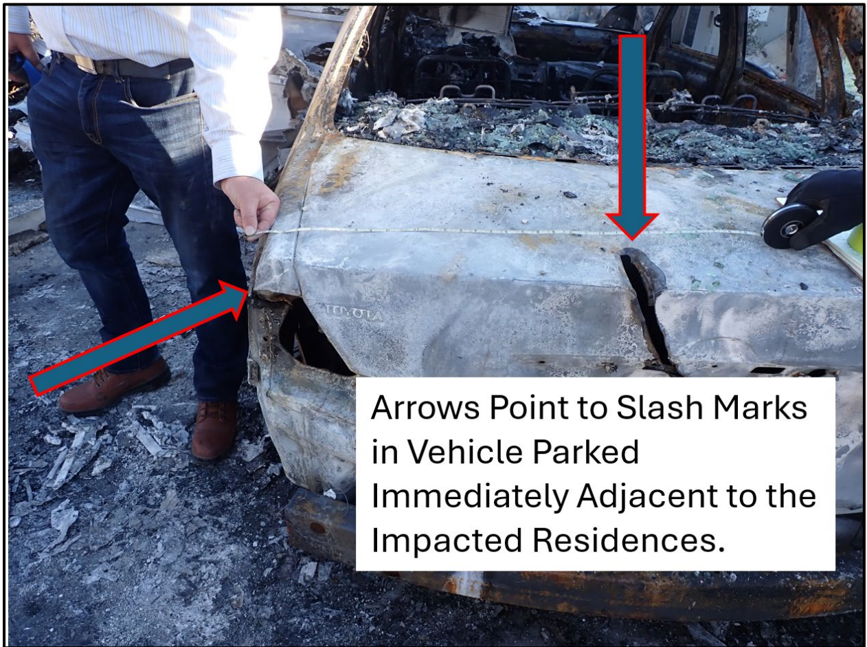
Figure 1 Annotated Picture Showing the 2 Parallel Slash marks in a Vehicle
