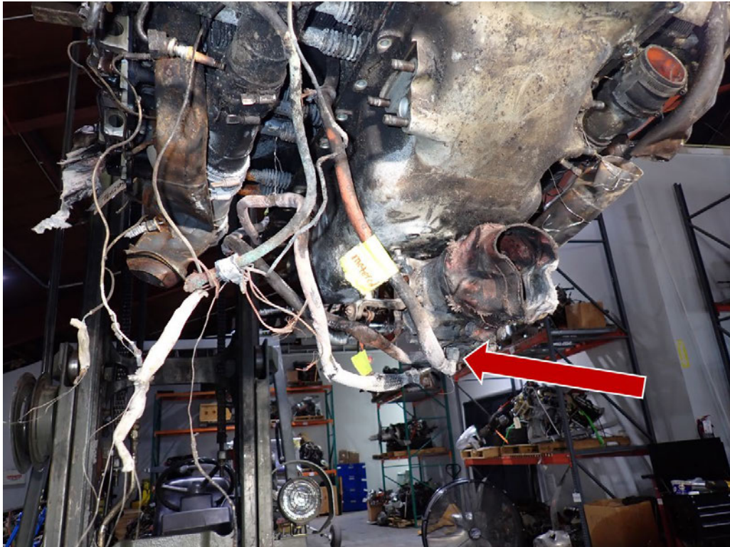
Figure 9 Arrow Points to Fractured Outlet Fitting of the Metering Valve and the Attached Flexible Metered Fuel Hose
