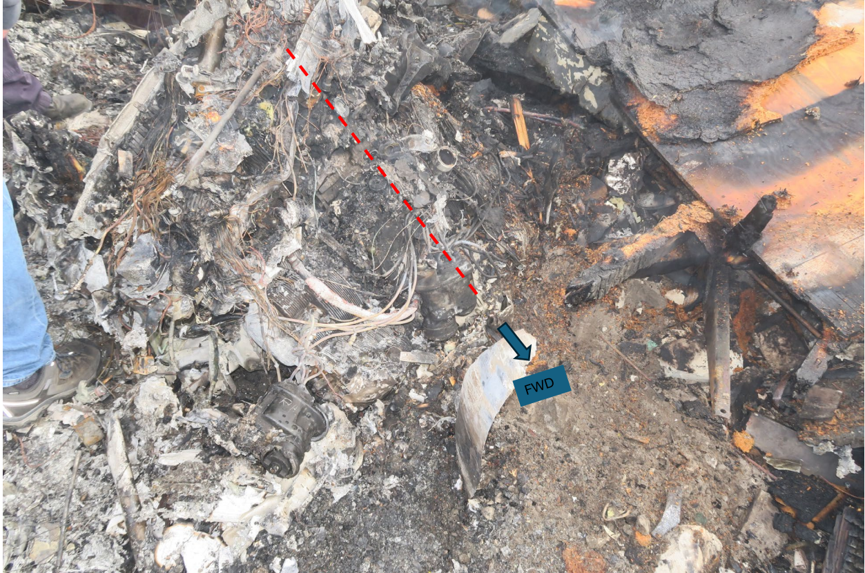
Figure 4. Aircraft engine after some of the building debris was removed. The underside of the sheathing that had been on top of the right side of the engine is visible in the top right of the photo. Engine centerline denoted by dashed red line.
