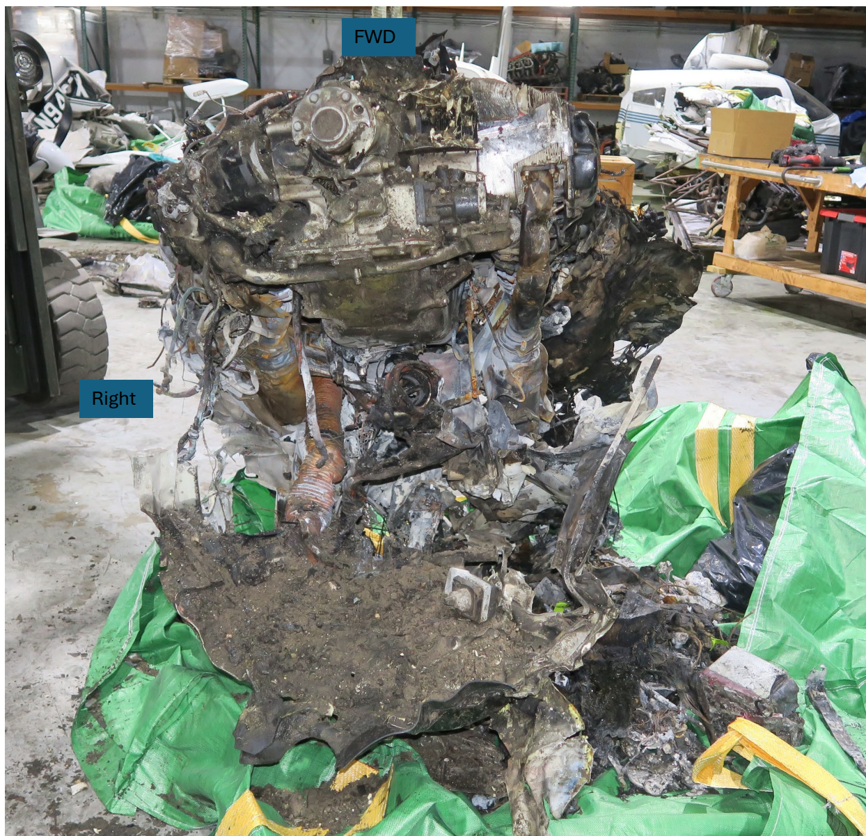
Figure 7. Forward/underside view of the engine with the cowling separated. The interior surface of the cowling contained dirt.
