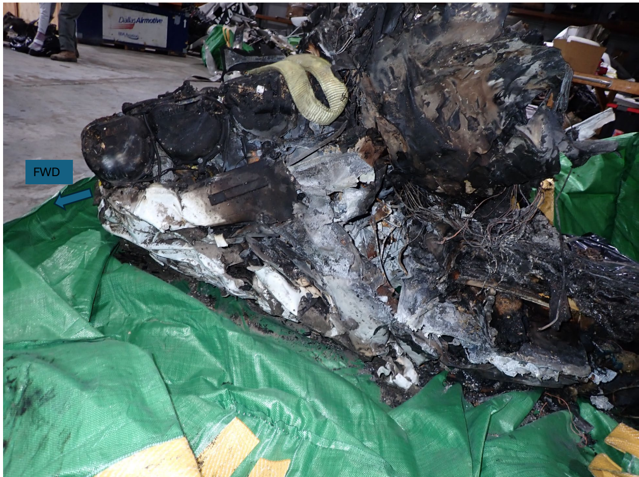
Figure 6. View of the left side of the engine and lower cowling. There is a sharp demarcation between the areas exhibiting clean burn, sooting and undamaged cowl.
