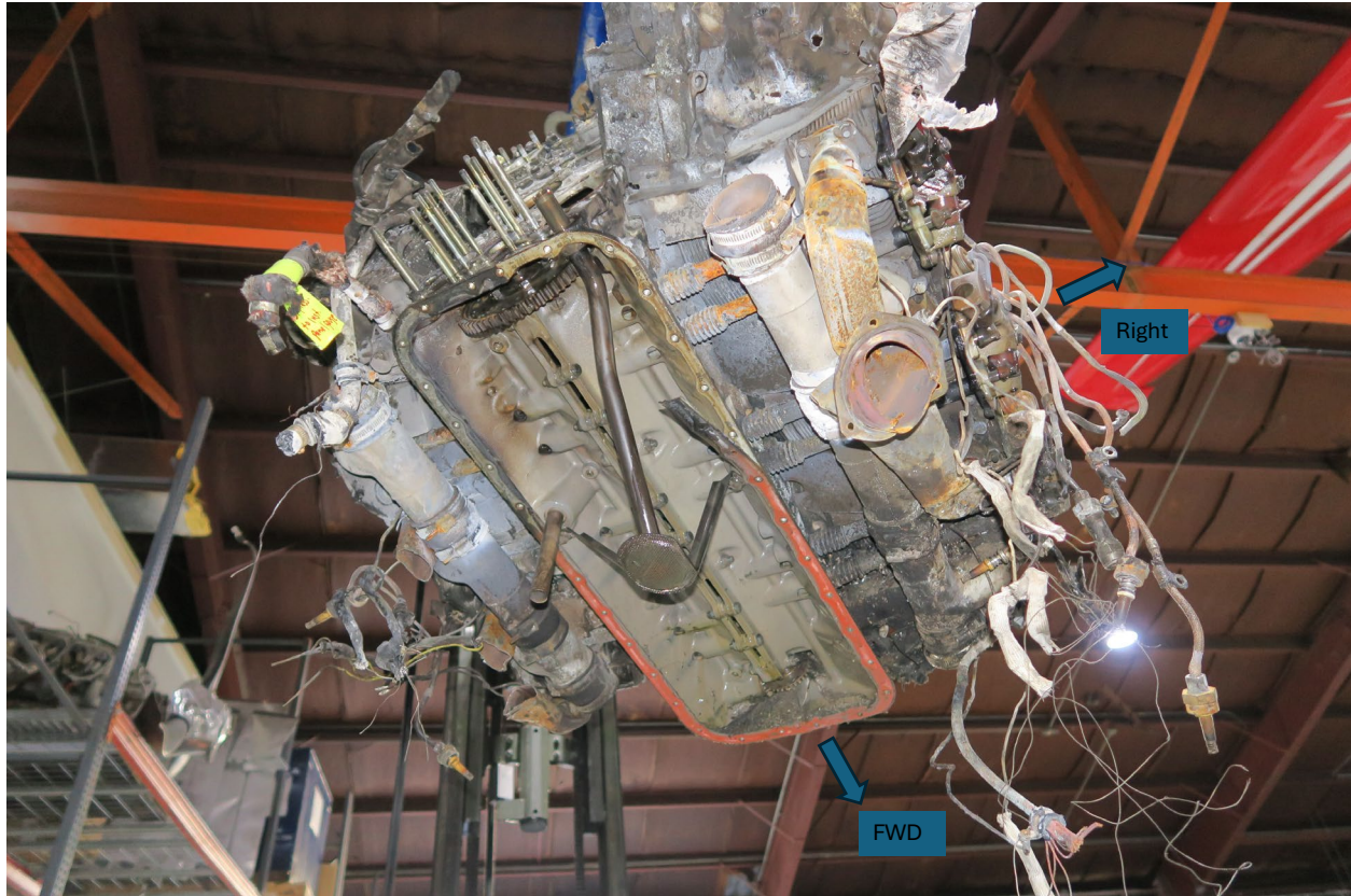
Figure 10. Underside of the crankcase with the oil sump cover removed. Sealing gasket thermally damaged and or consumed along the aft left and right areas.
