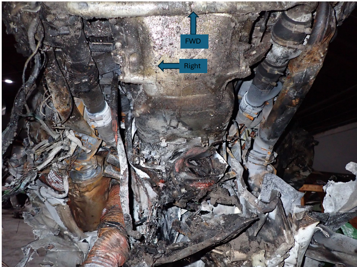
Figure 8. Underside of the engine looking from the front. An area of clean burn encompasses the aft portion of the oil sump cover, exhaust components on both sides and the throttle body and metering valve in the center.
