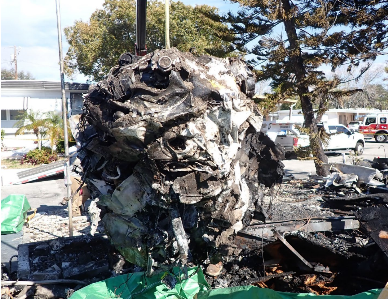
Figure 5. Aircraft engine being hoisted up during wreckage recovery. Lower engine cowlings are pressed against the engine.
