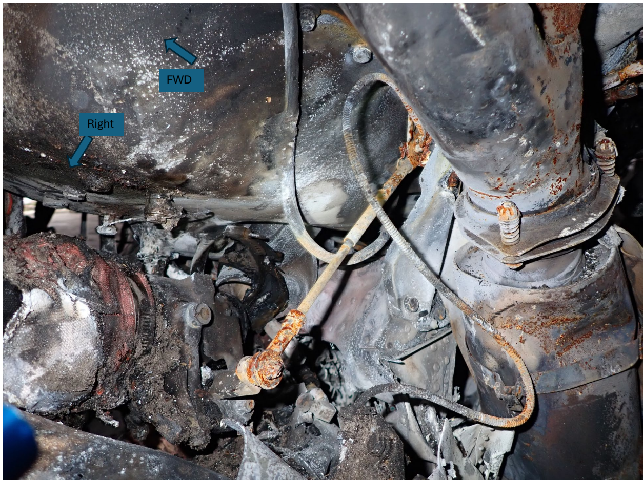
Figure 9. Close up view of the throttle body and metering valve below the oil sump cover.
