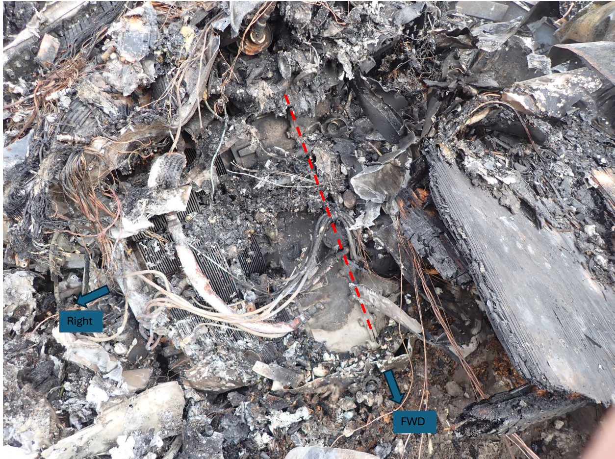
Figure 3. Aircraft engine as found among the building debris. A portion of sheathing is covering the left bank cylinders. The dashed red line denotes the engine's centerline.
