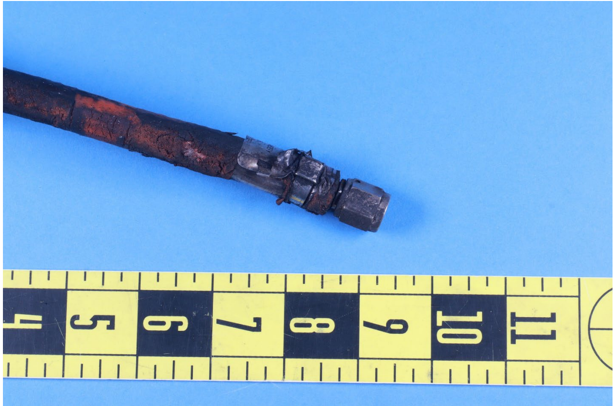
Figure 2. Fuel manifold end of the flexible fuel hose.
