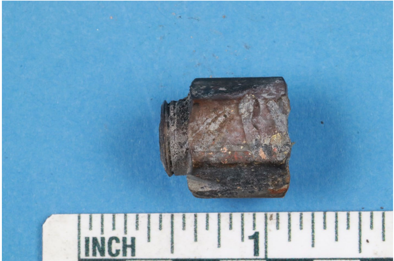
Figure 5. Deformation of female threaded nut consistent with impact forces.
