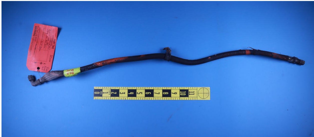
Figure 1. Metered fuel hose and fittings as received.
