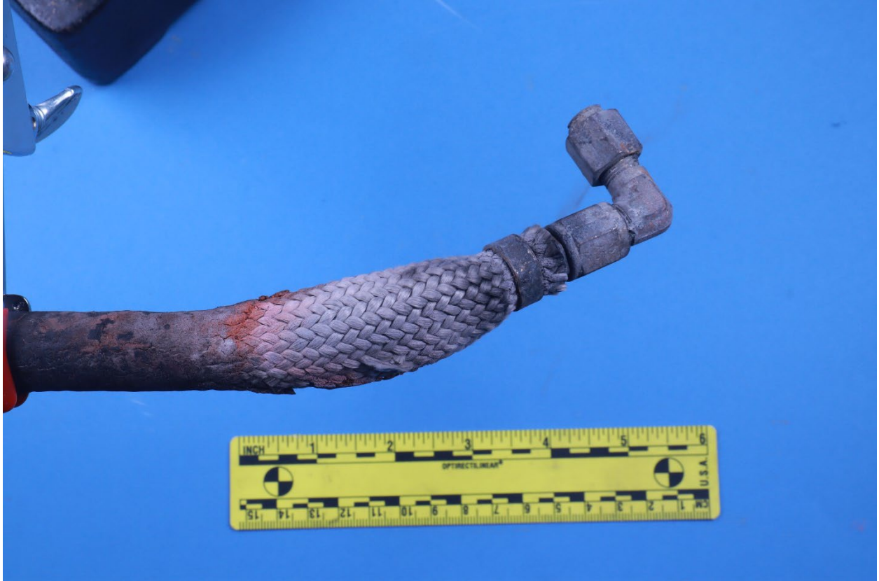
Figure 3. Fuel metering valve end of the flexible fuel hose. Localized thermal damage to the fire sleeve.
