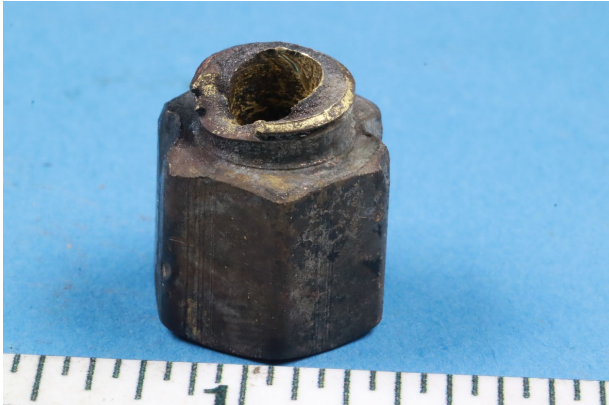
Figure 6. Fracture surface on male threaded portion of the fitting.
