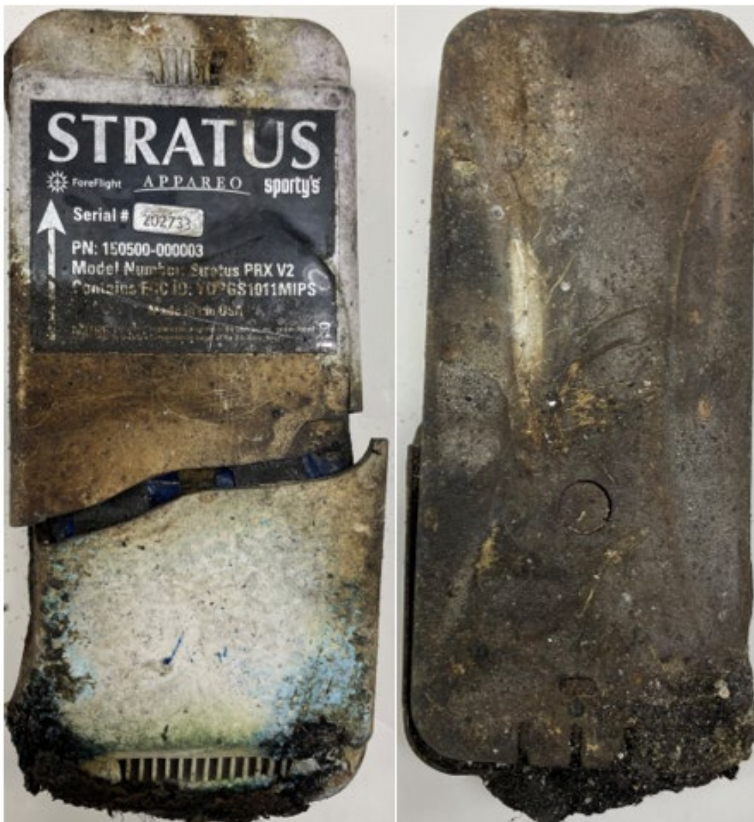
Figure 1. Appareo Stratus PRX V2 front (left) and back (right) as received by the Vehicle Recorder Lab.
