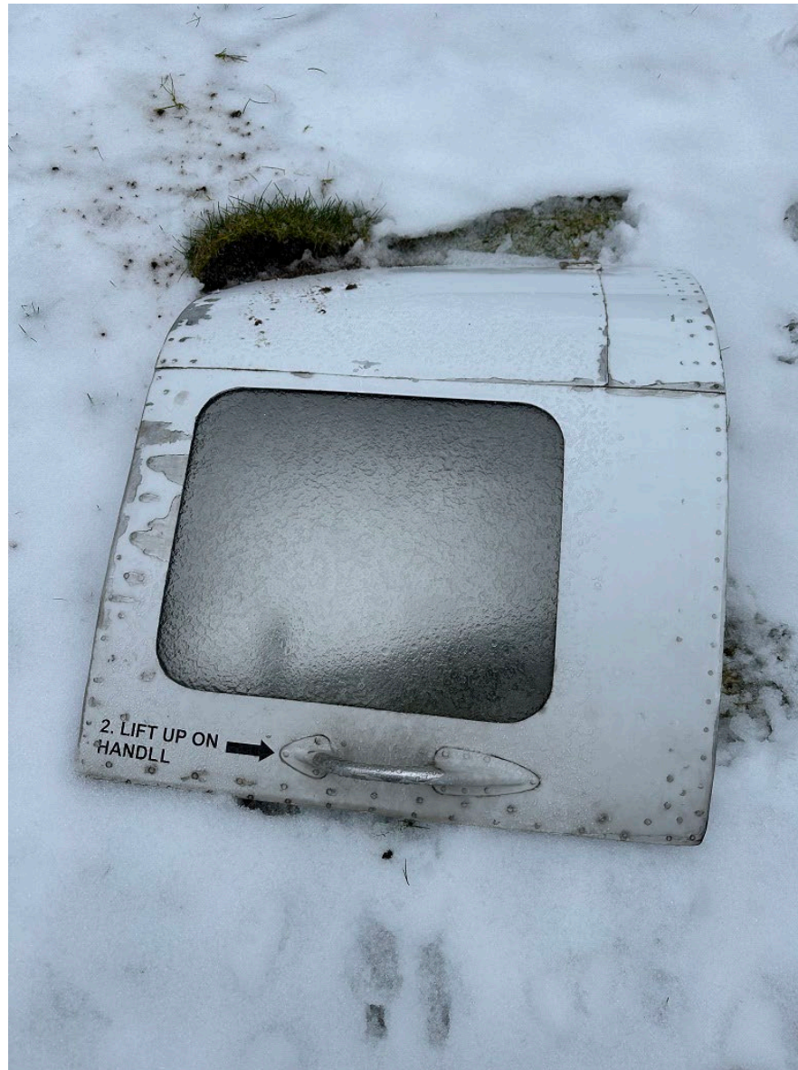
Photograph 2 - Separated Cockpit Door/Hatch as Found (Courtesy of TSA)
