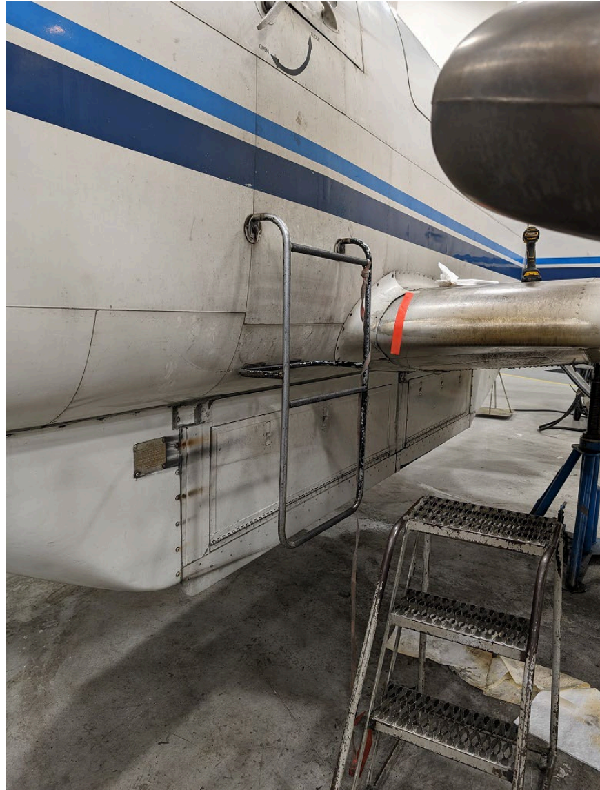
Photograph 4 - Exemplar Portable Ladder And Cockpit Door/Hatch (Courtesy of Wiggins)
