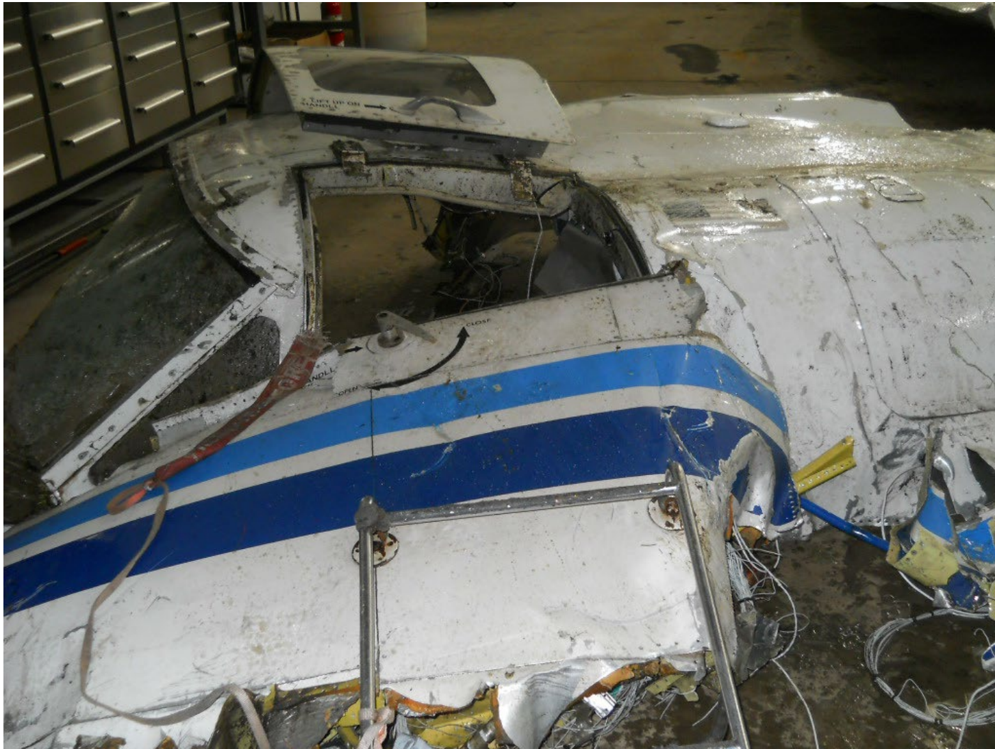
Photograph 5 - Cockpit Door/Hatch And Ladder Staged at Exam
