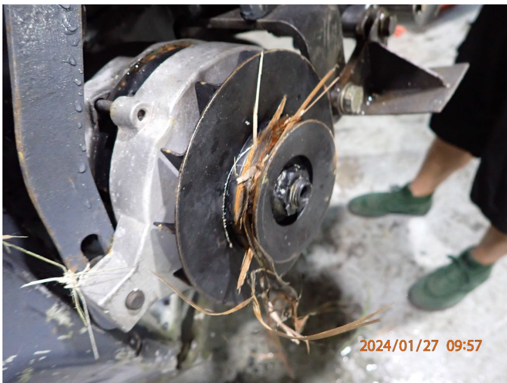
Photo 33: View of organic debris in the alternator pulley.
