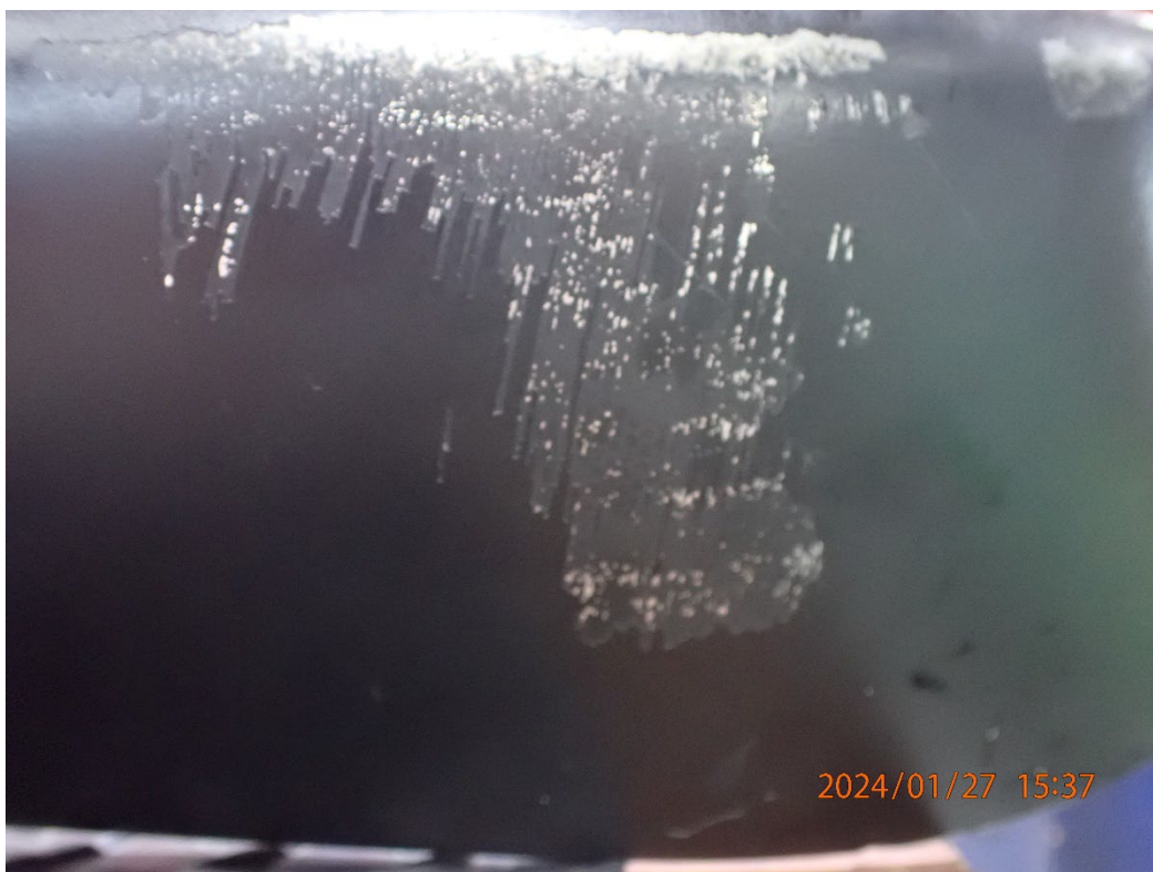
Photo 54: Chordwise scratching on blade B.
