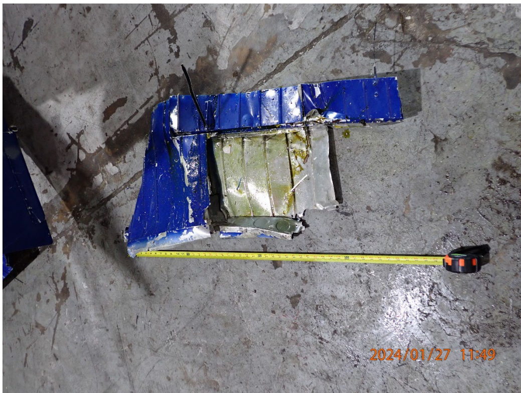
Photo 9: View of the impact separated portion of the right elevator and the elevator trim tab.
