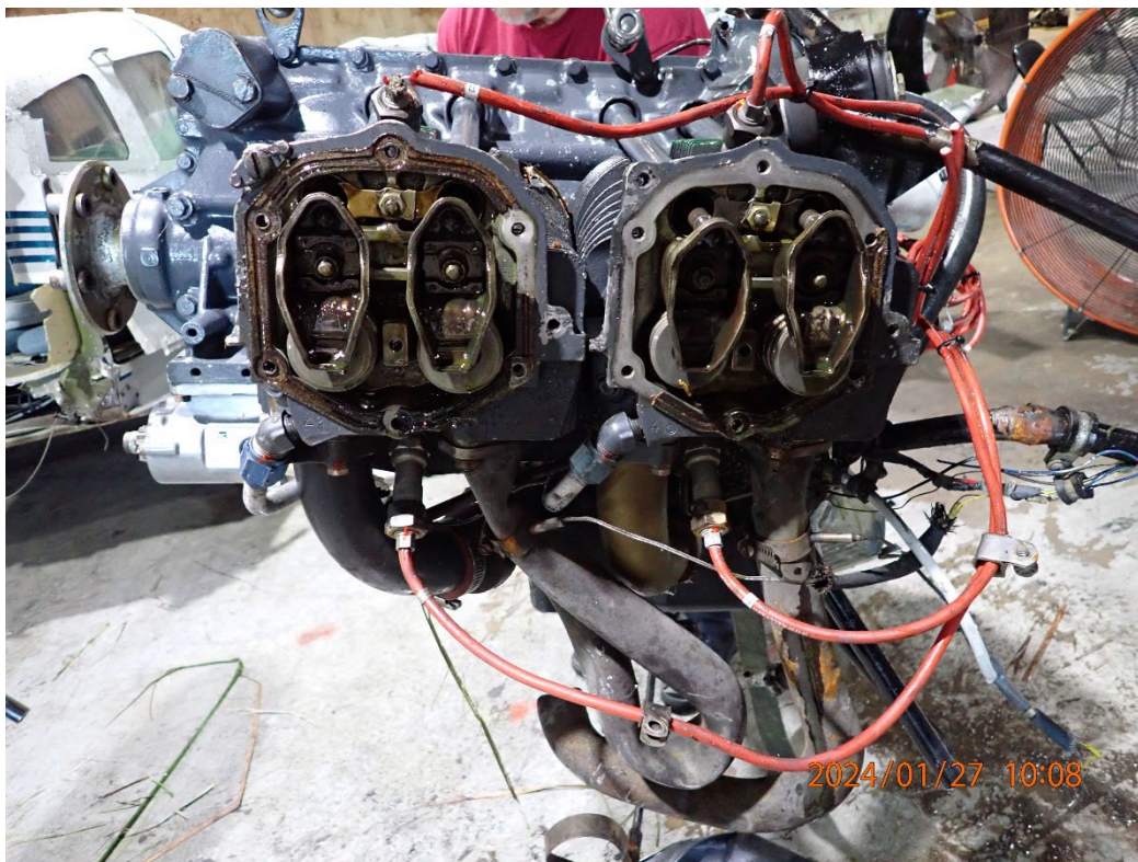
Photo 37: View of damage to the No. 2 top spark plug lead.
