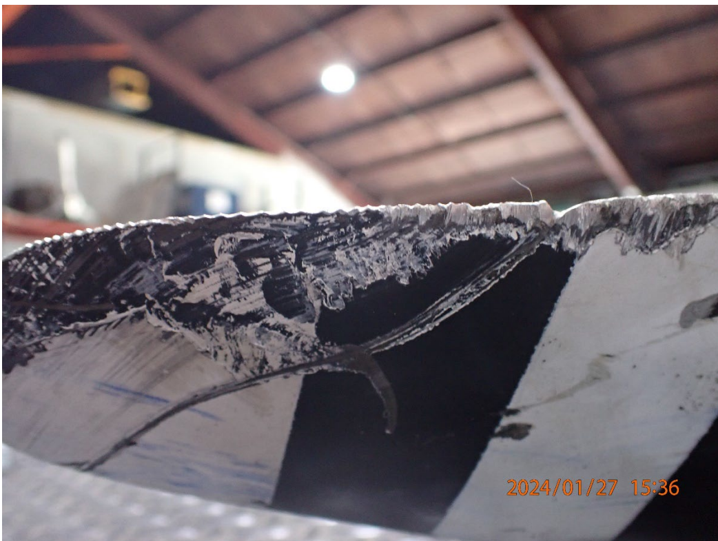
Photo 52: Trailing edge of blade A.
