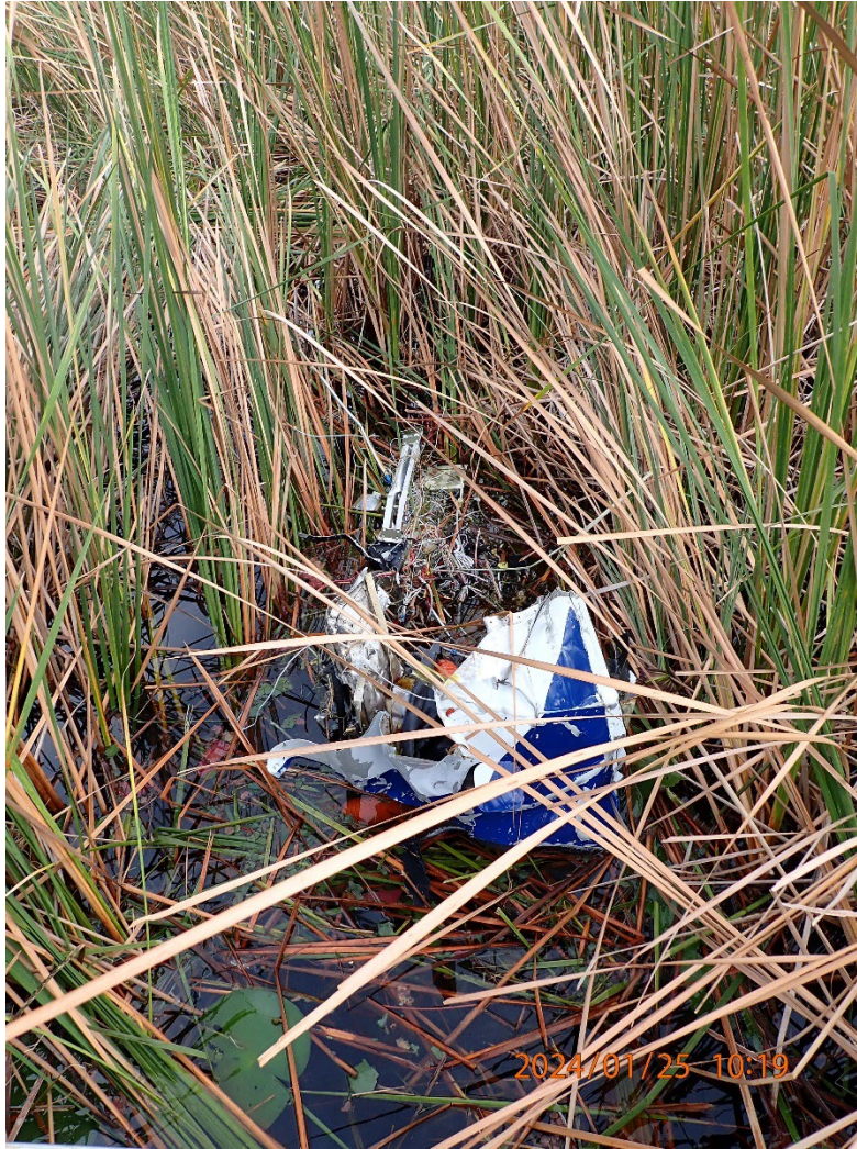
Photo 3: View of the instrument panel impact separated from the fuselage.
