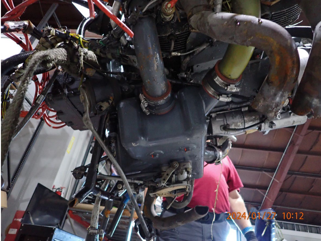
Photo 45: View of undamaged oil sump.
