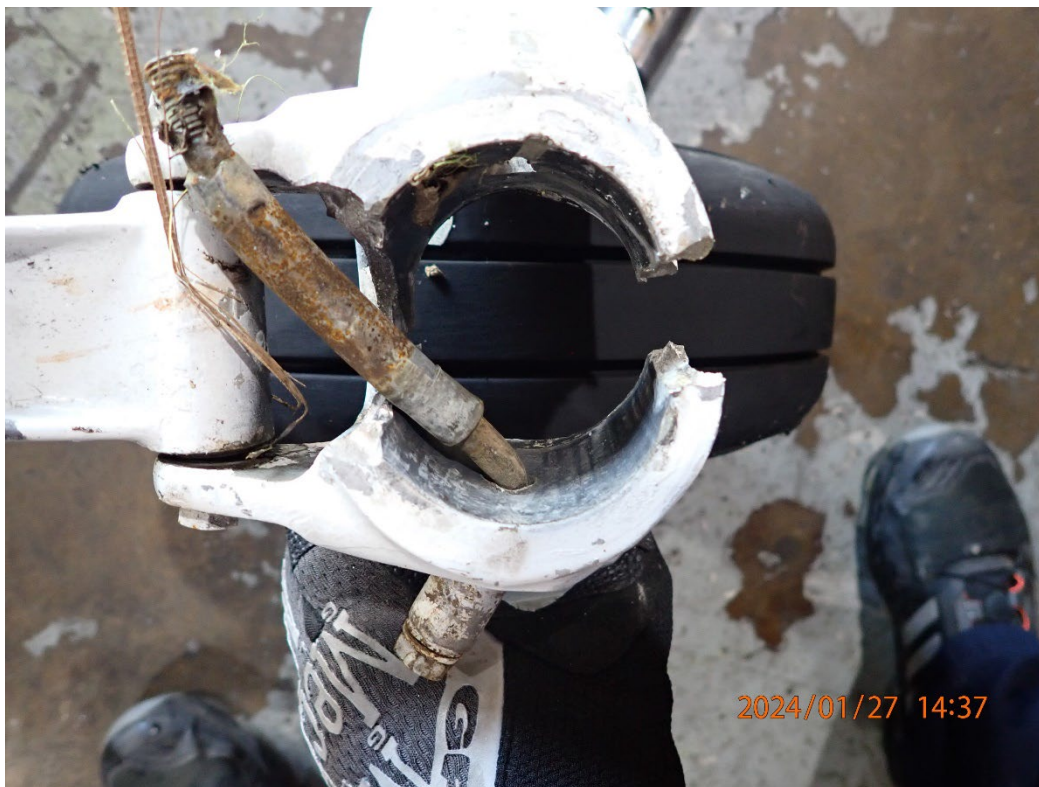
Photo 22: View of the nose wheel fork.
