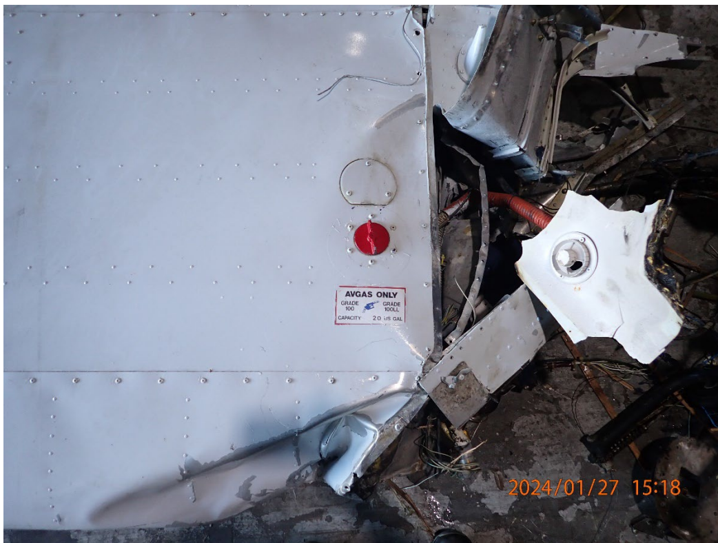
Photo 25: View of the right wing fuel cap.
