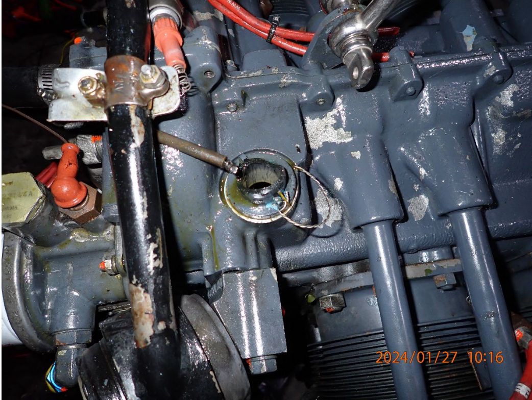
Photo 47: Impact separated oil filler tube and dipstick.
