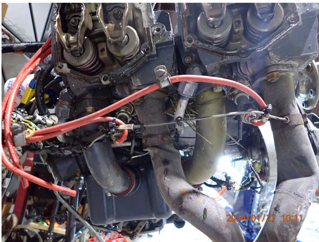
Photo 35: View of damage to the Nos. 1 & 3 exhaust.
