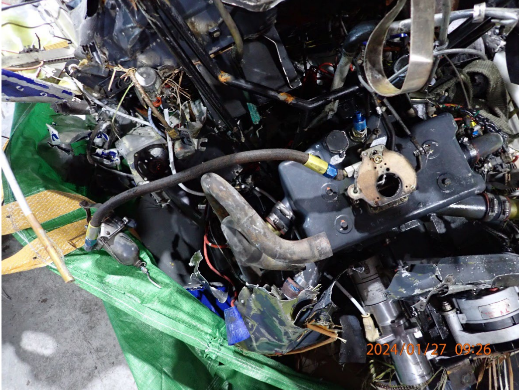
Photo 40: Fuel strainer and carburetor as first viewed at the recovery facility.
