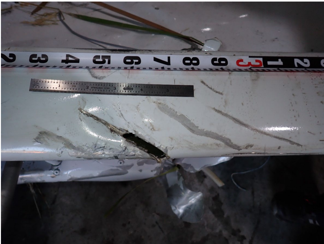
Photo 15: View of the cut and witness marks on the left wing strut. (Textron Aviation Photo)
