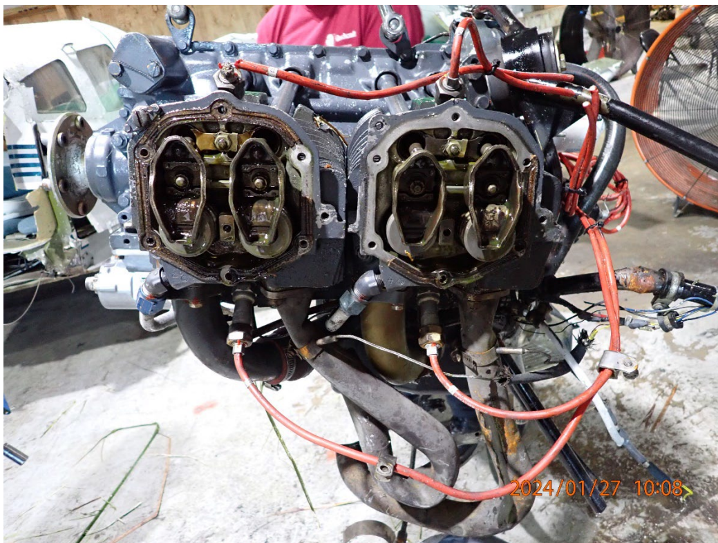
Photo 34: View of damage to the Nos. 2 & 4 exhaust.
