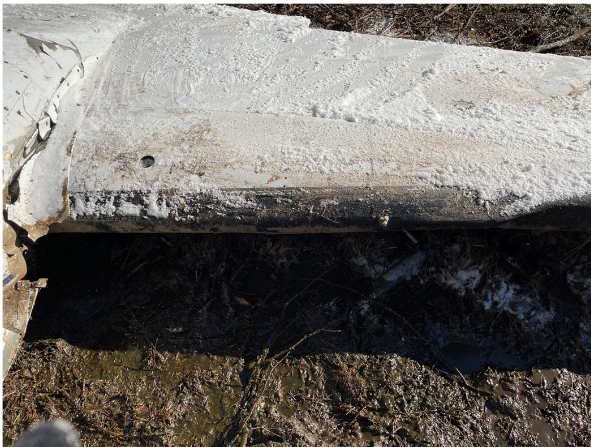
Photograph 4 - Ice on Leading Edge of Left Wing (outboard)
