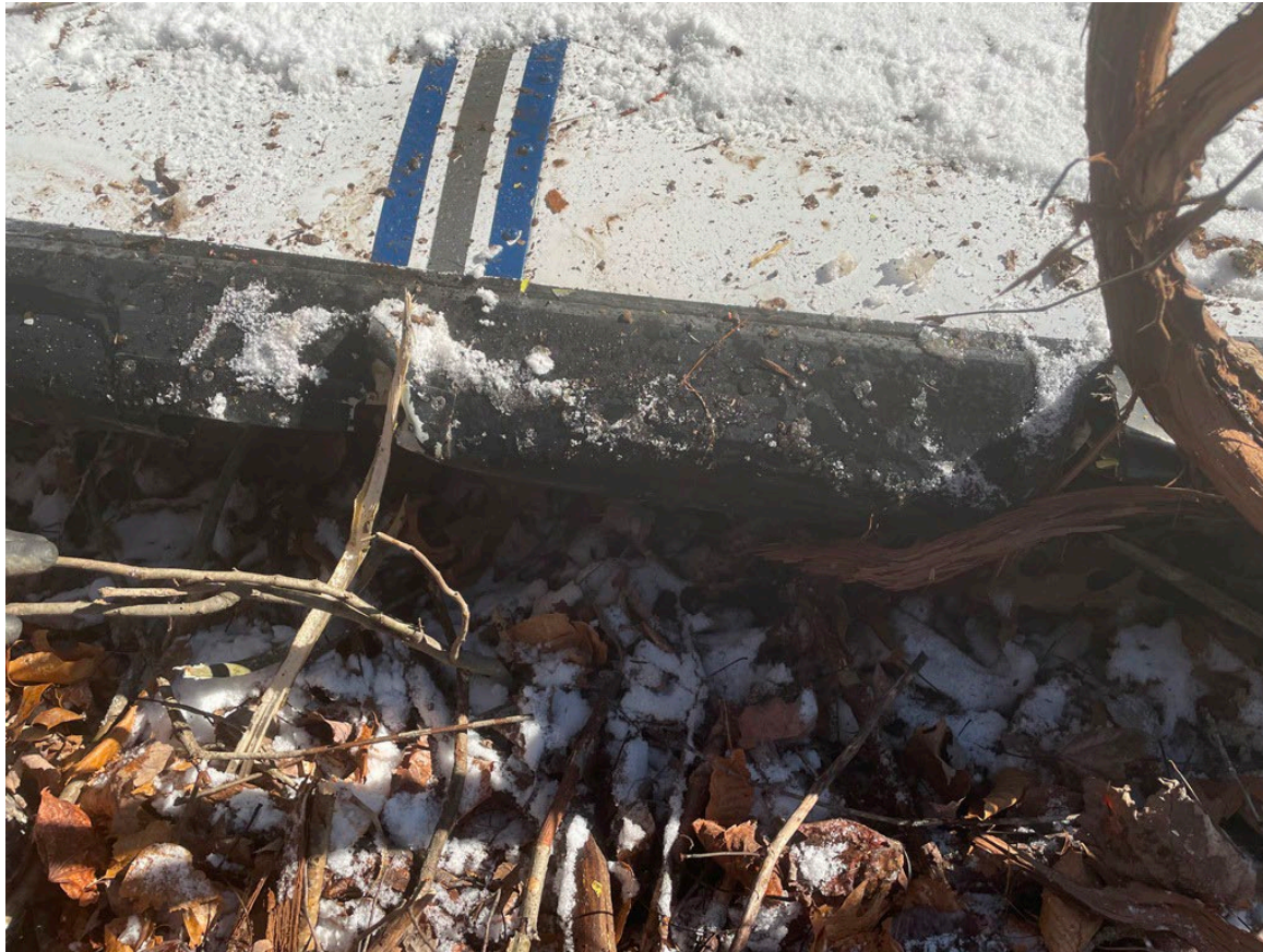
Photograph 5 - Ice on Leading Edge of Right Wing (outboard)
