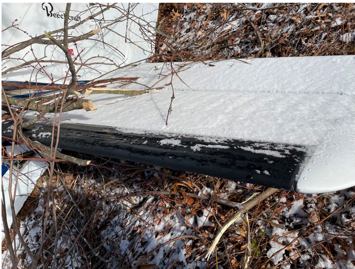
Photograph 6 - Ice on Leading Edge of Left Horizontal Stabilizer
