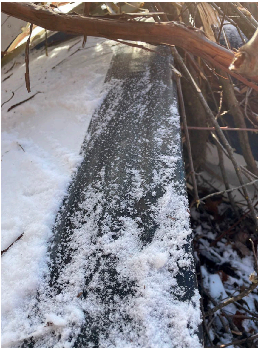
Photograph 7 - Ice on Leading Edge of Right Horizontal Stabilizer
