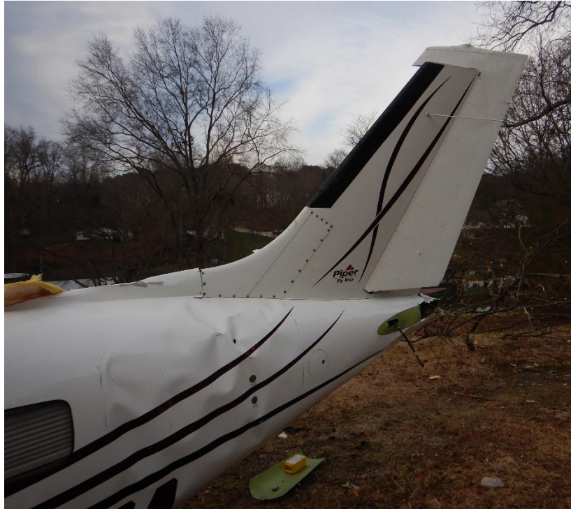
Photo 12 - Empennage with fractured left horizontal stabilizer.
