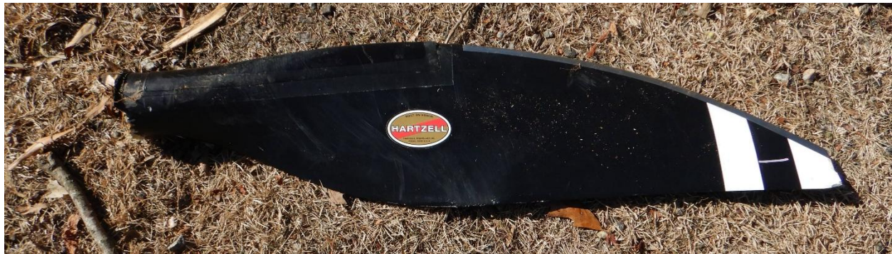
Photo 39 - Propeller blade separated from the propeller hub and intact.
