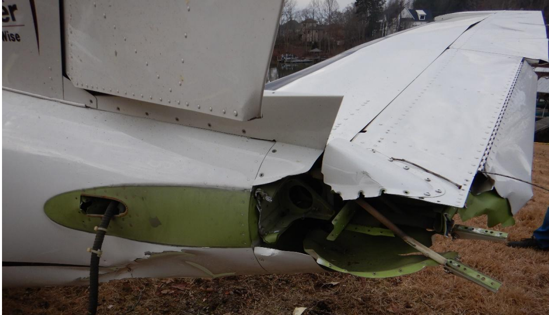
Photo 14 - View of right horizontal stabilizer from fracture area.
