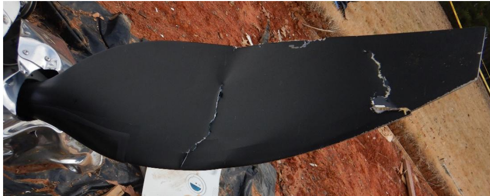
Photo 37 - One propeller blade remained attached to the propeller hub.
