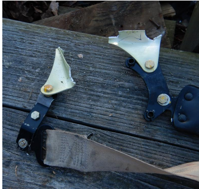
Photo 23 - Fractured pilot seatbelt anchors.
