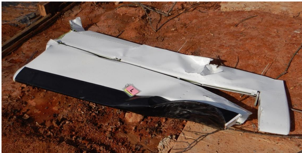
Photo 13 - Left horizontal stabilizer with elevator after elevator recovery from tree.
