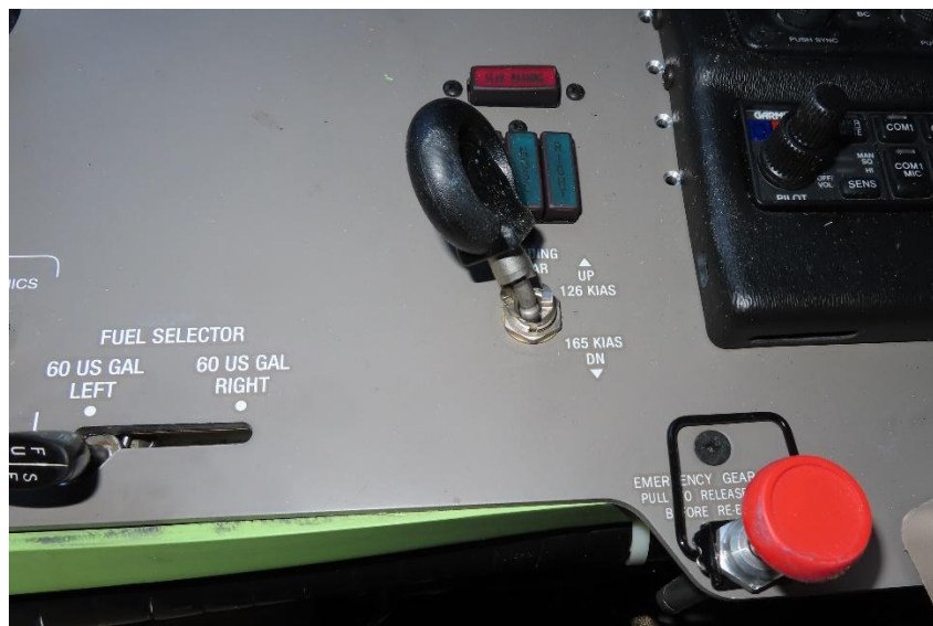
Photo 22 - Close-up view of landing gear selector in UP position.
