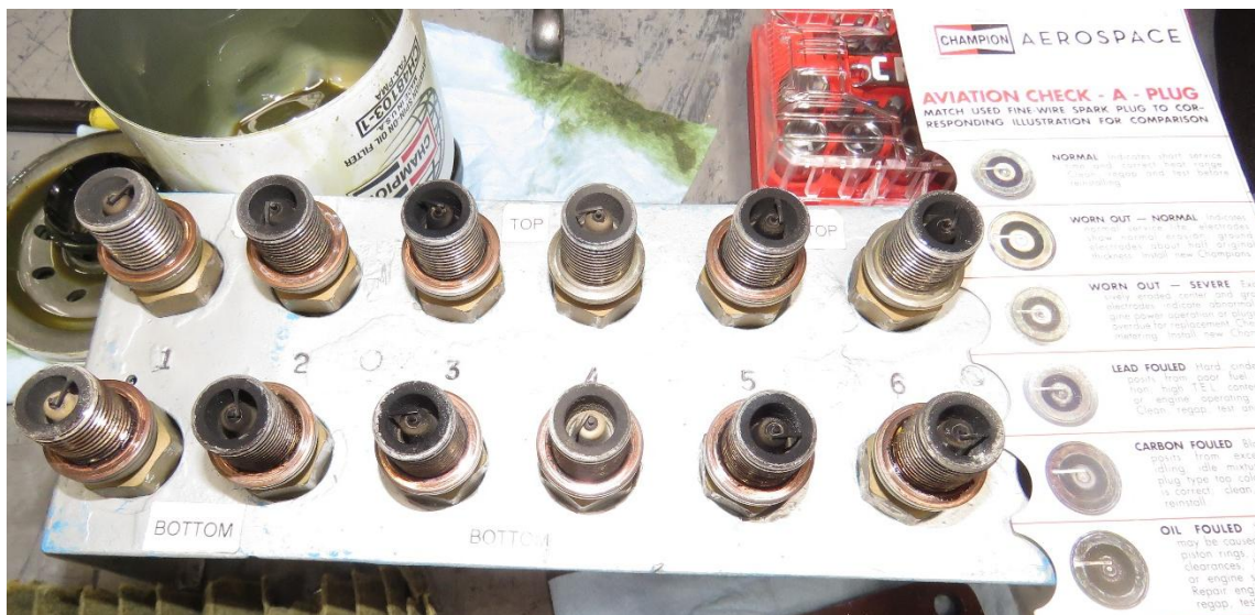
Photo 32 - The spark plugs were carbon fouled.
