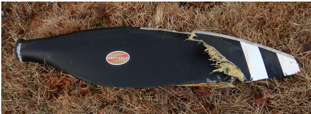
Photo 38 - Propeller blade separated from the propeller hub and fractured.
