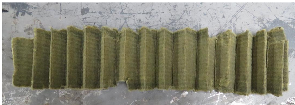
Photo 33 - Oil filter element free from debris.
