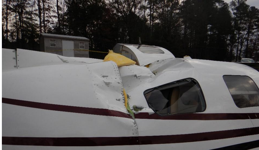
Photo 11 - Close-up of upper fuselage damage.
