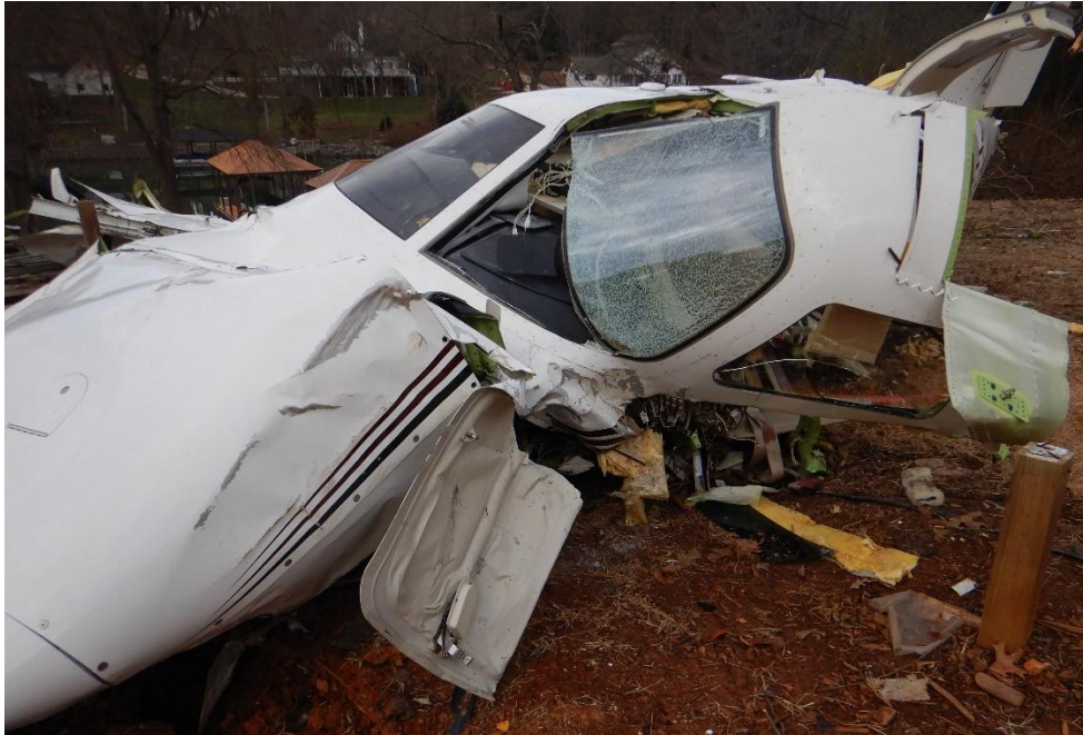
Photo 10 - Close-up view of crushing to lower front left cockpit area.
