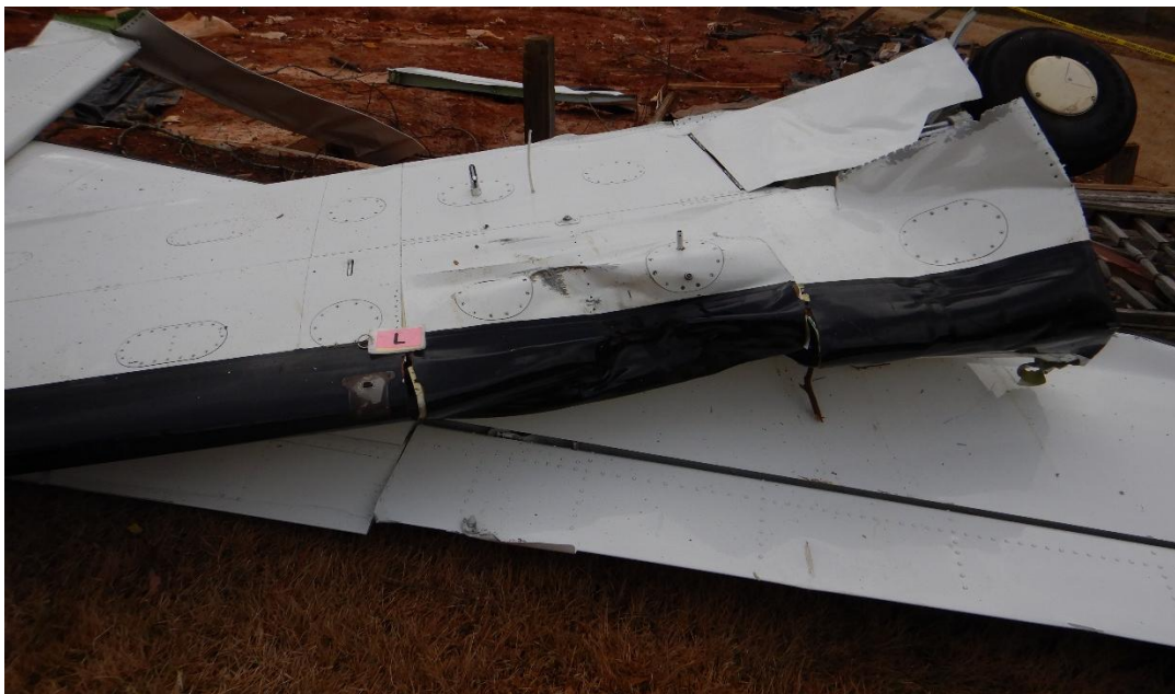
Photo 15 - Inverted left wing as found on right wing.
