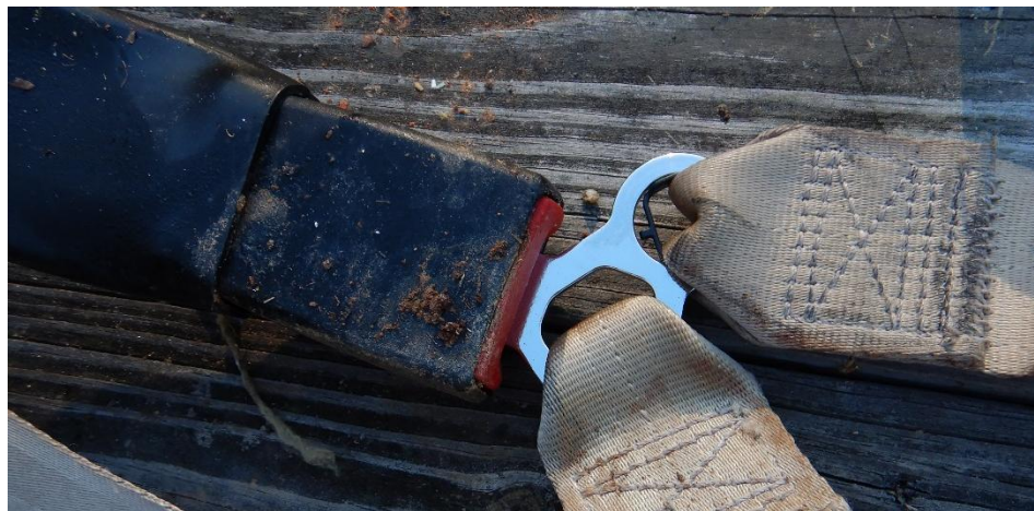
Photo 24 - Pilot seatbelt still fastened to buckle.
