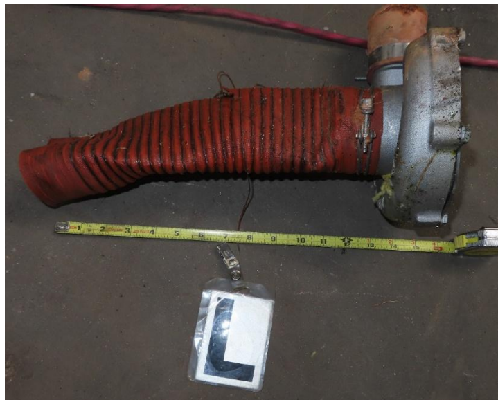
Photo 35 - Left side scat tubing from induction airbox to the left turbocharger compressor section.
