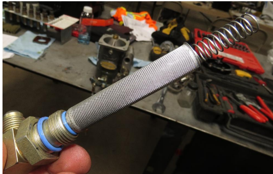
Photo 29 - The fuel servo screen was unobstructed.
