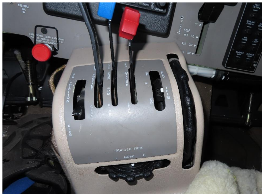
Photo 20 - Throttle quadrant and flap selector set to zero.
