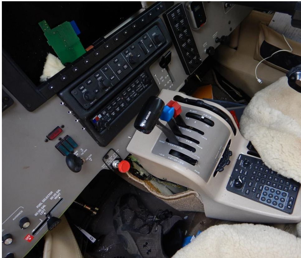
Photo 19 - Throttle control quadrant with all levers full forward.
