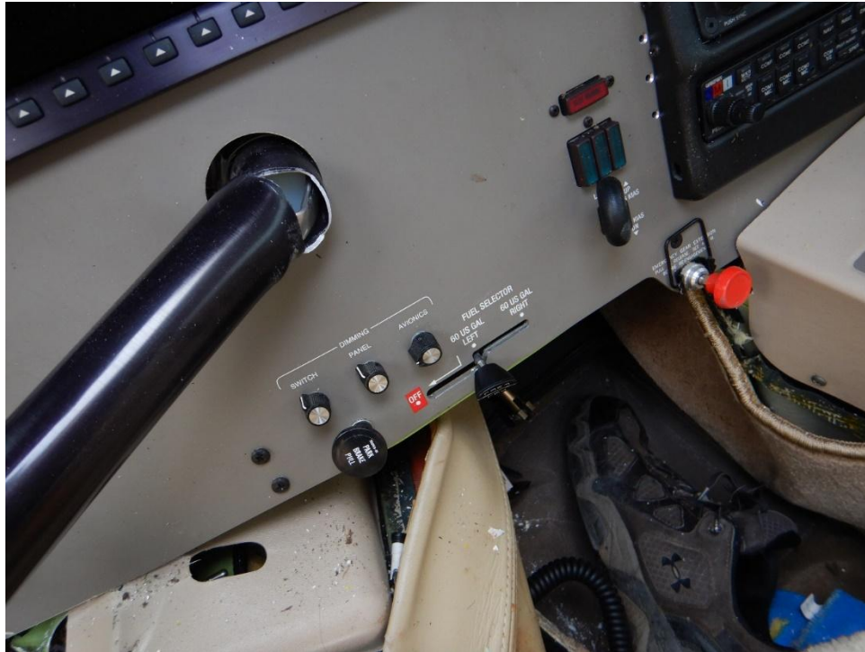
Photo 21 - Fractured pilot control column and fuel selector.
