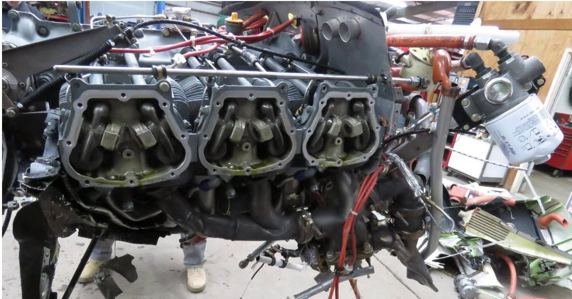
Photo 28 - Cylinder Nos. 2, 4 and 6 with rocker covers removed.
