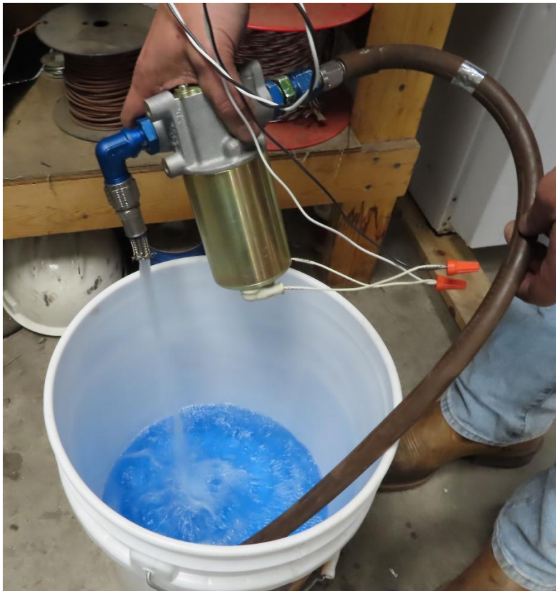
Photo 25 - Emergency fuel pump tested using 100LL fuel and 24 volt power source.
