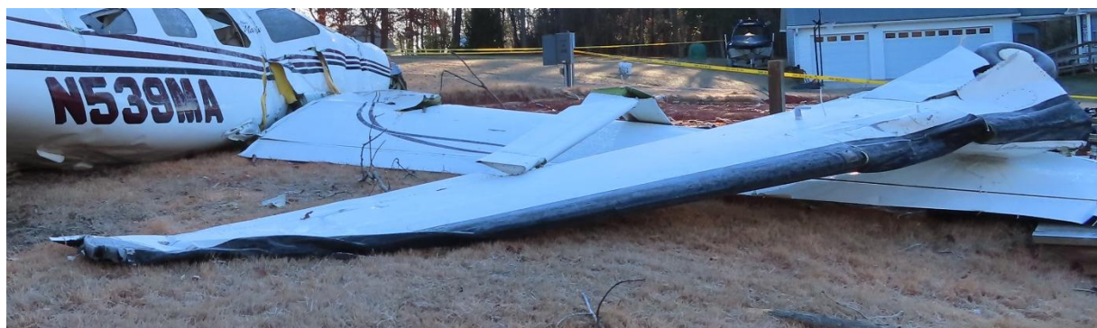
Photo 16 - View of inverted left wing once partially removed from right wing.
