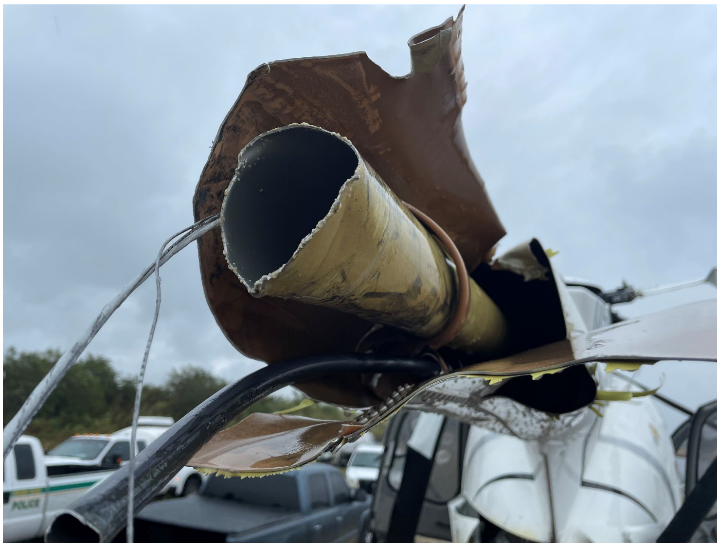
Photograph 2 - Tail boom cut off
