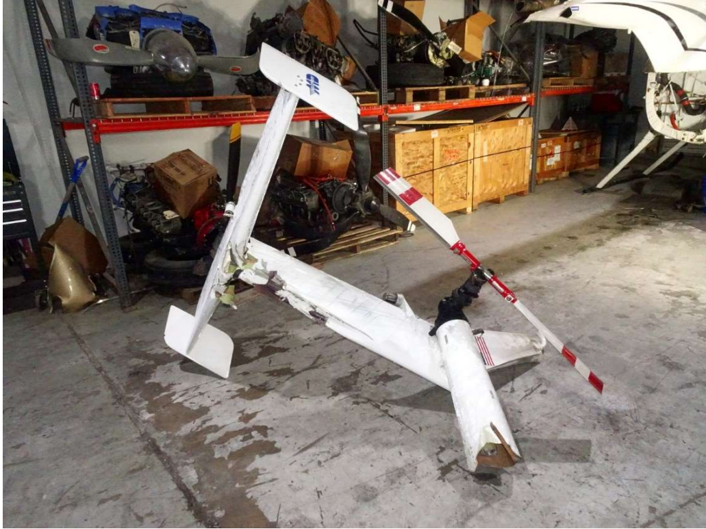
Figure 2. The recovered empennage wreckage.
