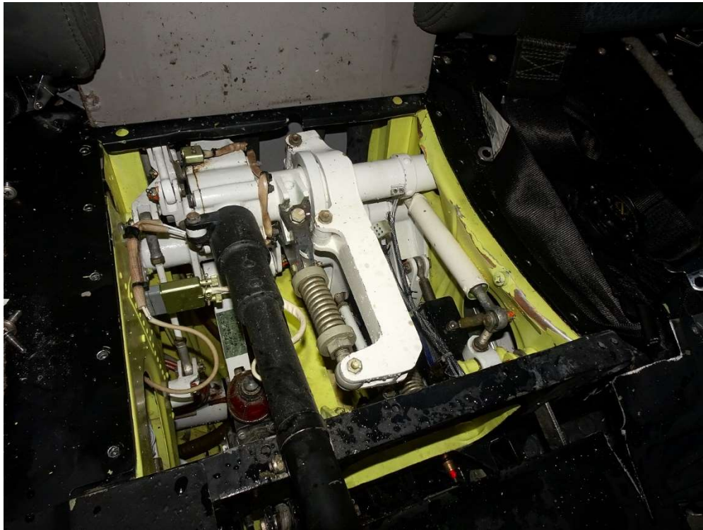
Figure 7. A portion of the cockpit flight control bellcranks and balance springs.
