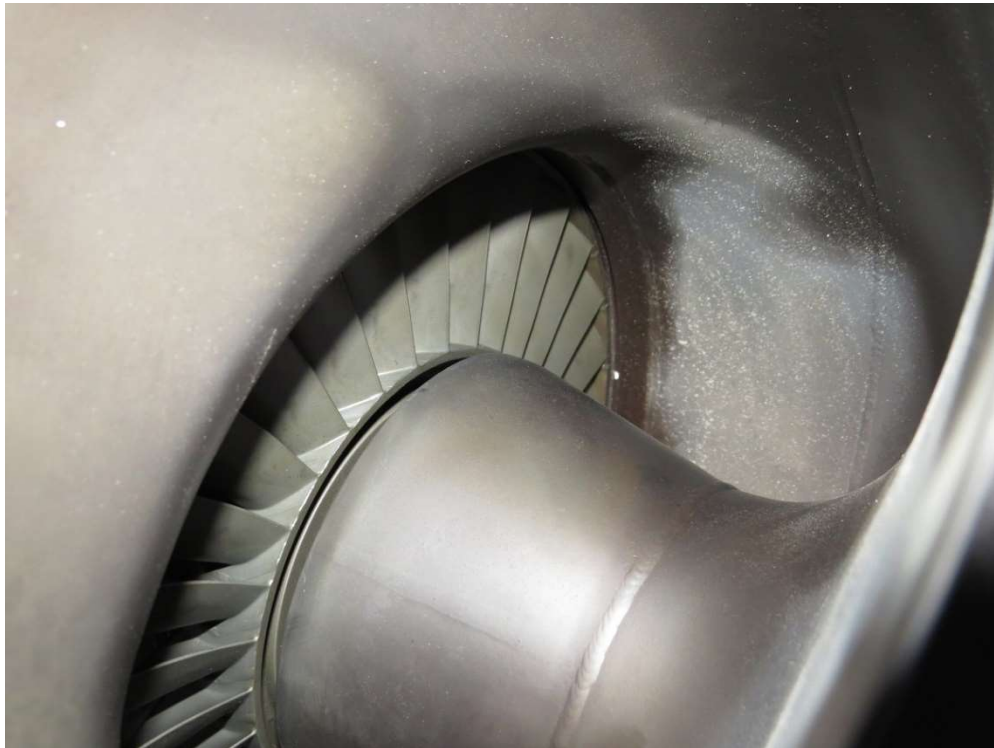
Figure 11. The fourth stage power turbine. (Image courtesy of Rolls-Royce)
