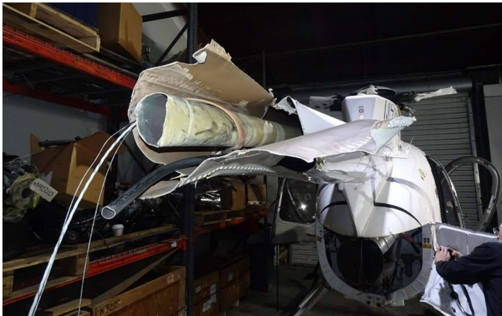
Figure 3. The fractured tail boom, tail rotor drive shaft, and tail rotor control tube.
