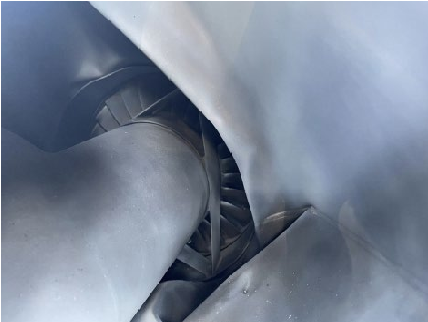
Photograph 12 - Power Turbine (Courtesy of Safran)
