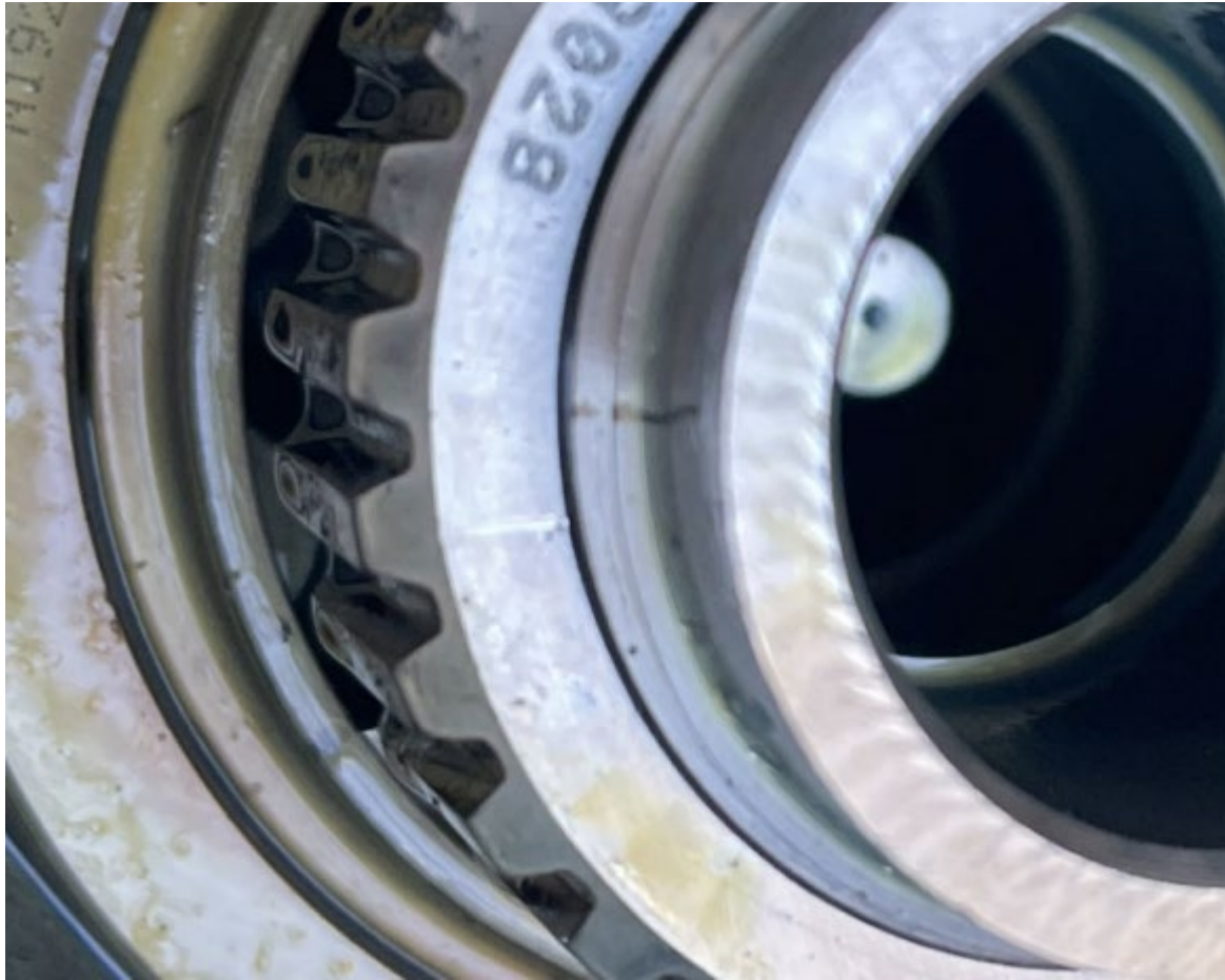
Photograph 13 - Input Pinion Slippage Mark Misalignment (Courtesy of Safran)
