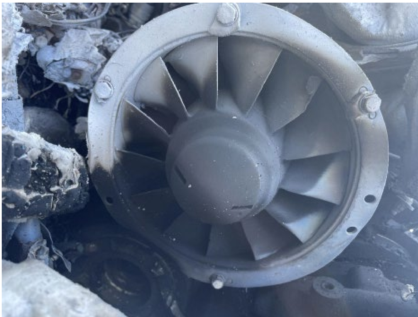
Photograph 11 - Axial Compressor (Courtesy of Safran)
