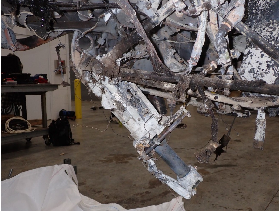
Photograph 10 - NTSB Digital Photograph. View Focused on the Remaining Portion of the Nose Landing Gear
