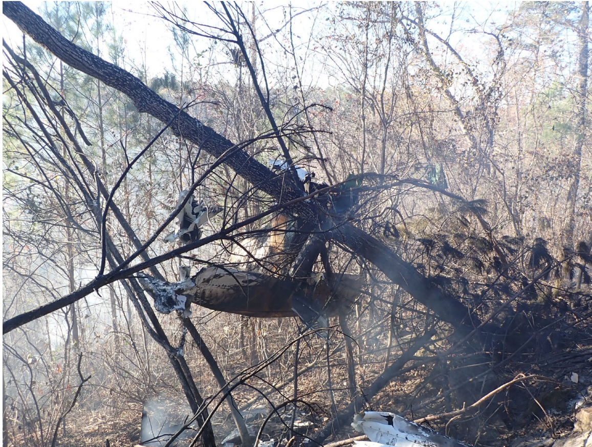
Photograph 3 - NTSB Digital Photograph. View of the Aft Empennage Suspended in Tree
