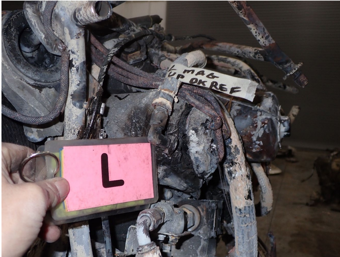
Photograph 13 - NTSB Digital Photograph. Close-Up View of Heat Damaged Left Magneto
