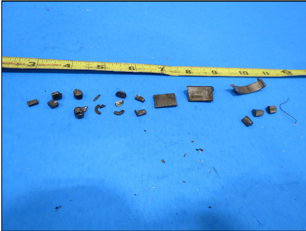
Figure 16 Ferrous Debris Retained From Oil Sump
