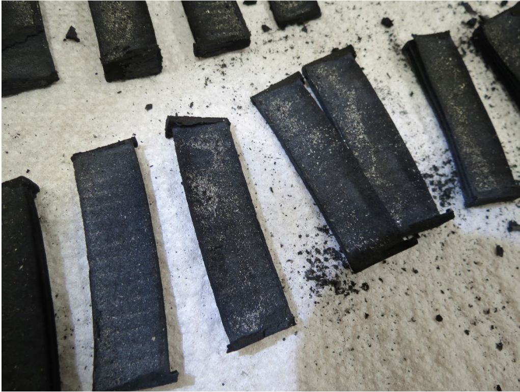
Figure 17 View of Debris on Oil Filter Element
