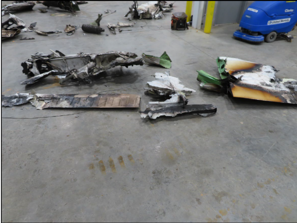
Figure 12 Remaining Sections of Right Wing, Landing gear, and Sections of Flap and Aileron
