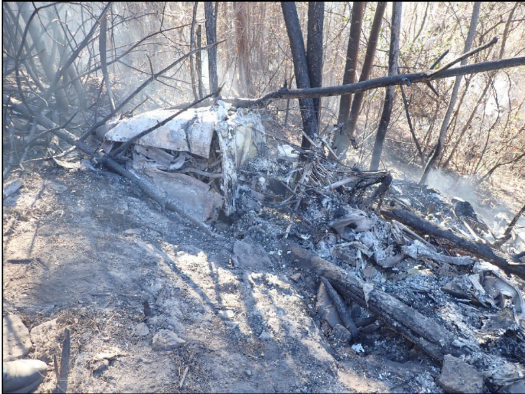
Figure 10 Left Side View of the Remains of the Cockpit, Cabin, and Engine Assembly with Attached Propeller.
