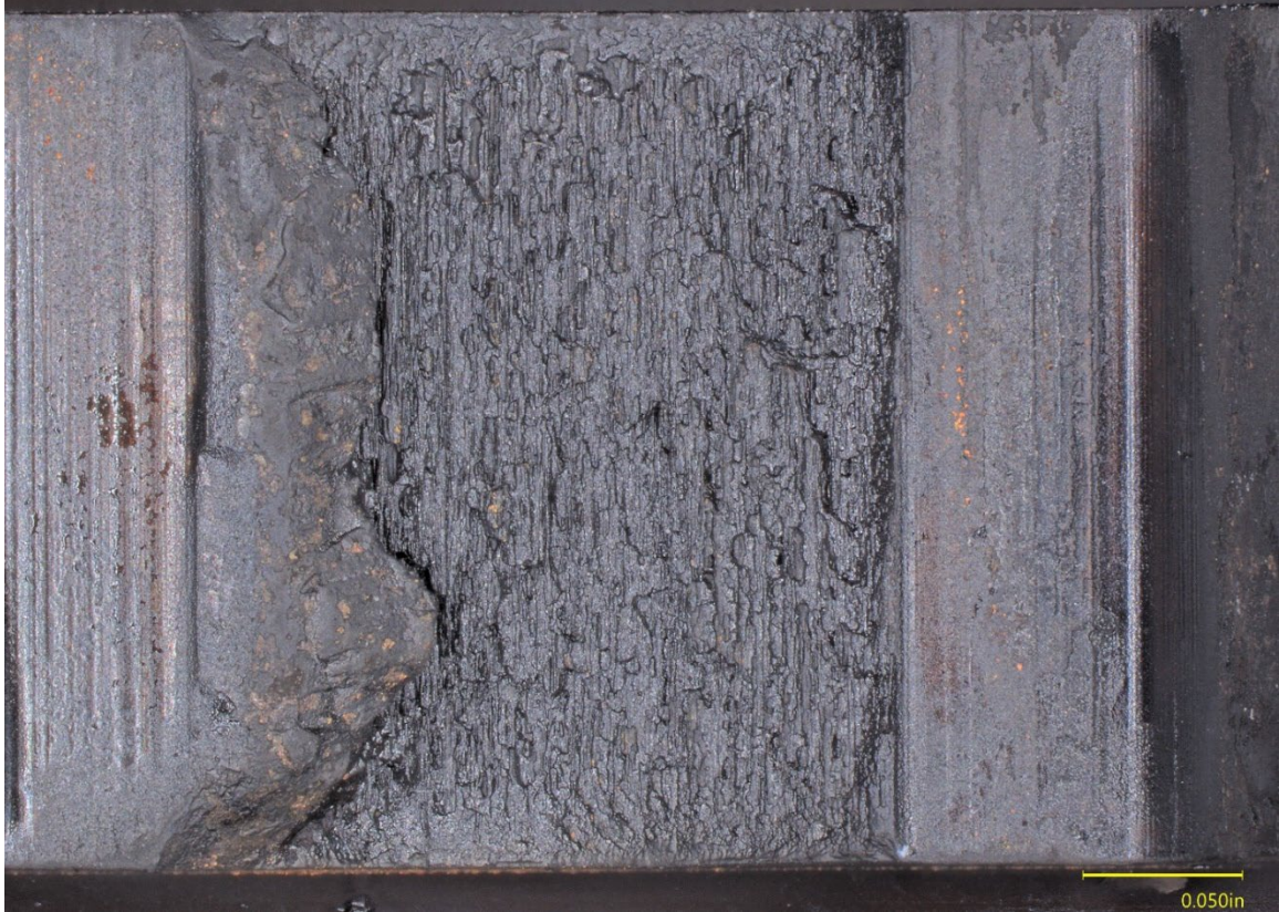
Figure 16. View of the right side crankshaft idler gear tooth fracture in Figure 7 .
