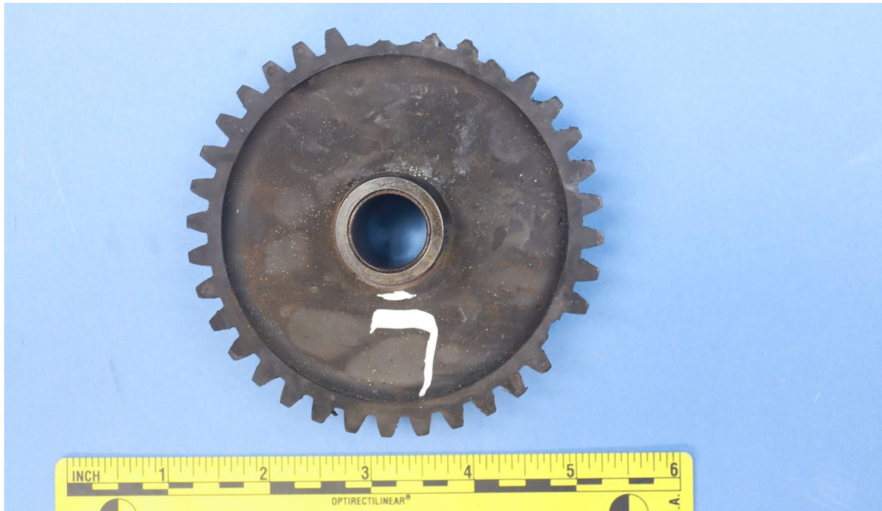
Figure 2. The marked face of the left crankshaft idler gear, as received.
