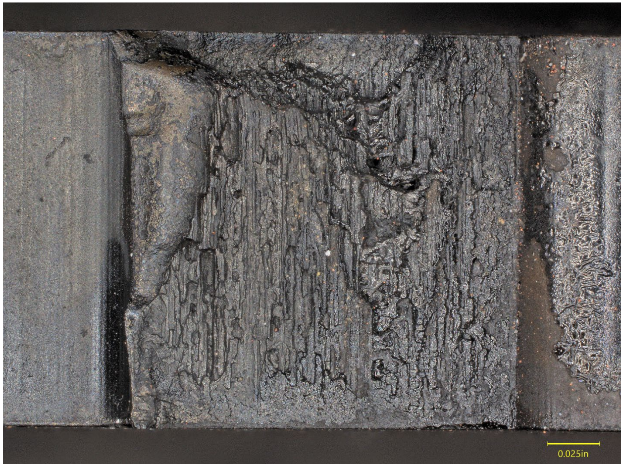
Figure 26. View of the left tooth fracture on the fuel pump idler gear from Figure 25 .
