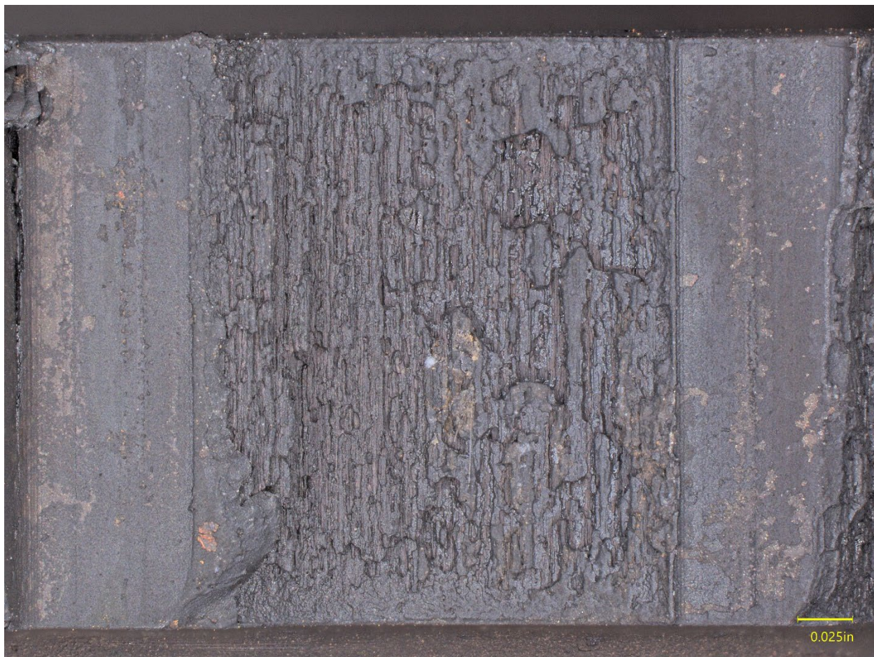
Figure 8. View of the left tooth fracture surface on the idler gear from Figure 7.
