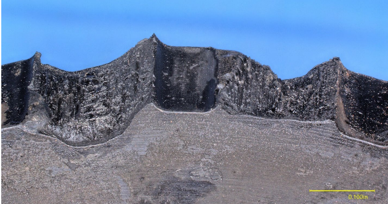
Figure 24. Angled view of the fuel pump idler gear fracture surfaces.
