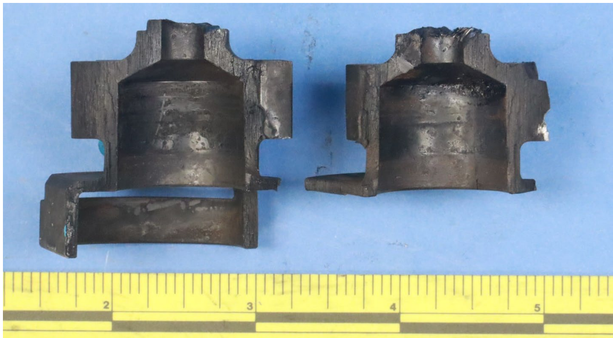
Figure 36. The opposite-facing fracture surfaces of the left magneto gear, as received.
