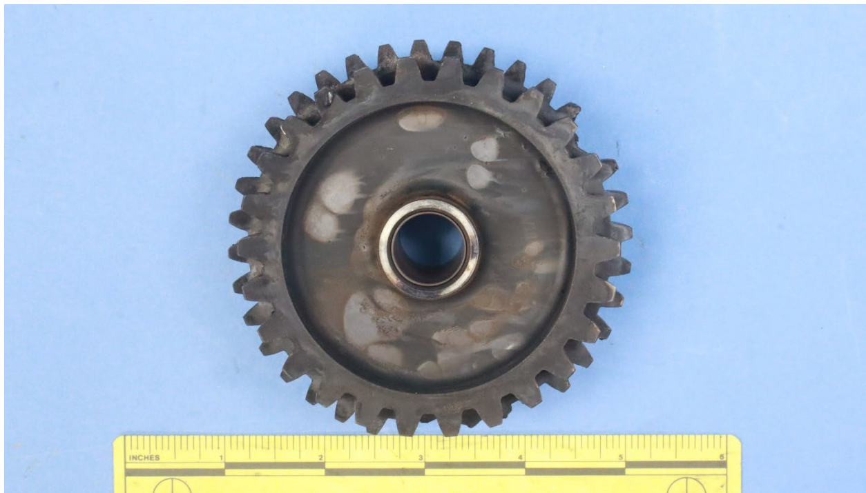
Figure 3. The left crankshaft idler gear viewed opposite from Figure 2 .
