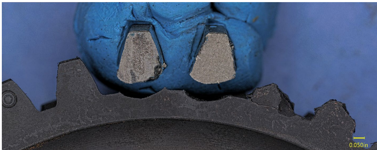
Figure 6. View of the two fractured teeth from the idler gear, positioned near their respective fracture locations.
