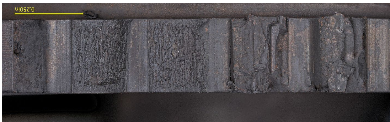
Figure 7. View of the fractured teeth surfaces in Figure 6 , showing the adjacent damaged teeth remnants.
