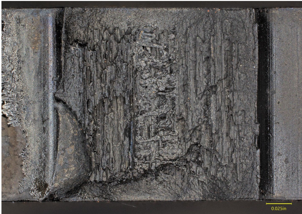
Figure 33. The right tooth fracture surface from the fuel pump idler gear in Figure 25 .
