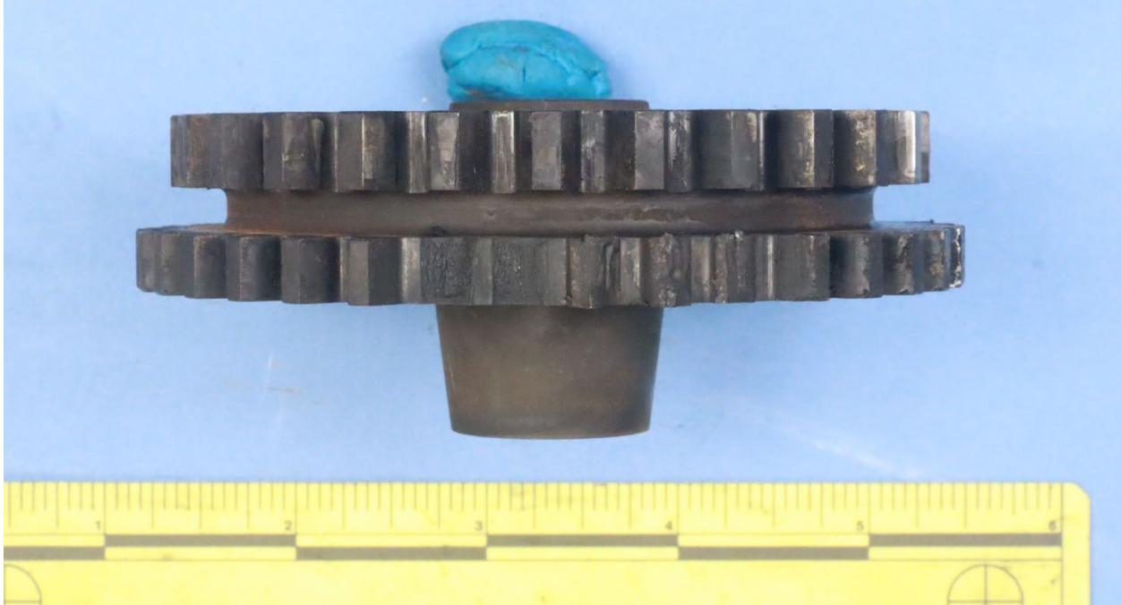
Figure 4. View of the two fractured teeth at the 12 o'clock position on the crankshaft idler gear as clocked in figure 2.
