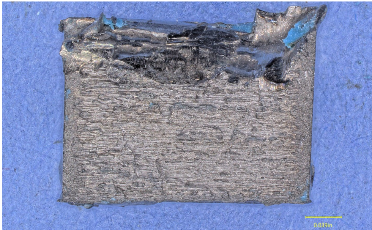
Figure 9. View of the left tooth fracture surface from the liberated tooth.
