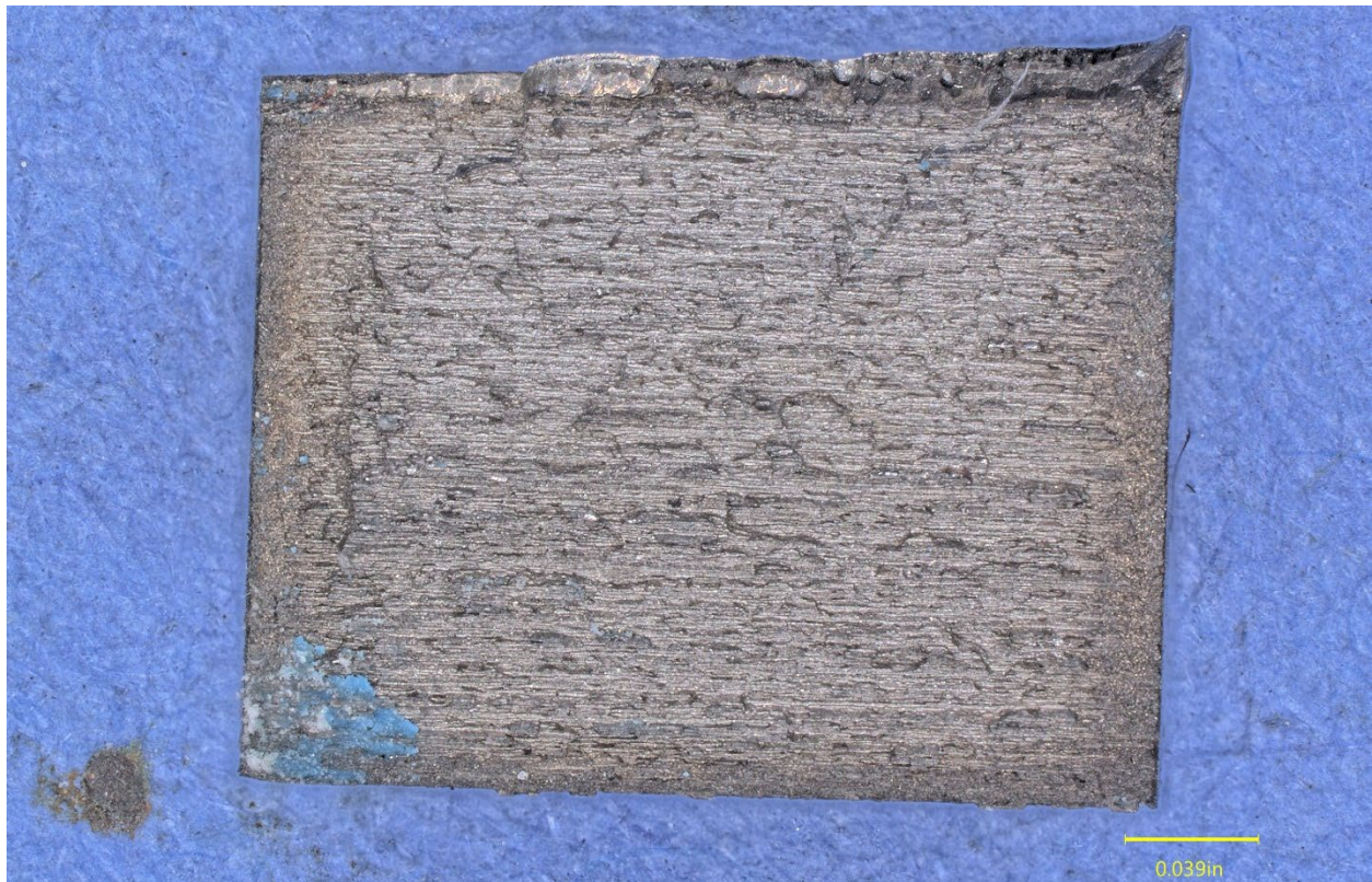
Figure 20. The fractured tooth fracture surface opposite the gear surface in Figure 19 .
