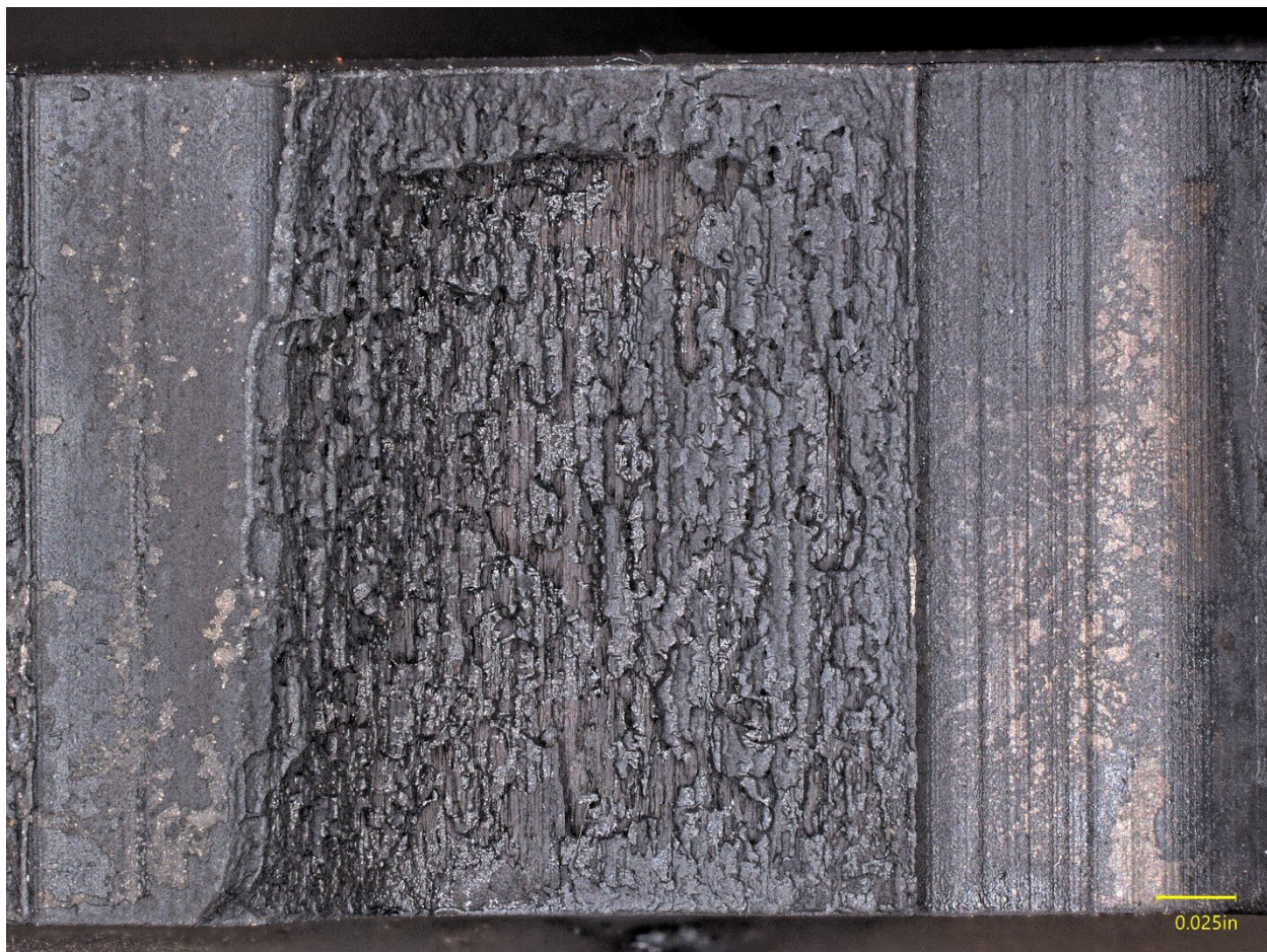
Figure 19. The single tooth fracture surface on the crankshaft idler gear.
