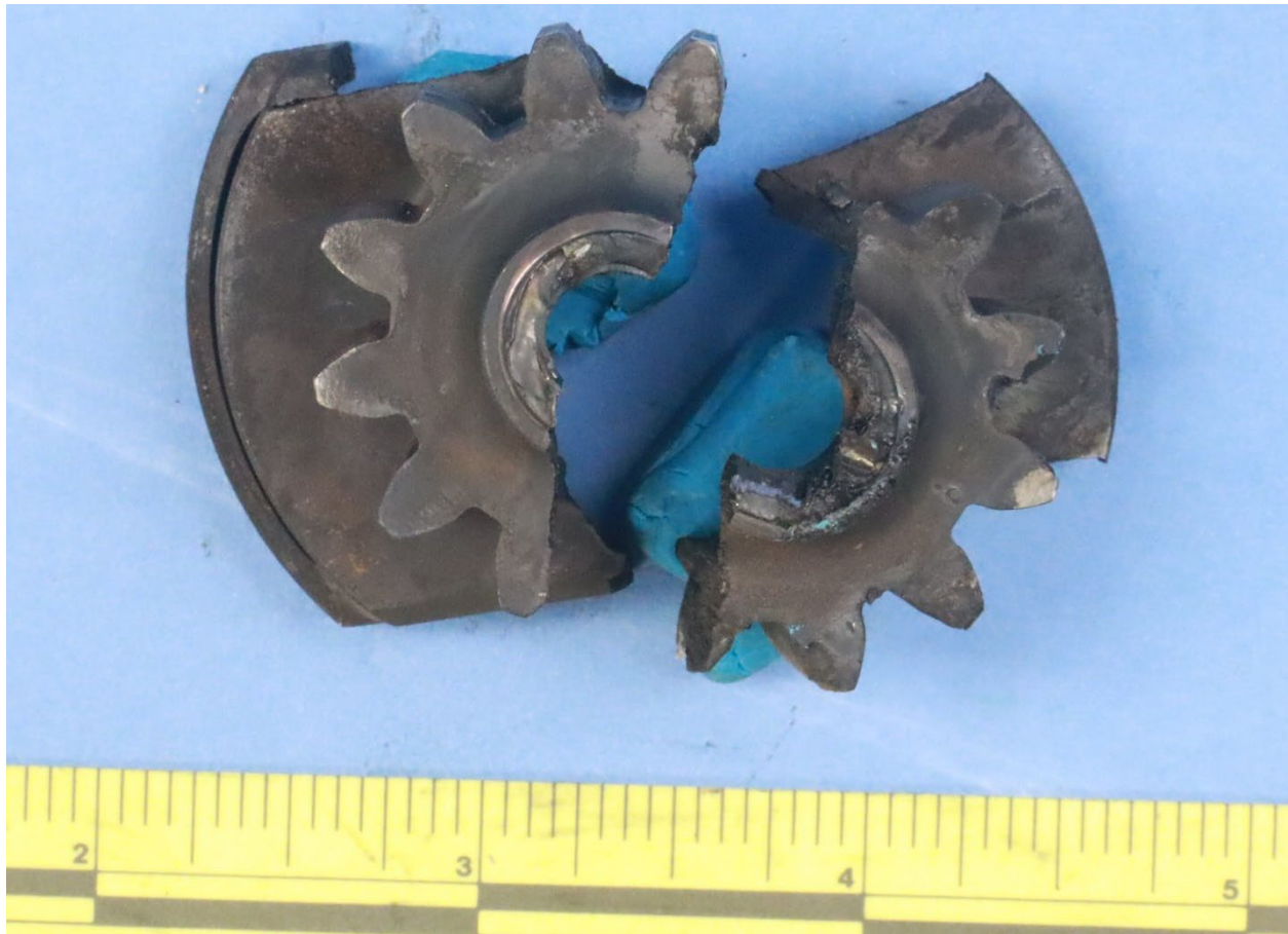
Figure 35. The fragments of the fractured left magneto gear, as received.
