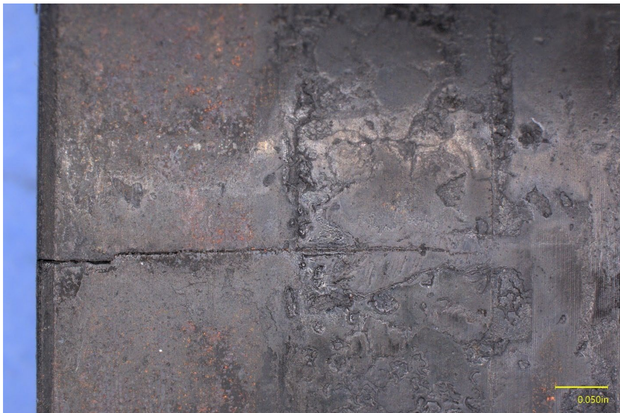
Figure 37. View of a crack on the boss of the larger magneto gear remnant.
