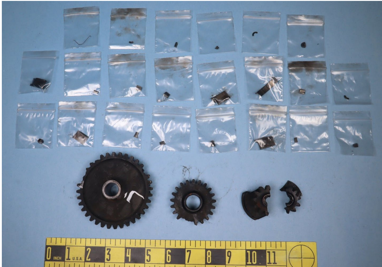
Figure 1. The pieces submitted from the accident, including the fuel pump idler gear, left crankshaft idler gear, left magneto gear, and multiple loose gear teeth and debris in individual bags.
