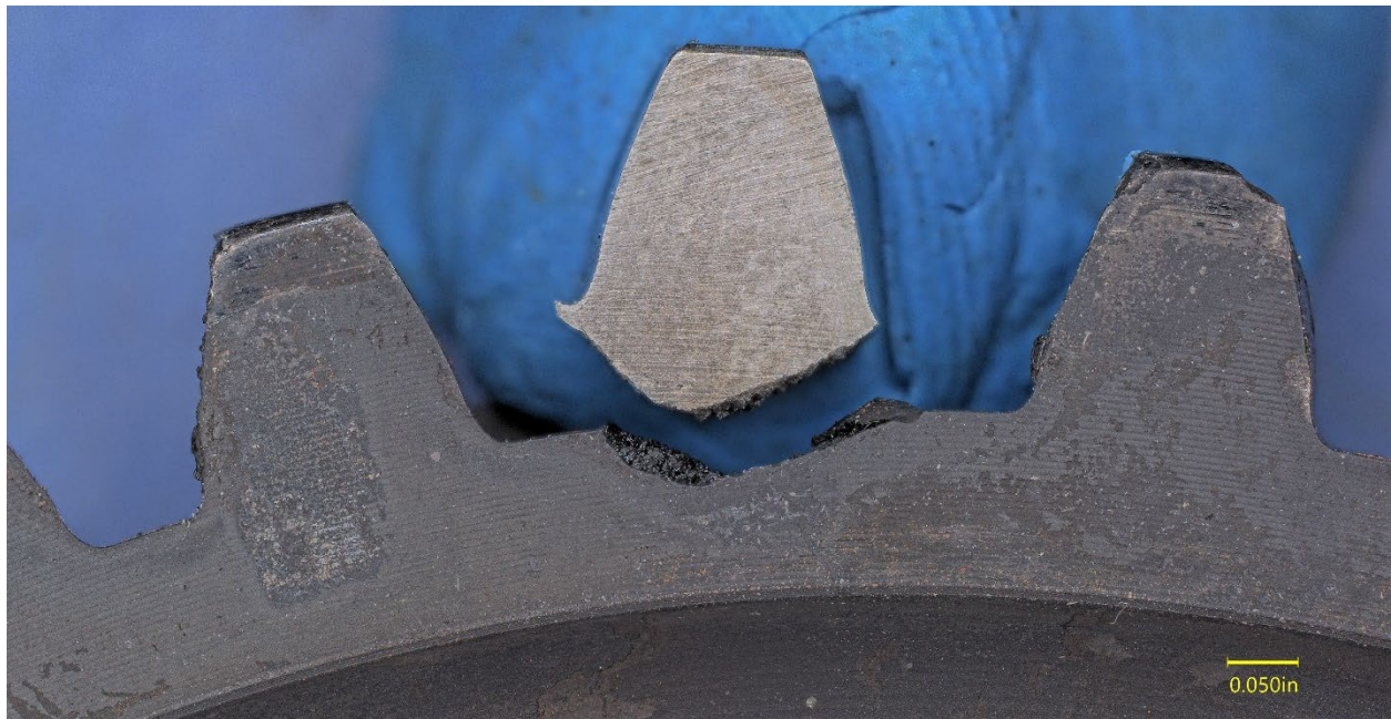
Figure 18. The opposite single tooth fracture of the crankshaft idler gear.
