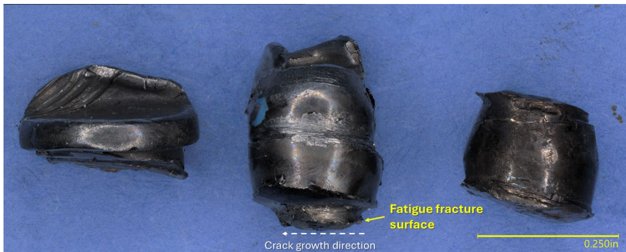
Figure 48. Side view of the three fractured rivet remnants. The arrow denotes the location of the fatigue cracking.
