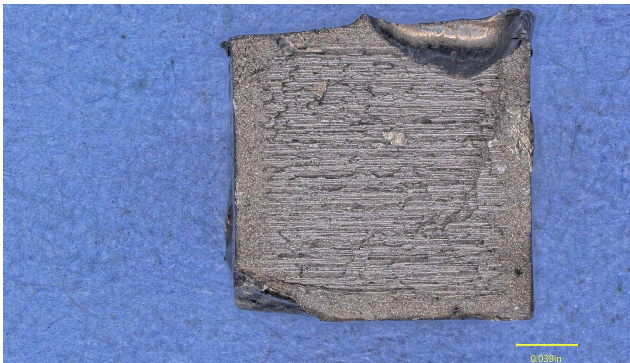
Figure 34. Right liberated tooth fracture surface that mates with the surface in Figure 33 .
