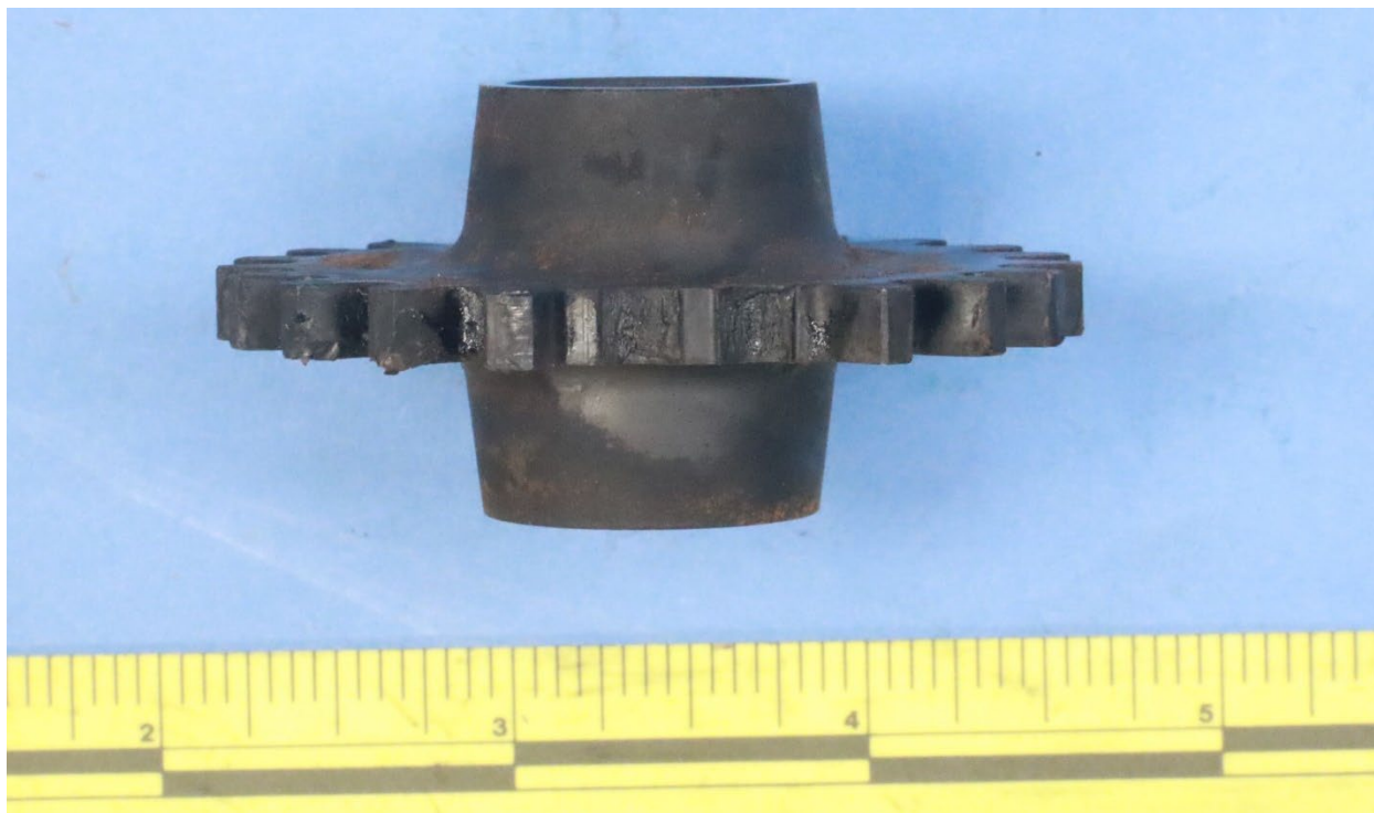
Figure 22. The fractured teeth locations of the fuel pump idler gear, as received.
