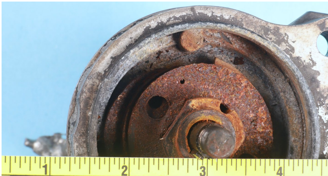
Figure 8. Closer view of the stop pin after impulse shell removal (and after rivets shown in Figure 9 had fallen out).
