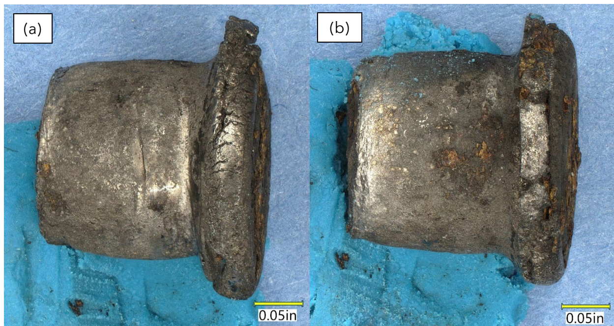
Figure 14. Side views of the downward-facing rivet, after removal of most of the surface rust.
