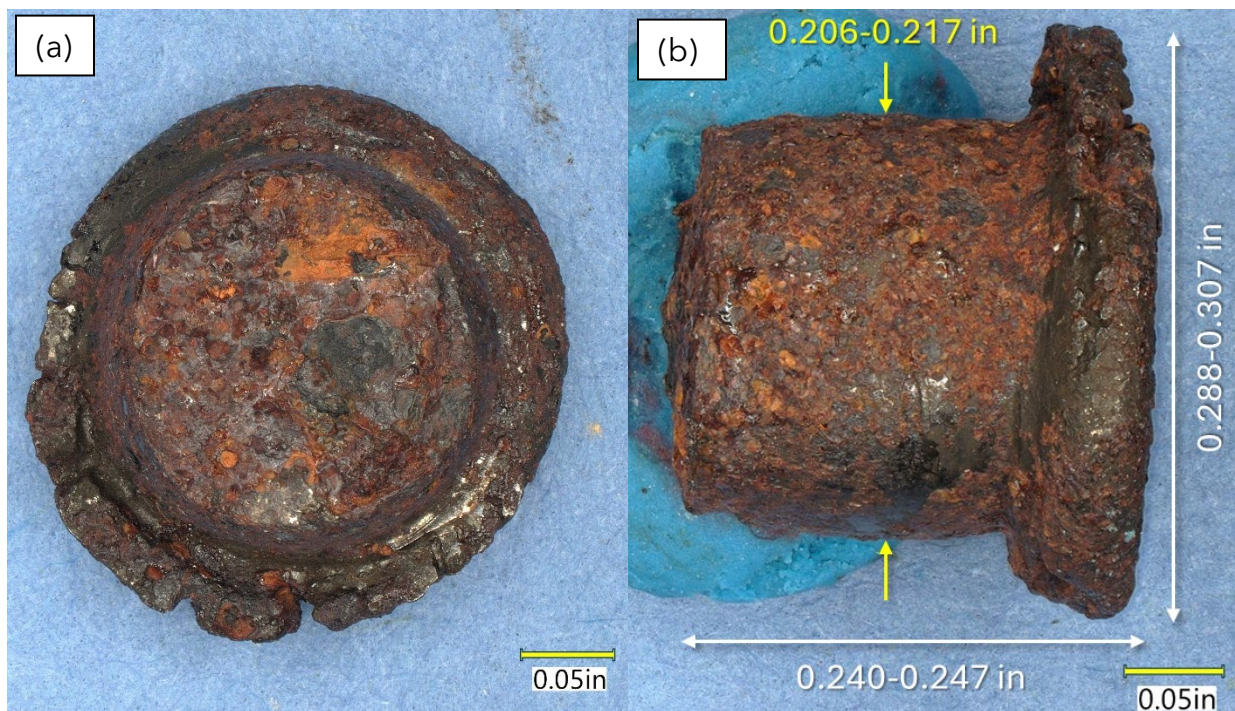
Figure 12. The upward-facing rivet (located on the top of Figure 9) from (a) the fracture surface and (b) the side, as disassembled.
