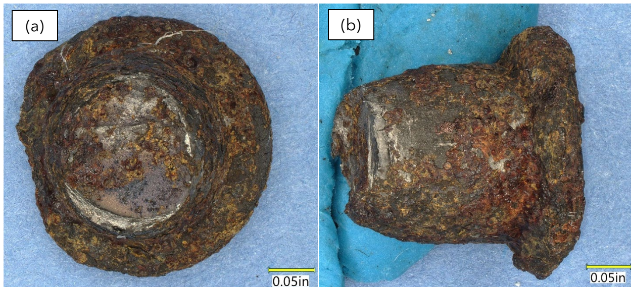
Figure 18. Fracture surface and side views of the upward-facing rivet, after removal of much of the surface contamination.
