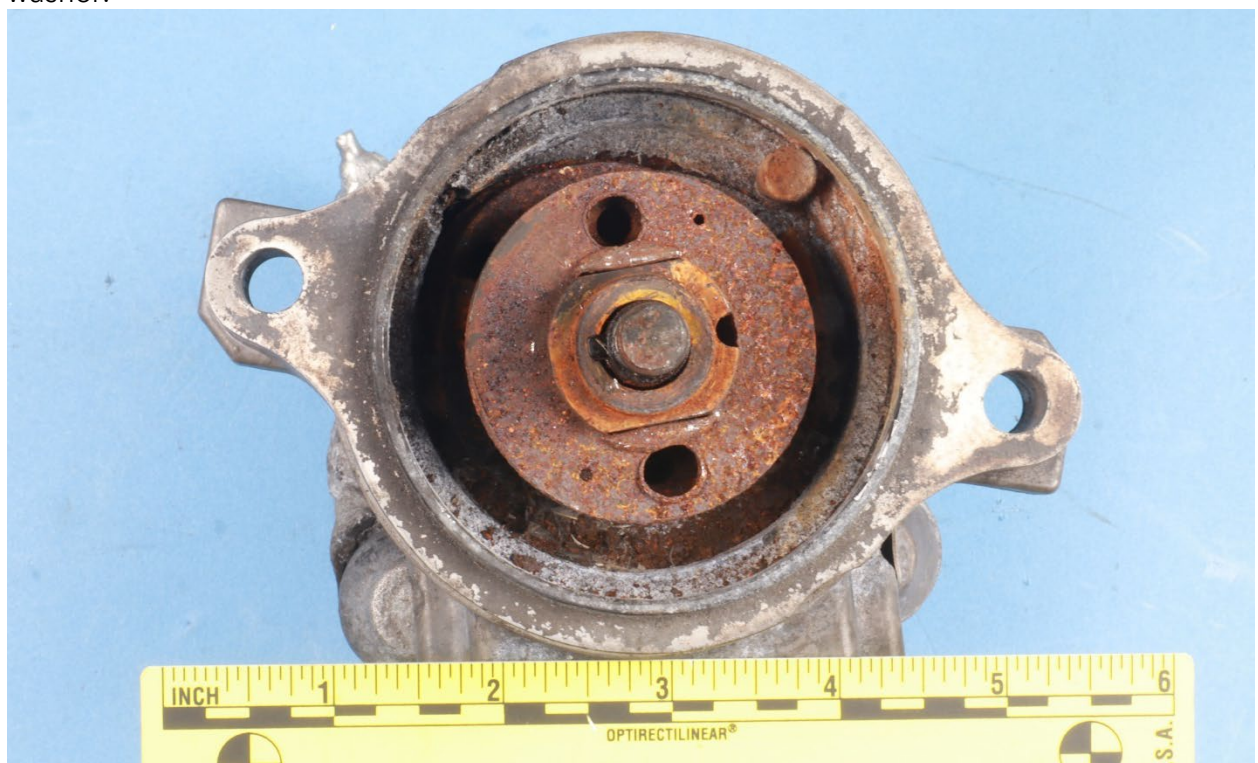
Figure 10. View of the impulse hub from Figure 9, after rivet removal, showing the widened rivet holes with deformation indications.
