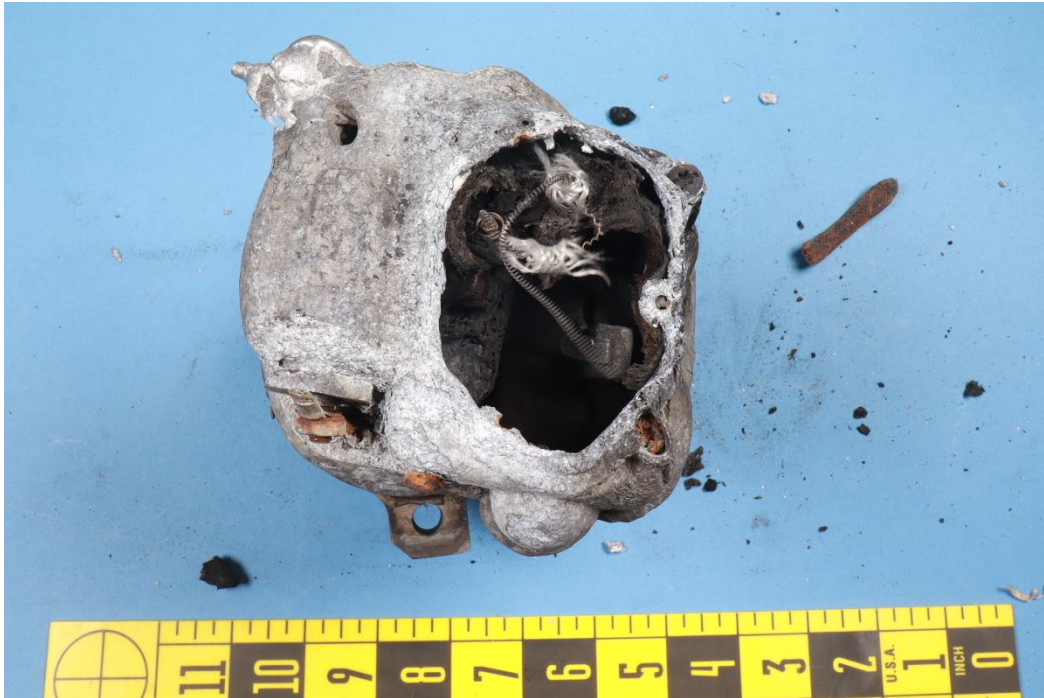
Figure 3. View of the missing area of the magneto housing, consistent with heat damage.
