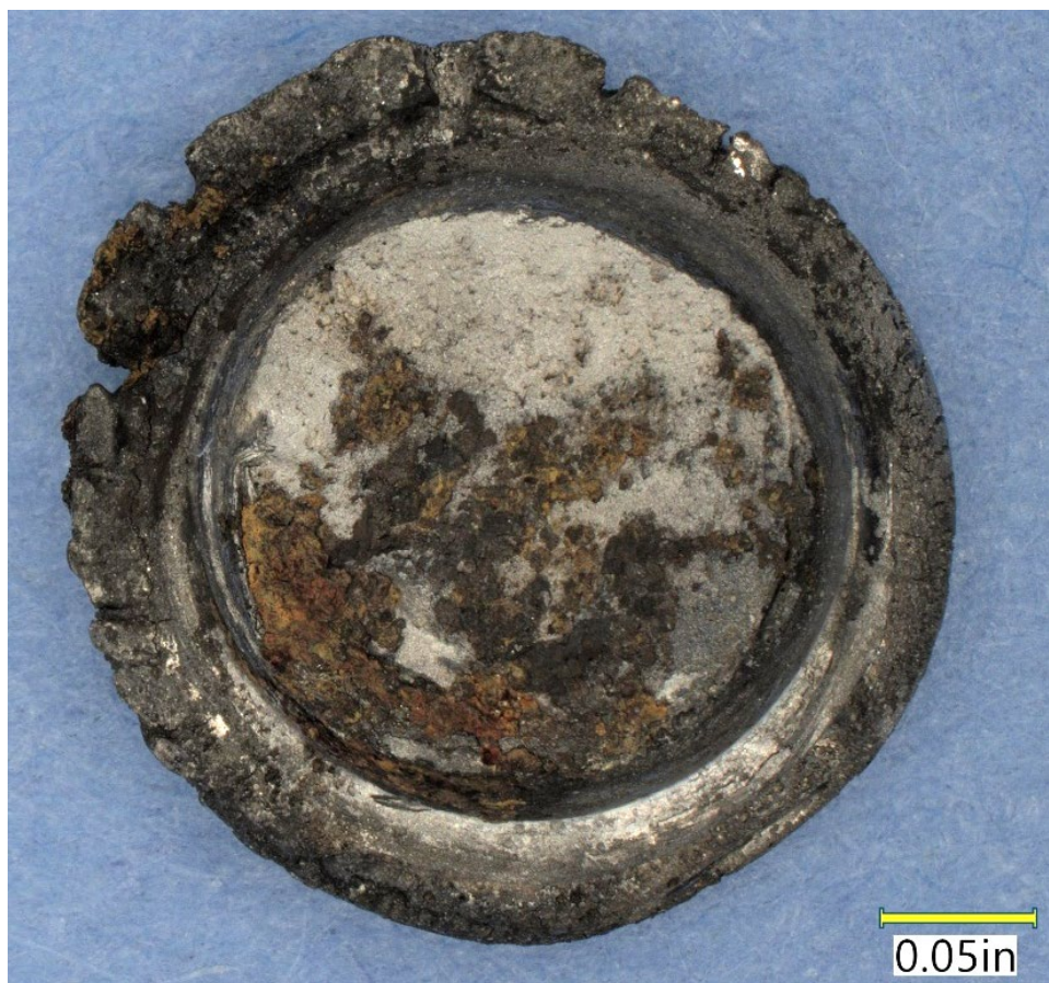
Figure 15. View of the fracture surface of the downward-facing rivet, after removal of most of the surface contamination.
