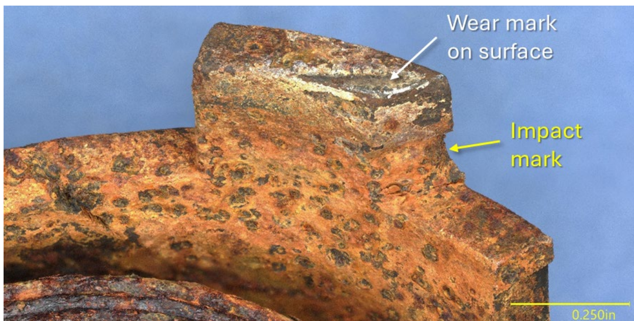
Figure 6. View of the wear mark on the stop boss protruding from the impulse shell skirt.
