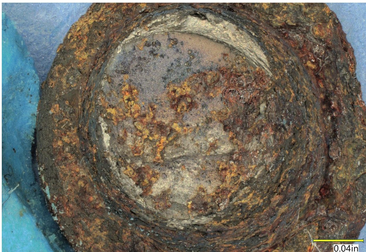
Figure 19. Closer view of the upward-facing rivet fracture surface, showing areas of wear and a flat, discolored portion of the fracture surface.
