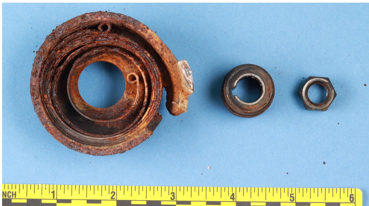
Figure 5. View of the underside of the impulse shell with coiled spring, the hub, and nut after disassembly.
