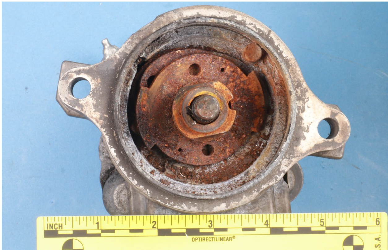
Figure 11. View of the underlying pawls under the key, after removal of the hub.
