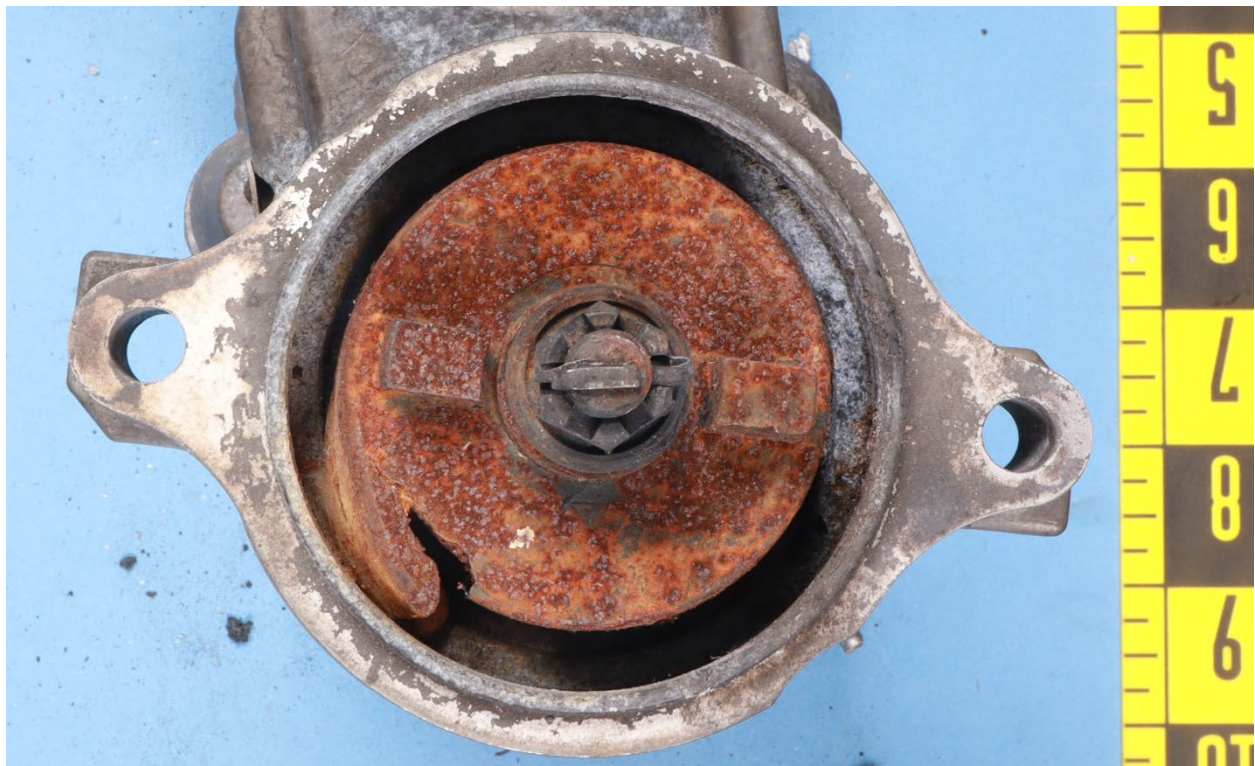
Figure 4. View of the opened end of the magneto with the impulse hub assembly, showing the cracked impulse coupling shell.
