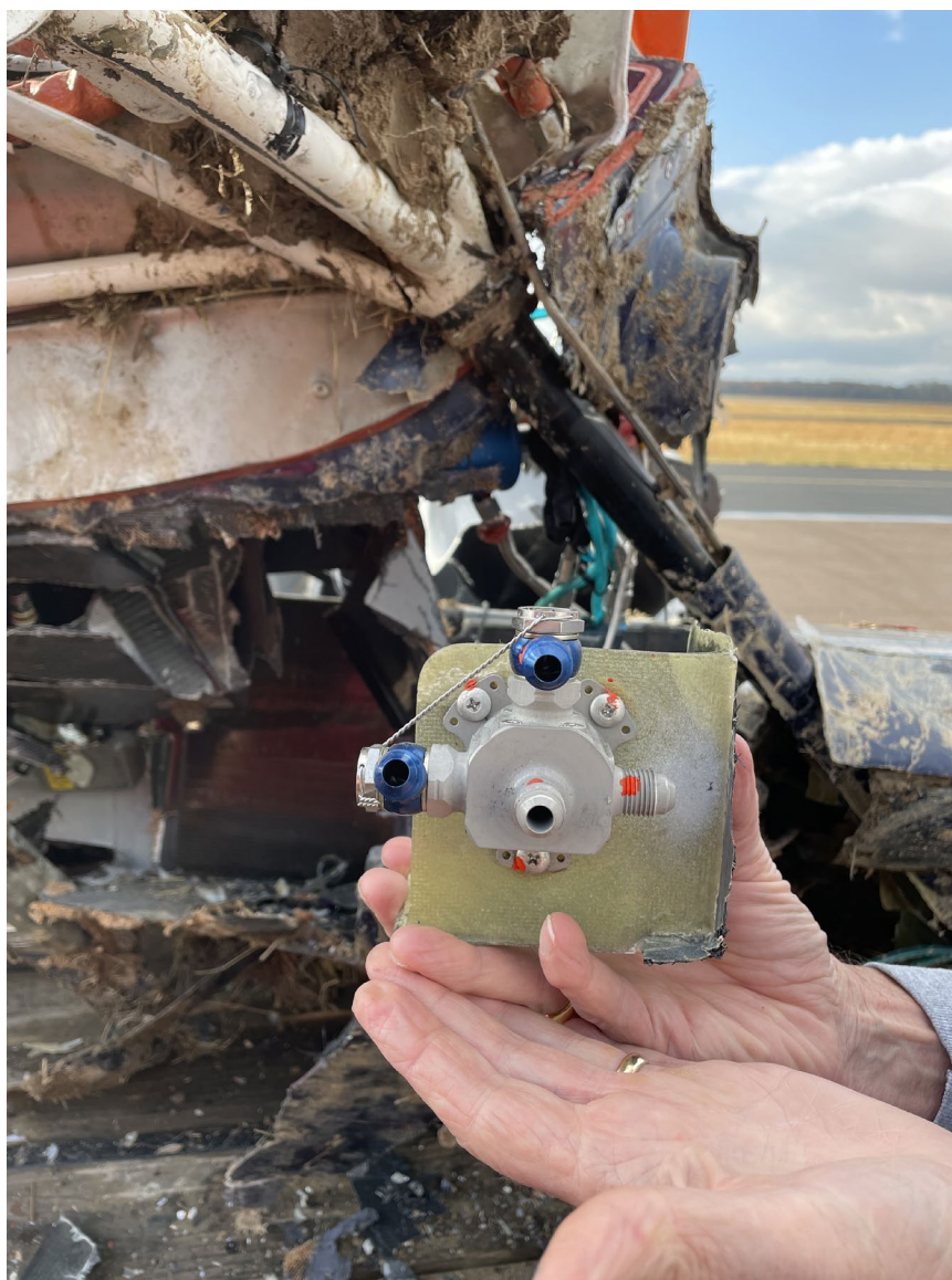
Photograph 3 - View of the fuel selector valve.
