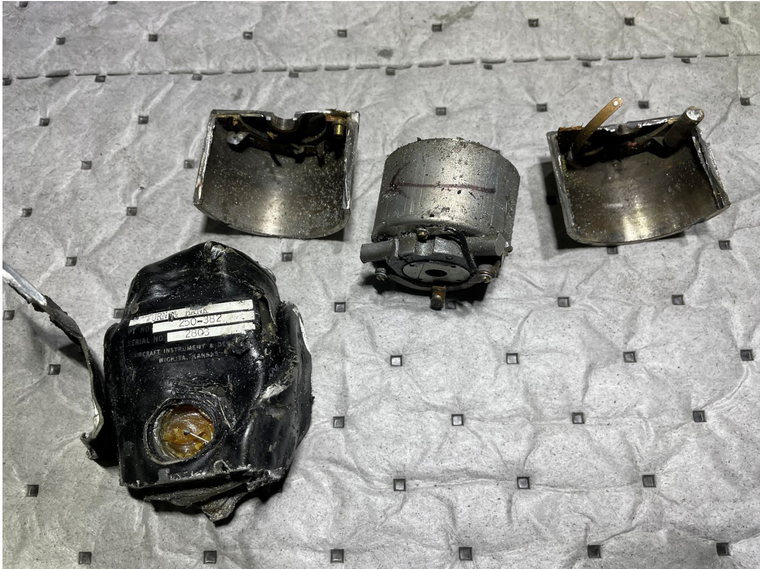
Photograph 6 – Turn and bank indicator after disassembly
