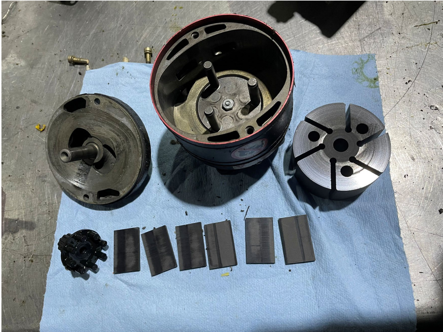
Photograph 4 – Vacuum pump after disassembly
