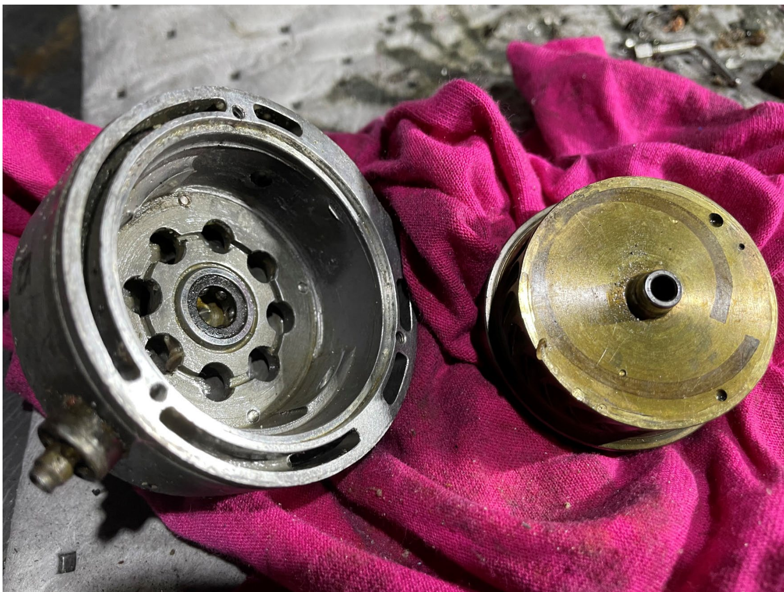
Photograph 5 – Attitude indicator gyro after disassembly
