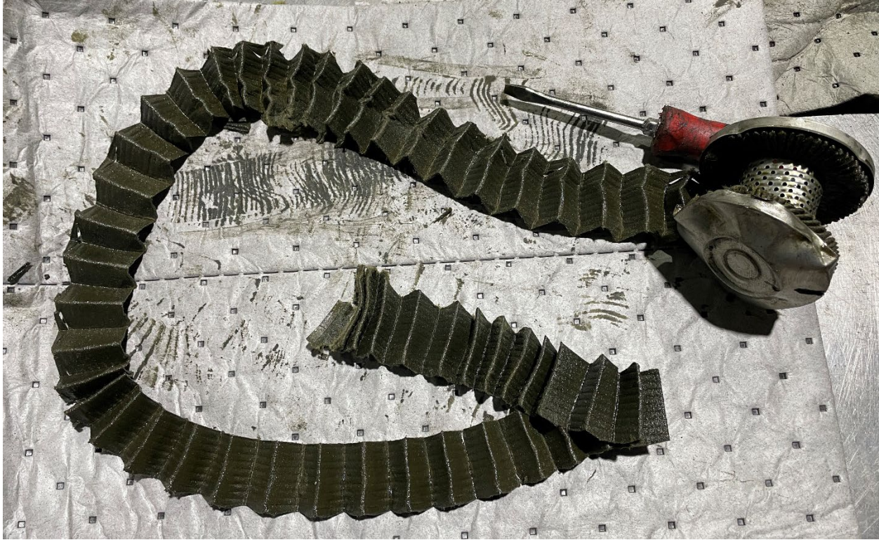
Figure 21. View of disassembled oil filter.
