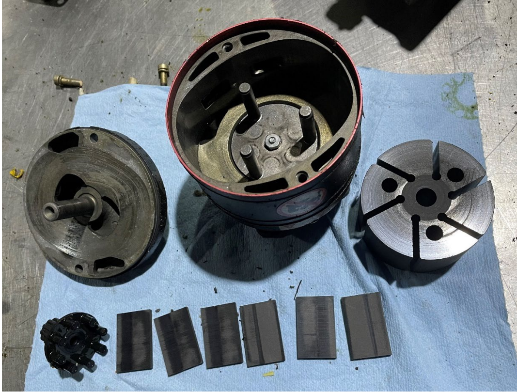
Figure 16. View of disassembled vacuum pump.
