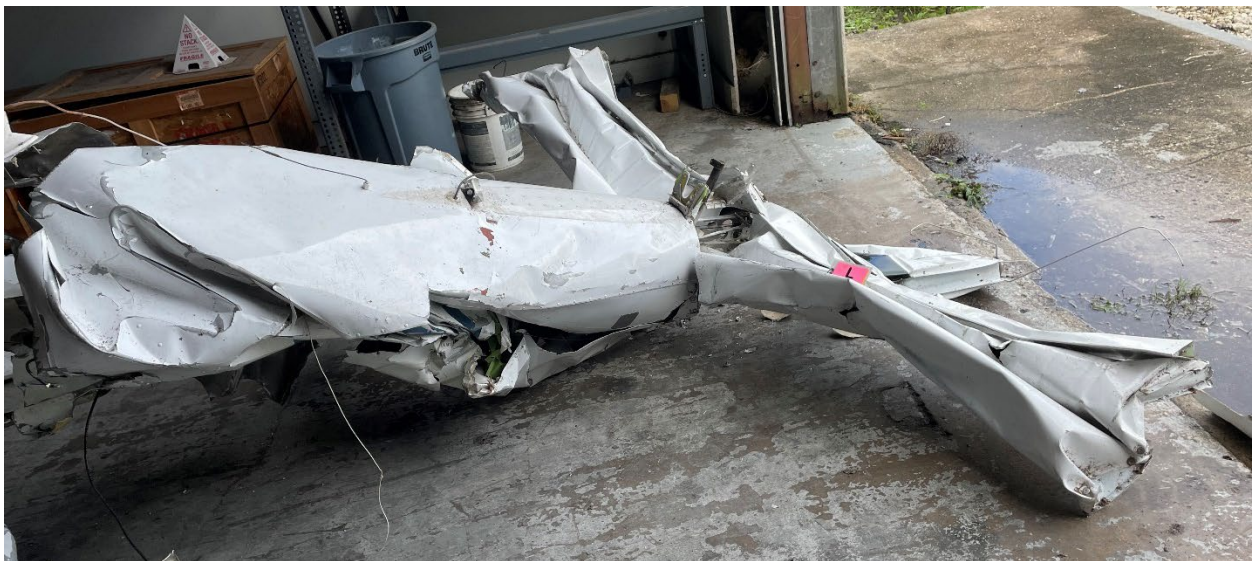
Figure 4. View of empennage.
