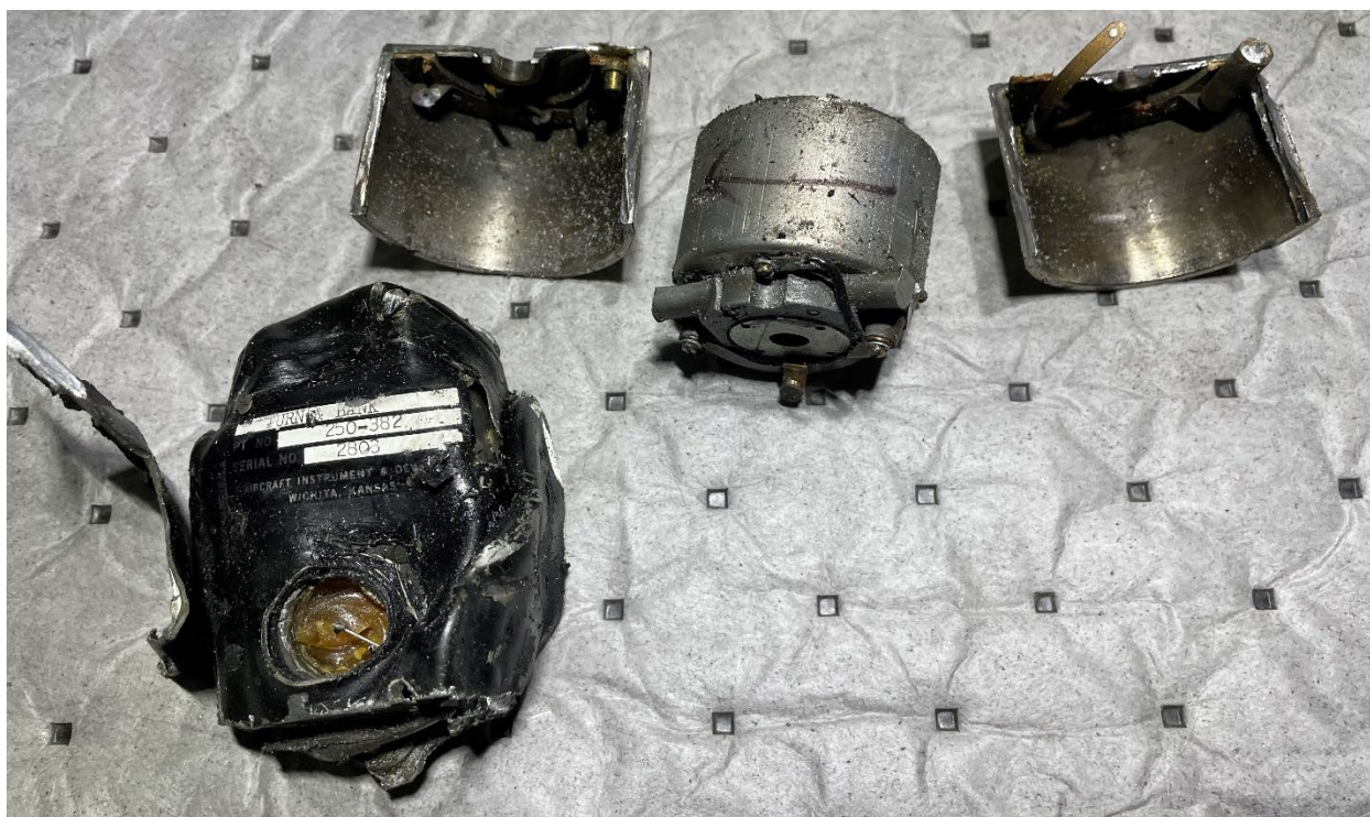
Figure 9. View of turn and bank electronic gyroscope and gyroscope housing.
