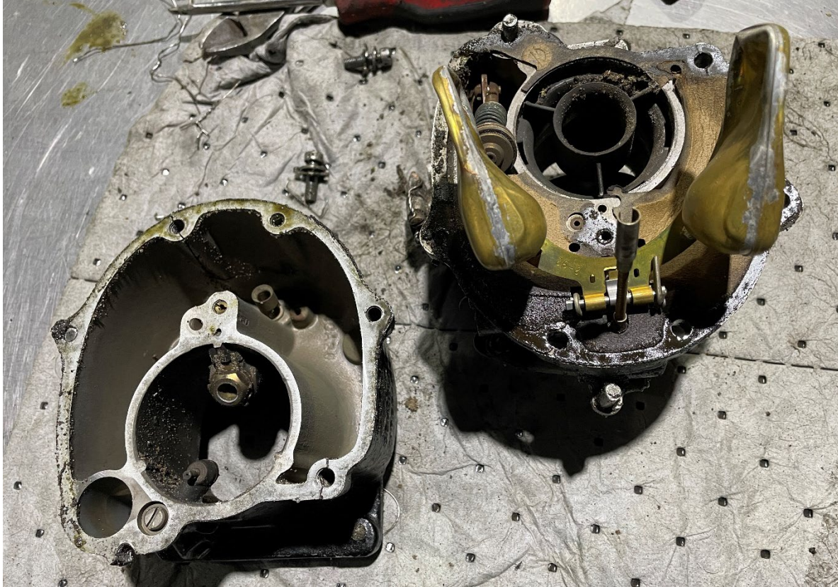
Figure 17. View of disassembled carburetor.
