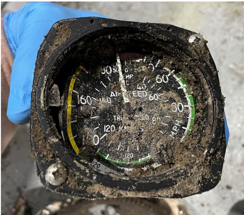
Figure 12. View of airspeed indicator as found. Note needle position.
