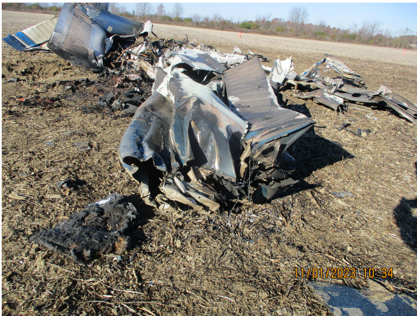
Photograph 2 - Left wing, Note: accordion crushing
