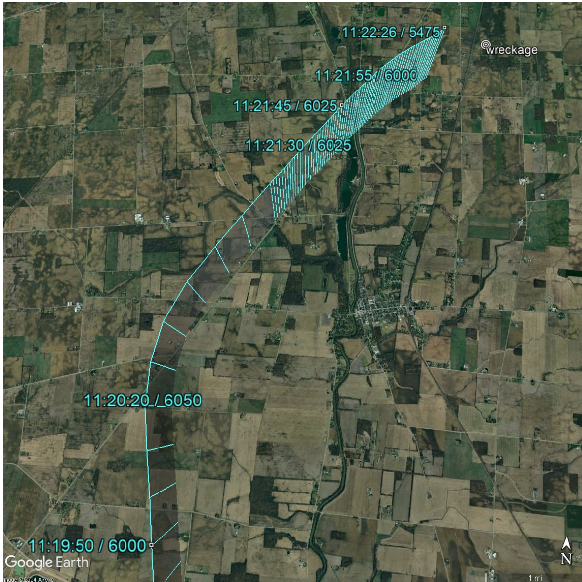
Figure 5. End ADS-B flight path with selected times and altitudes notated. Data before 11:18:00 is shown every 10 seconds. Data after 11:18:00 is shown at the full ADS-B resolution of 1 Hz.
