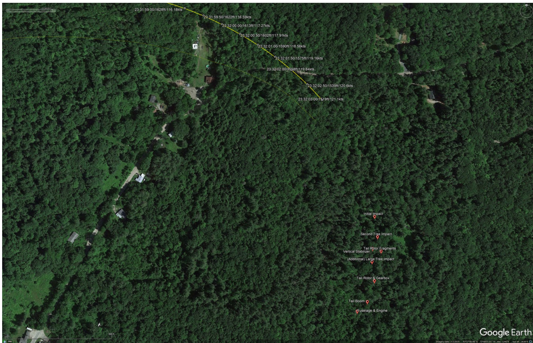
Figure 3. Google Earth overlay showing the final 4 seconds of recorded data, points of impact, and location of wreckage.
