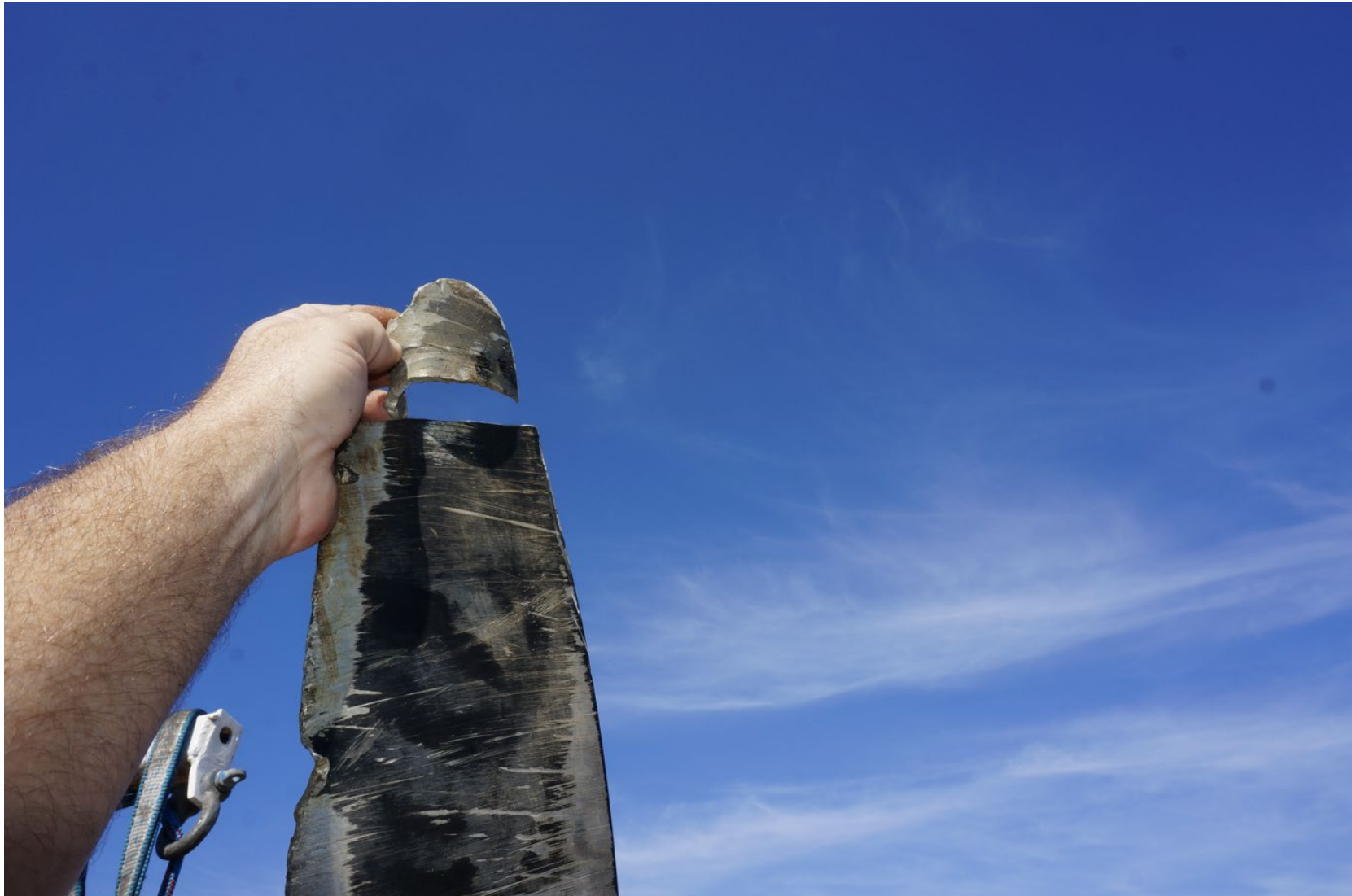
Photograph 14 - Tip from Second Propeller Blade
