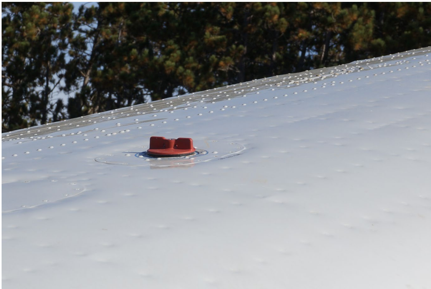
Photograph 34 - Left Wing Fuel Tank Filler Port
