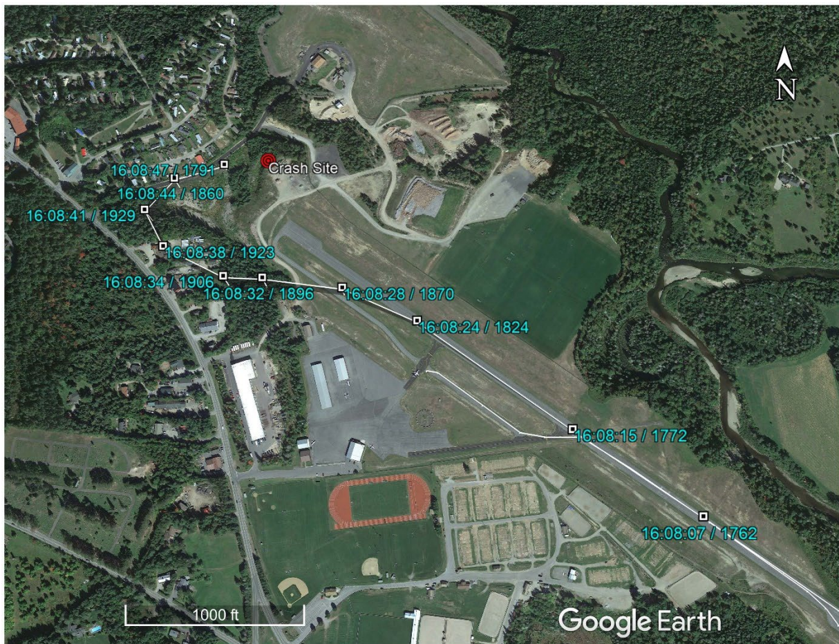
Figure 1. Overhead view of the flight path on a Google Earth background. Annotations indicate the time EDT (hh:mm:ss) and recorded altitude (ft). The crash site is indicated by the red circle.
