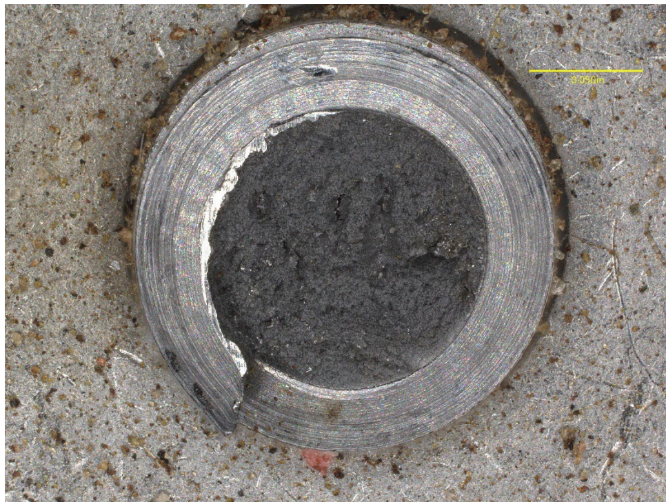
Figure 5. Fracture surface on the threaded section of the throttle arm.
