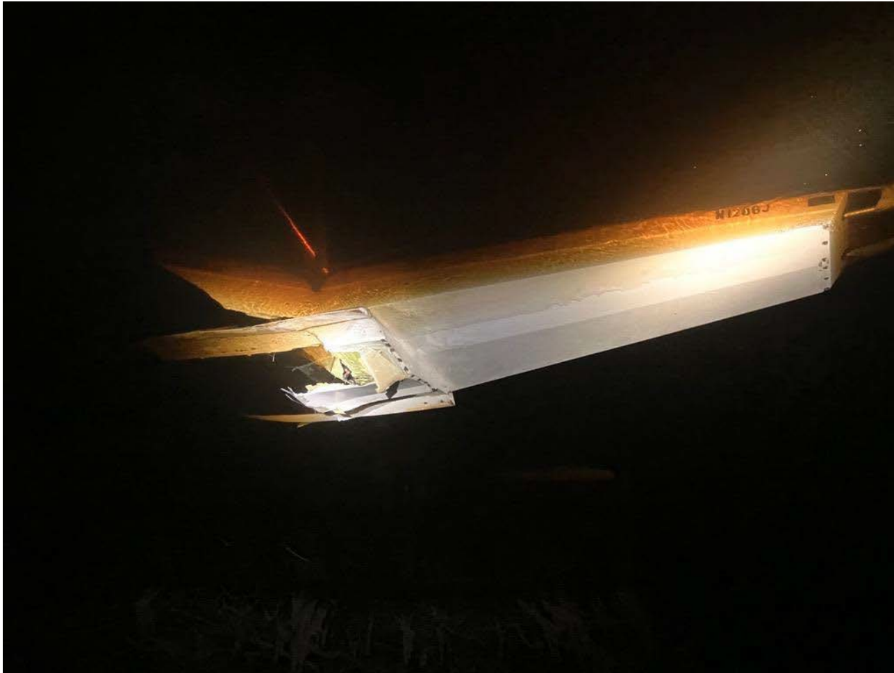
Photograph 2 - View of submerged and damaged float. (Courtesy of Wakulla County)
