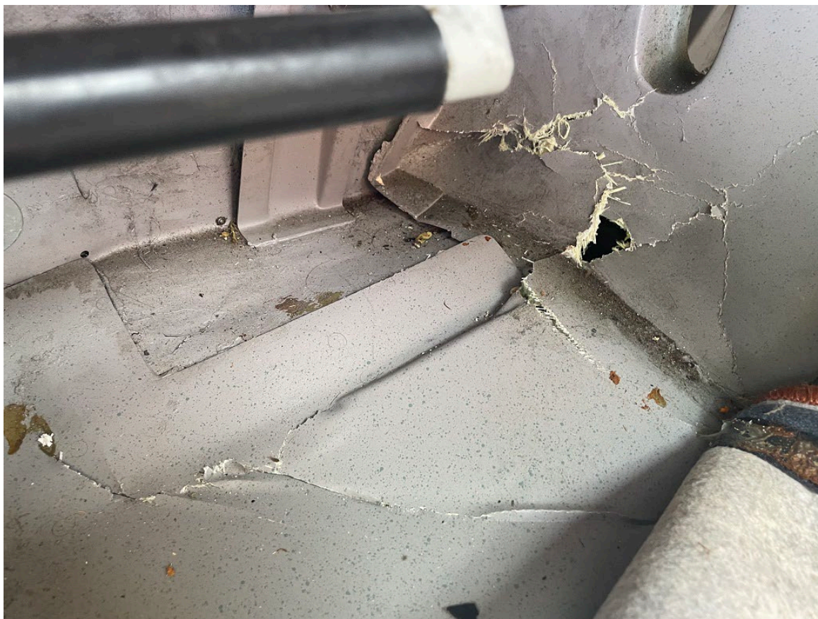
Photograph 3 - Lower Fuselage Composite Damage (Courtesy of FAA)
