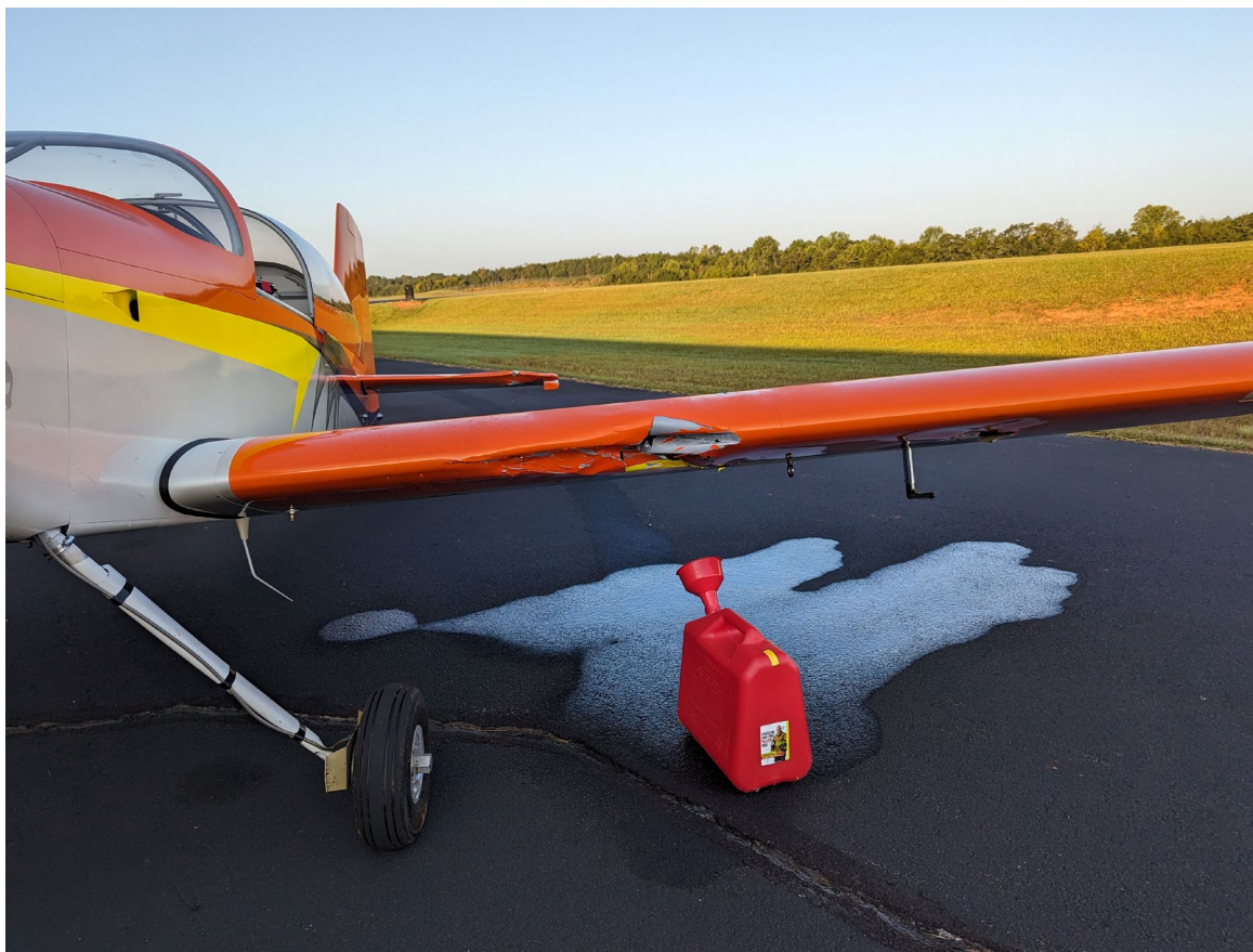
Photograph 1 - Overview of damage to the left wing. (Courtesy of FAA)
