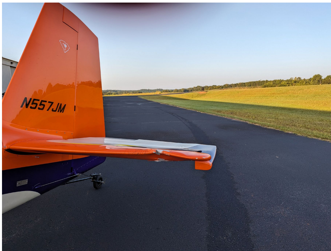
Photograph 4 - View of damage to the left horizontal stabilizer. (Courtesy of FAA)
