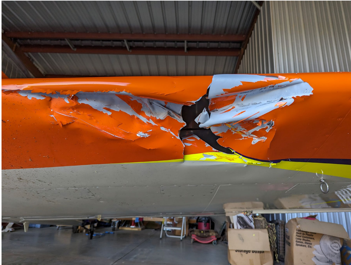
Photograph 2 - View of damage to the left wing leading edge. (Courtesy of FAA)
