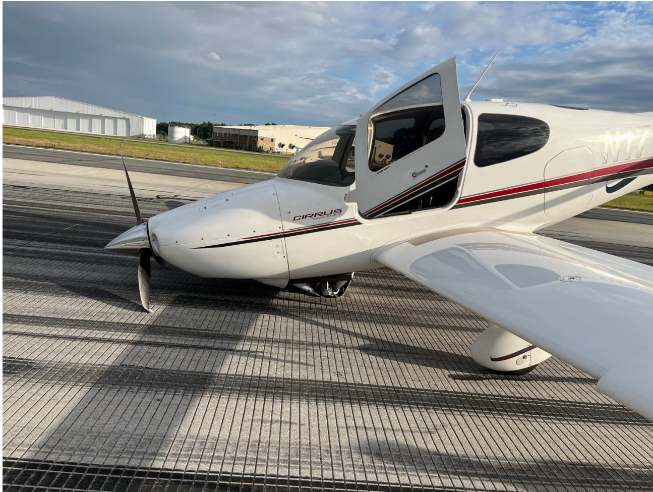
Photograph 1 - View of left side of airplane with collapsed nose landing gear. (Courtesy of Pilot)
