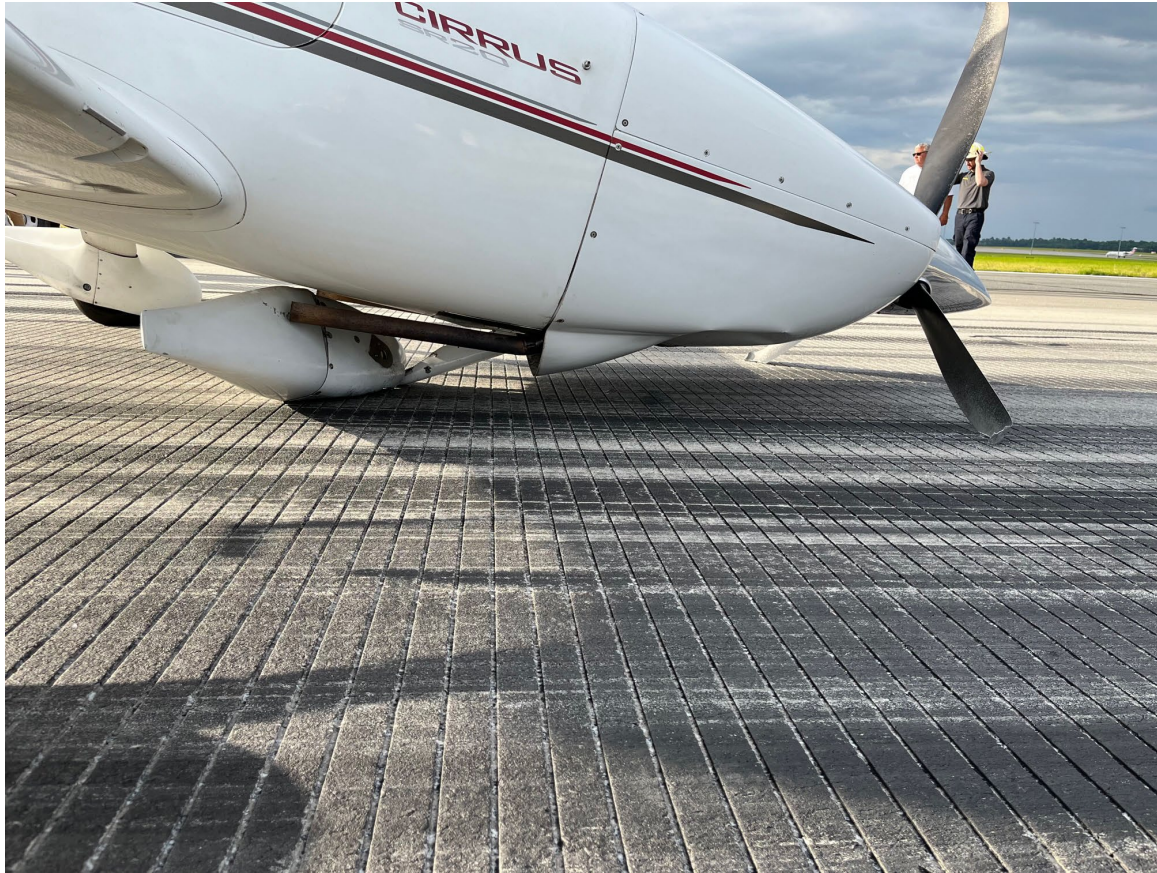
Photograph 2 - View of right side of airplane with closeup view of nose landing gear damage. (Courtesy of Pilot)
