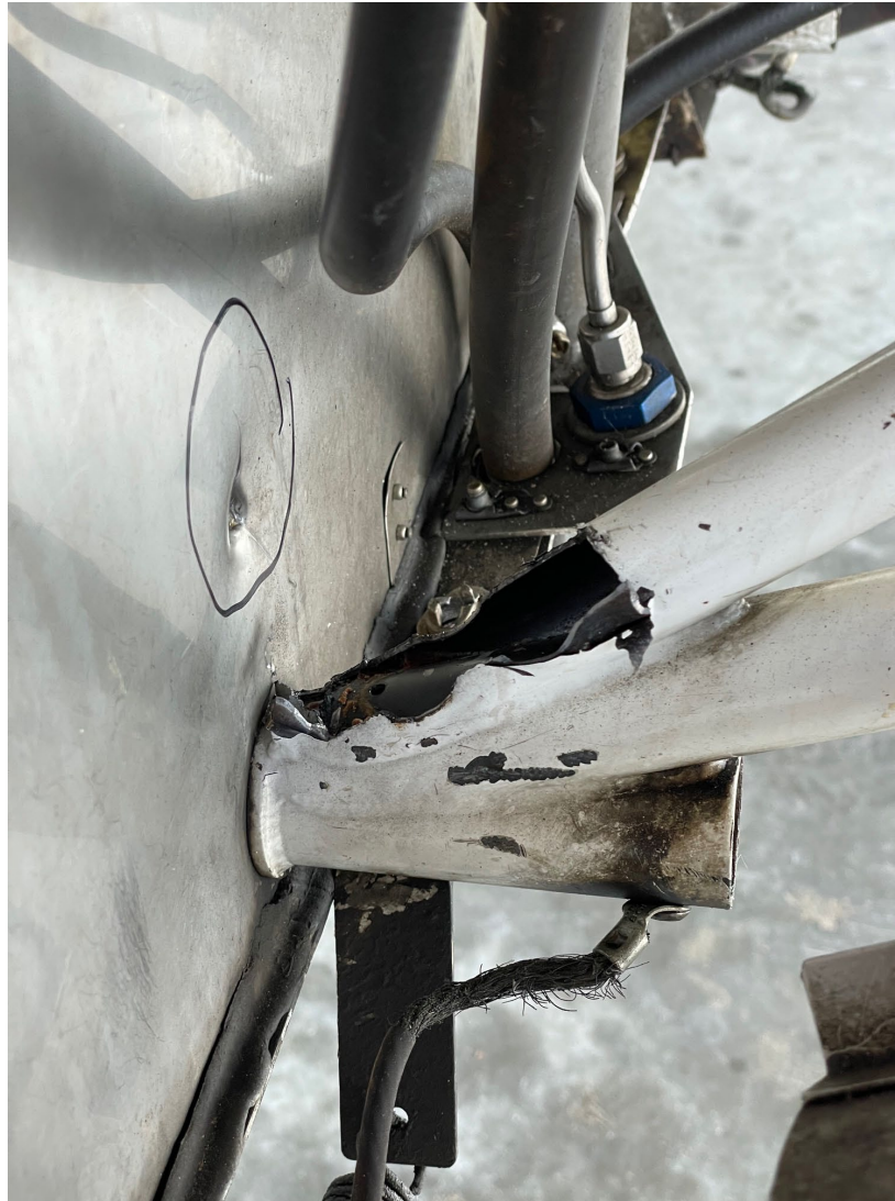
Photograph 3 - Closeup view of firewall puncture and engine mount damage (Courtesy of Savannah Aviation)
