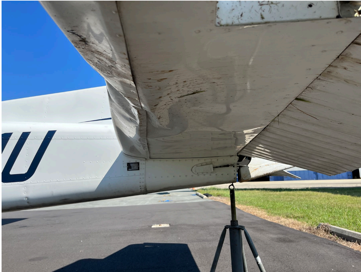
Photograph 3 - View of damage to the left horizontal stabilizer. (Courtesy of FAA)
