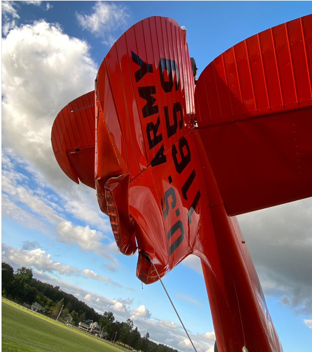
Photograph 2 - View of damaged empennage (Courtesy of FAA)
