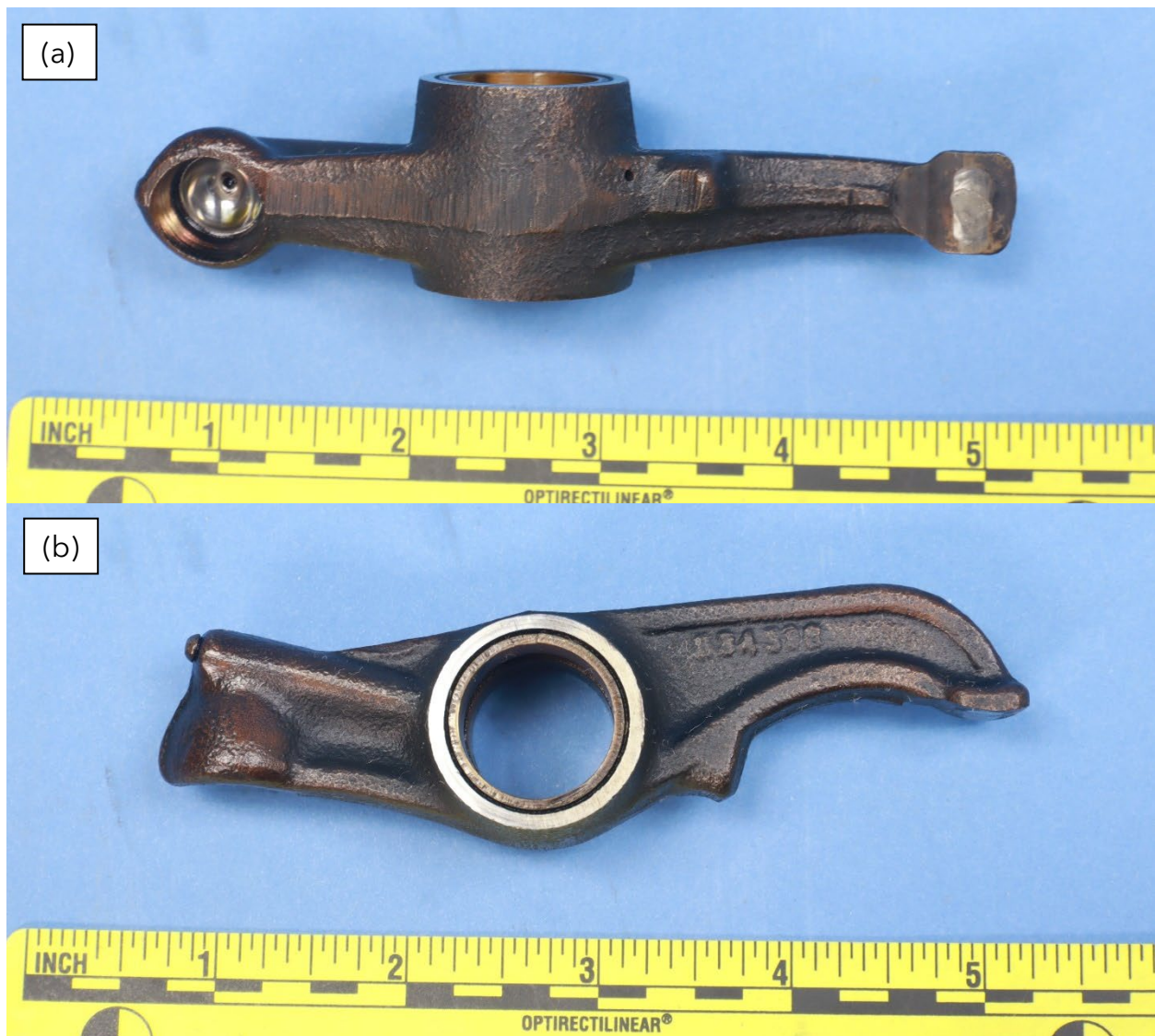
Figure 2. View of the rocker arm from (a) the underside with contact surfaces and (b) the side showing the casting markings and internal bushing.
