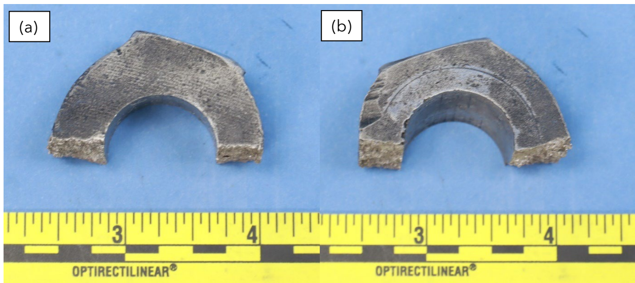
Figure 6. The loose cylinder housing from (a) the outboard and (b) inboard faces.
