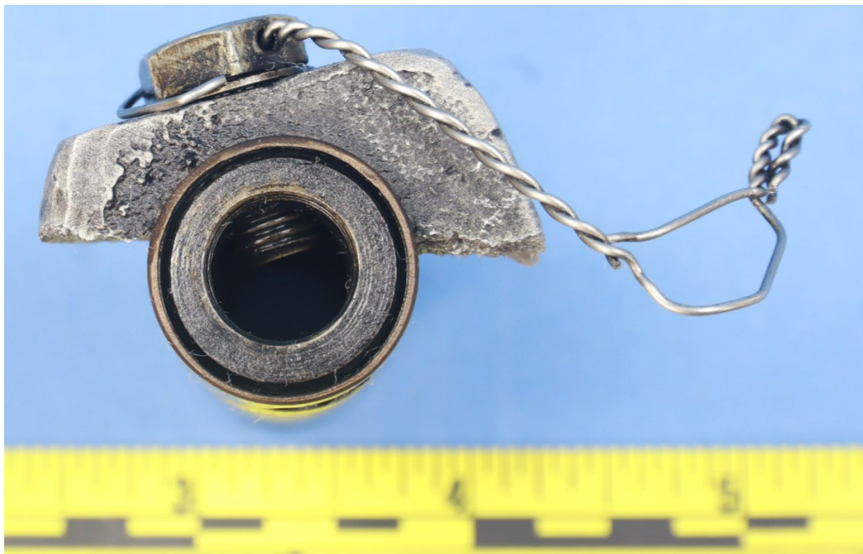
Figure 4. End of the rocker arm shaft attached to a fractured cylinder housing fragment.
