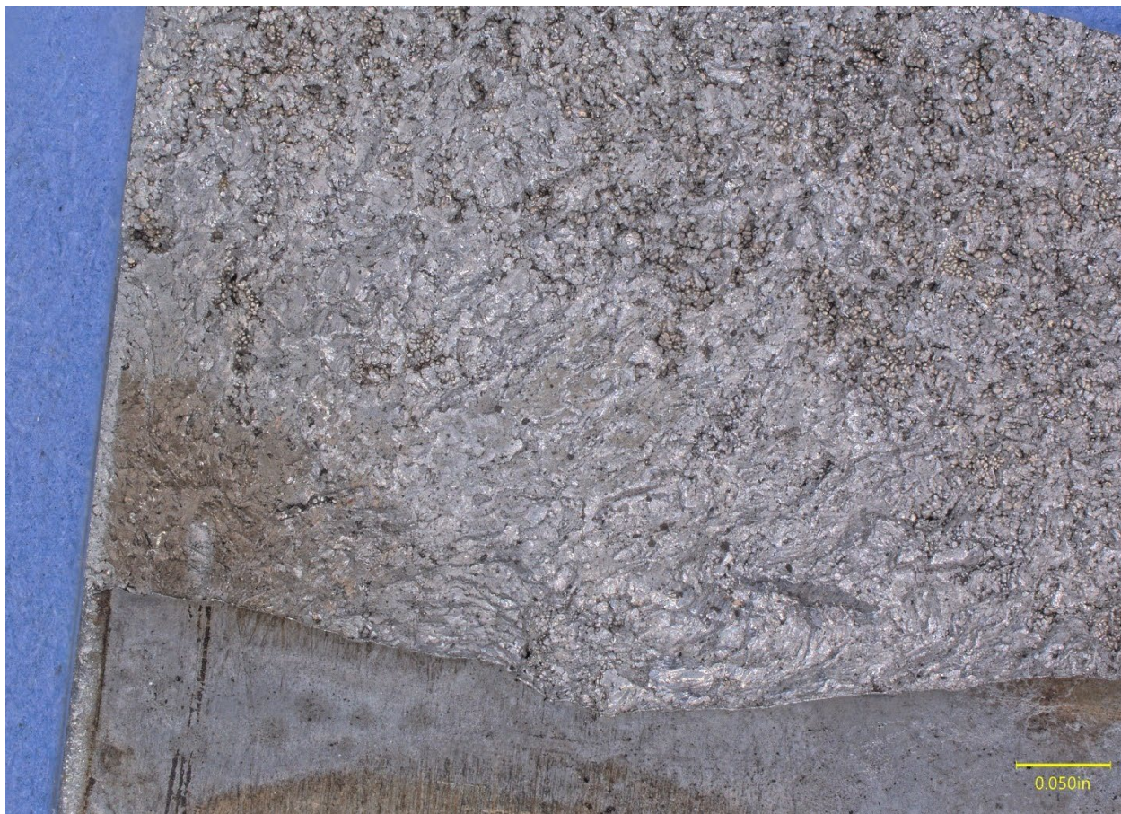
Figure 8. View of an inward corner of the left fracture surface in Figure 7, showing a darker triangular region on the fracture surface.
