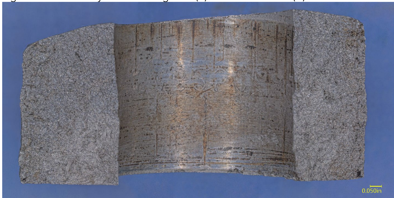
Figure 7. View of the loose housing fragment fracture surfaces, after cleaning.
