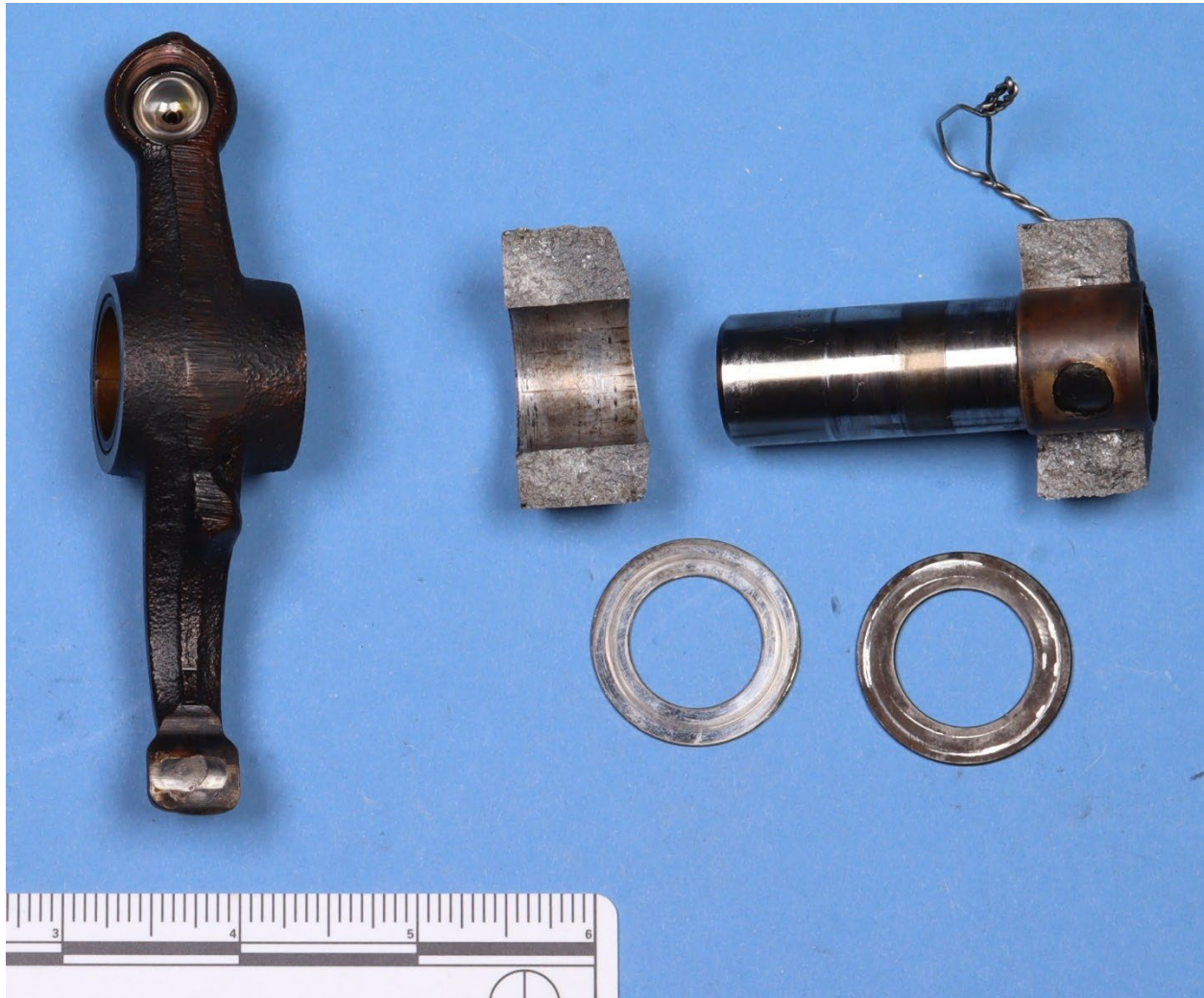
Figure 1. The pieces submitted from the accident, including a rocker arm, two fractured sections of cylinder housing, the adjacent shaft bolted to the right fragment with safety wire, and two washer/spacers.
