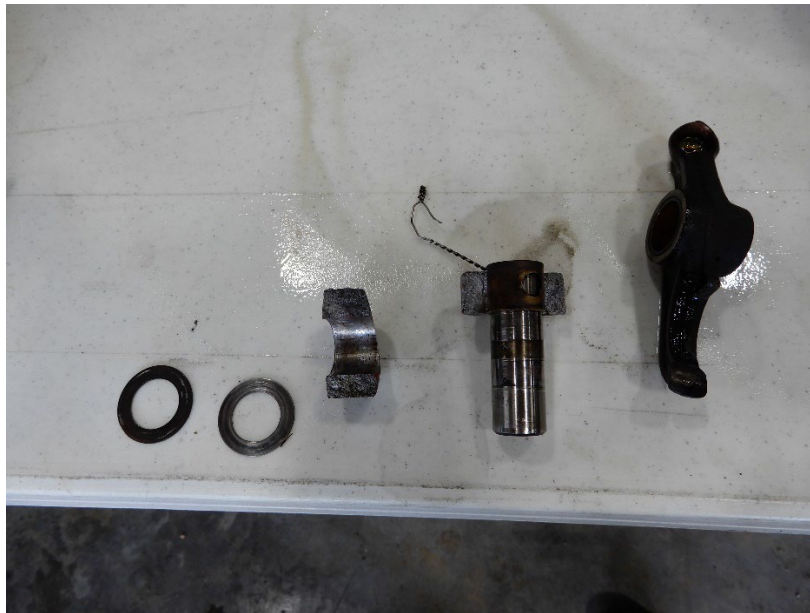
Photo 2 - Loose Parts Found inside No. 6 Cylinder Head Rocker Cover
