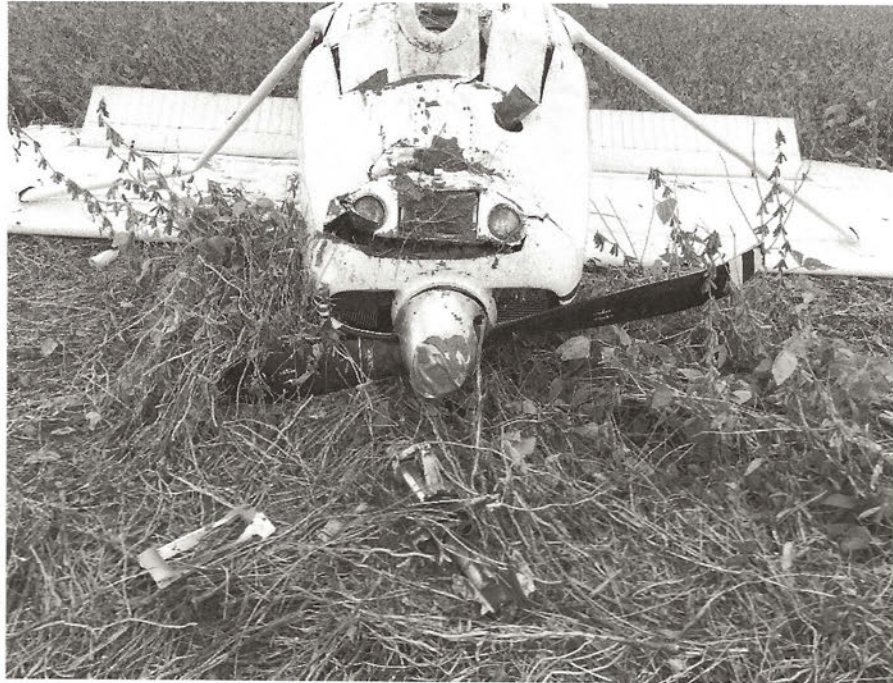
Figure 7 View looking at nose of aircraft. Nose landing gear strut in front of spinner in grass.
