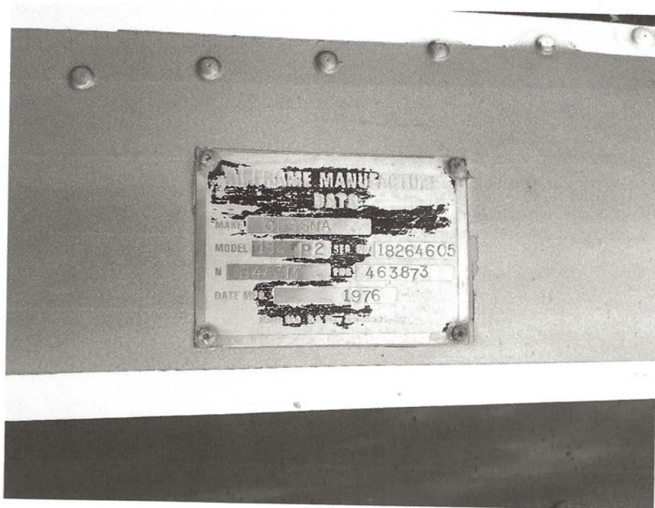
Figure 17 Aircraft data plate.
