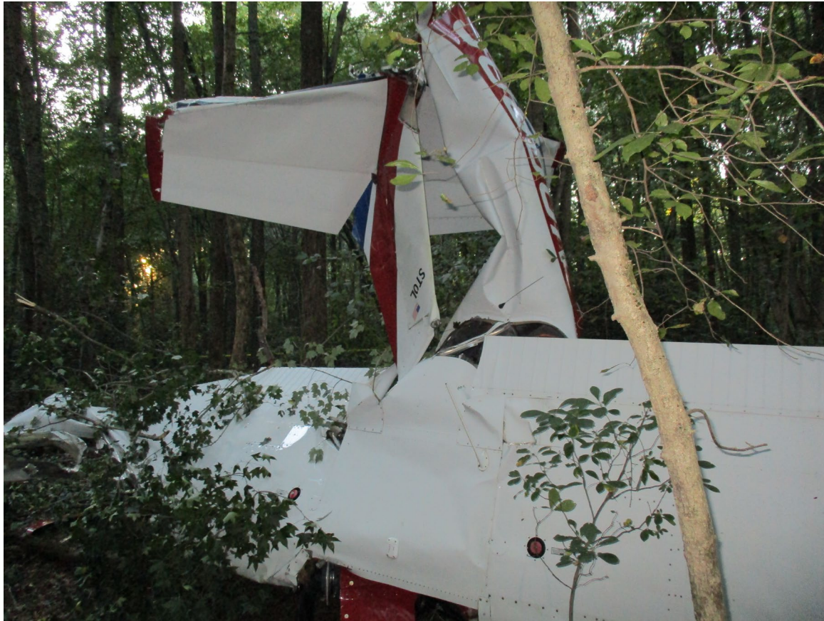
Photograph 2 - Top view of airplane showing fuselage and empennage damage (Courtesy of FAA)
