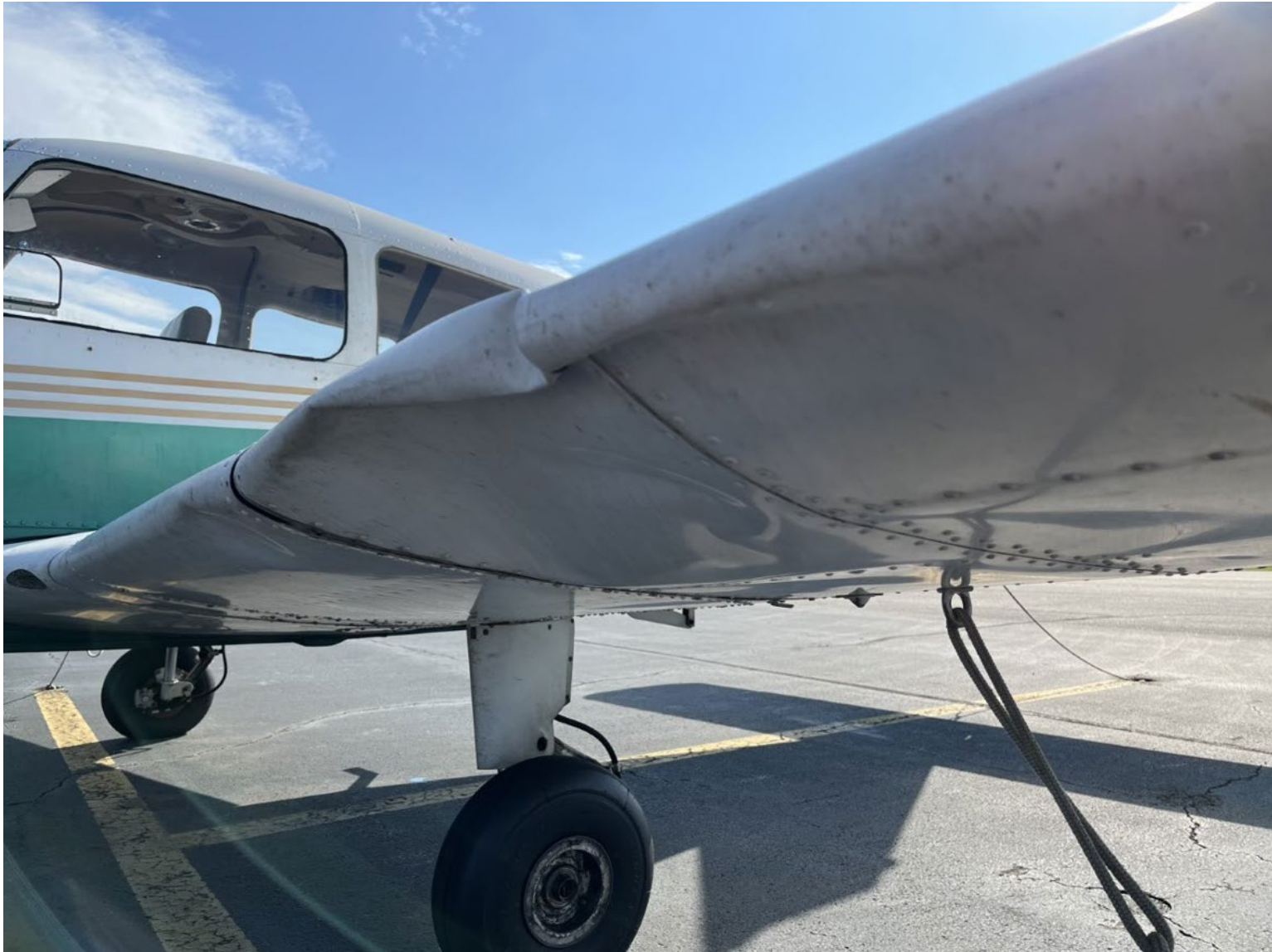
Photograph 2 - Side view of wing damage (Courtesy of FAA Inspection)
