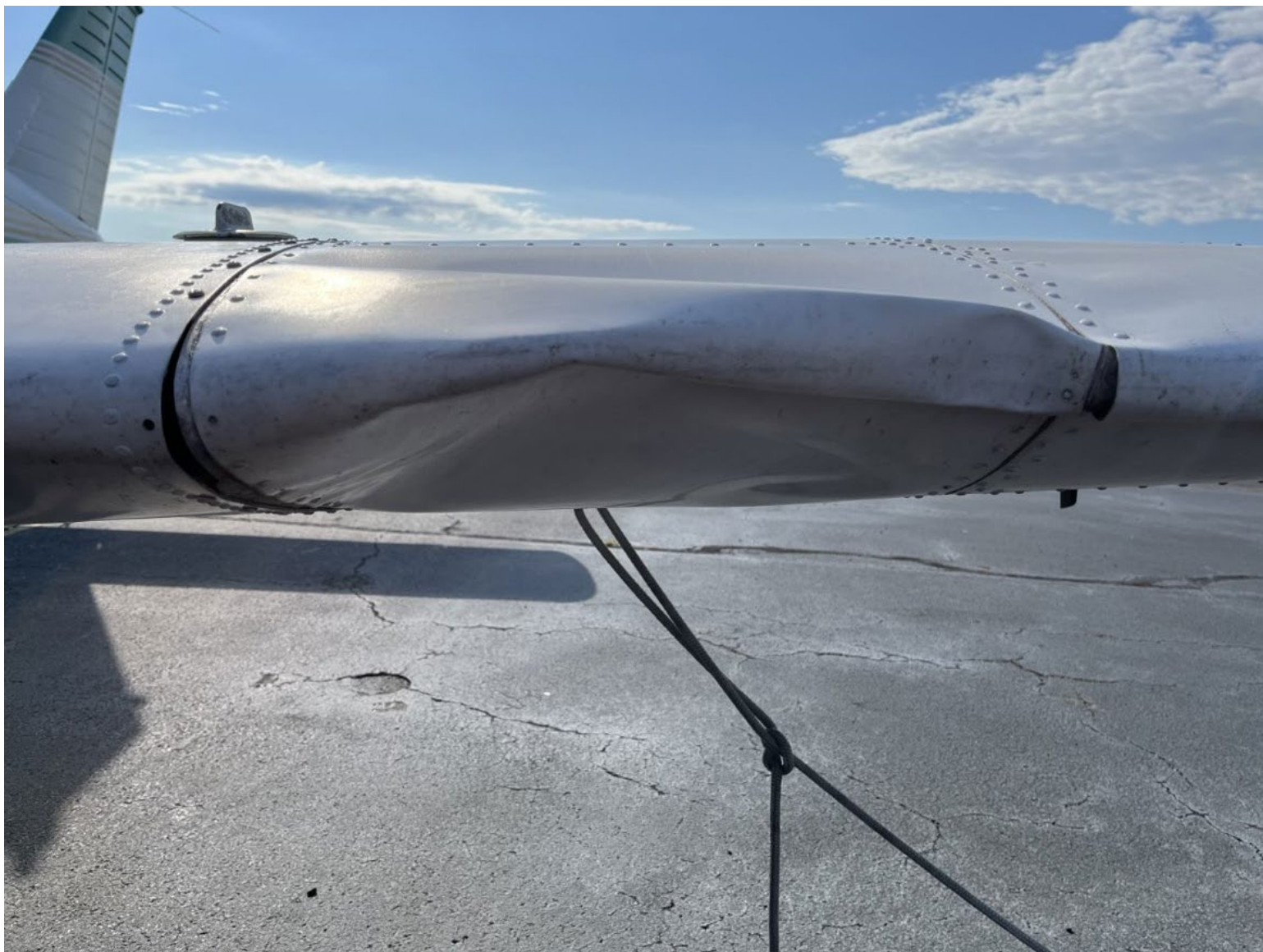
Photograph 3 - Close view of wing damage. (Courtesy of FAA Inspector)
