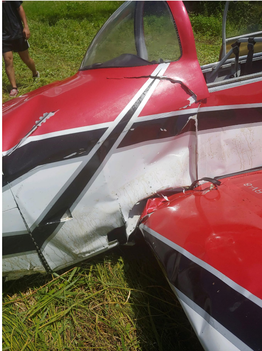
Photograph 3 - View of damage to the left side of the fuselage. (Courtesy of FAA)
