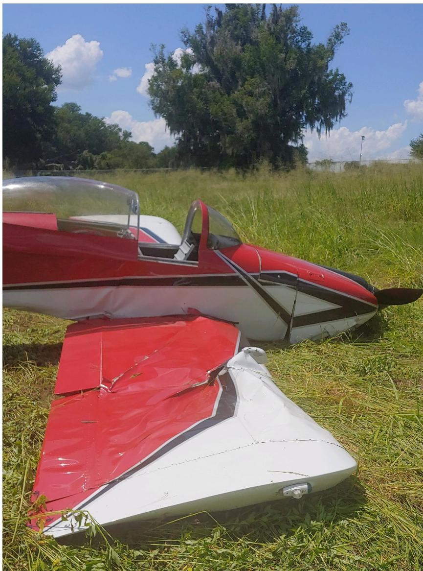
Photograph 2 - View of damage to the right wing and fuselage (Courtesy of FAA)
