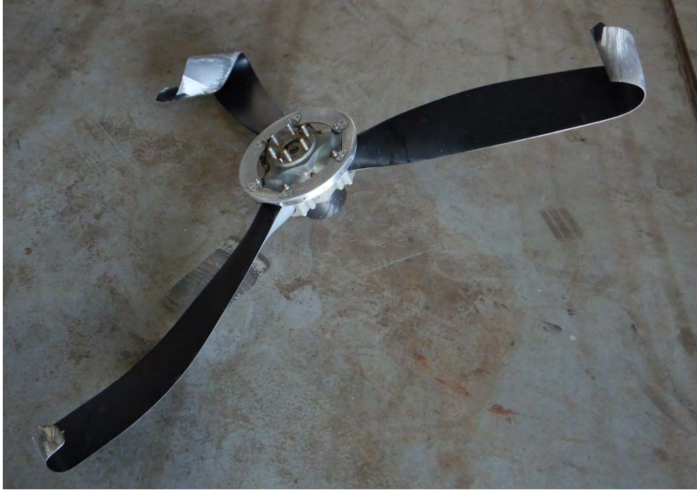
Photo 26 - Propeller with tip curling and chordwise abrasion on all blades.
