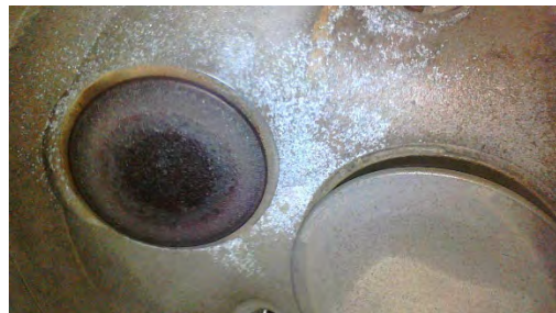
Photo 16 - No. 3 cylinder exhaust and intake valves.
