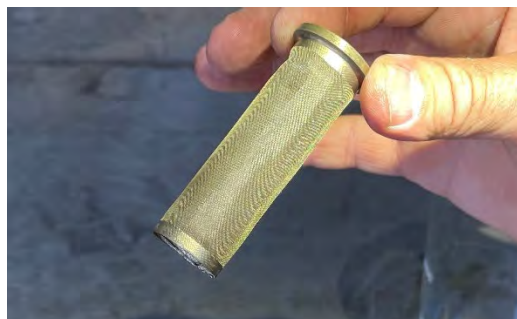
Photo 10 - Fuel strainer screen free of debris.
