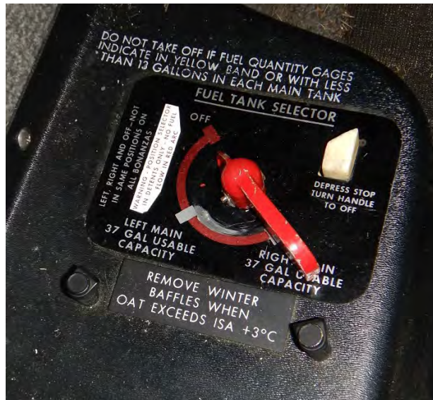
Photo 8 - Fuel selector in OFF position prior to examination.
