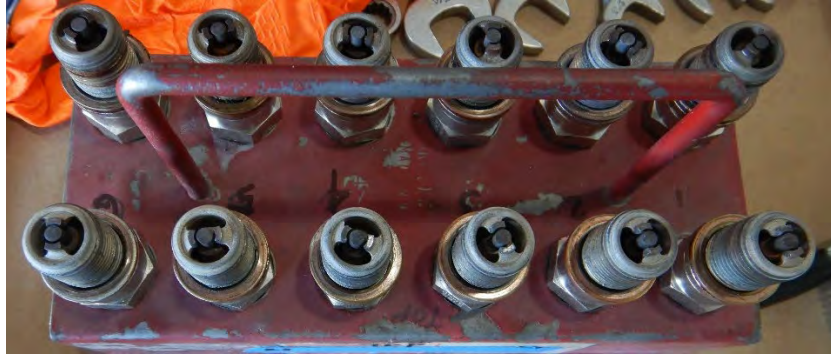
Photo 12 - Spark plugs showing normal wear.
