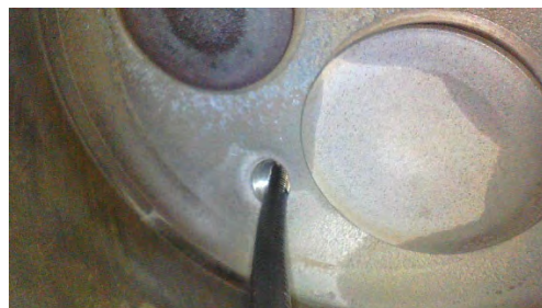
Photo 18 - No. 5 cylinder exhaust and intake valves.
