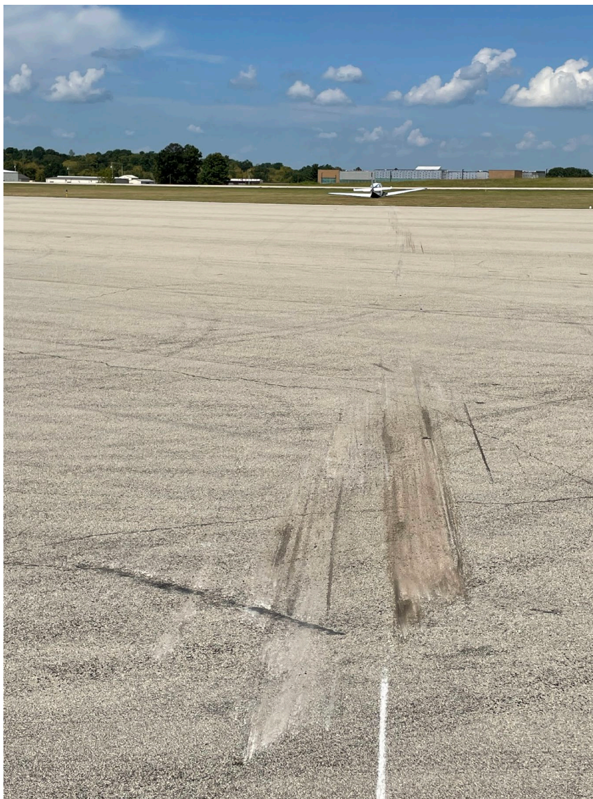
Photograph 5 - View of runway scars leading to airplane. (Courtesy of FAA)
