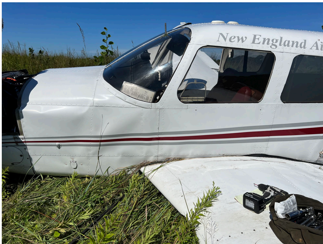
Photograph 3 - View of left side of fuselage buckling. (Courtesy of Operator)
