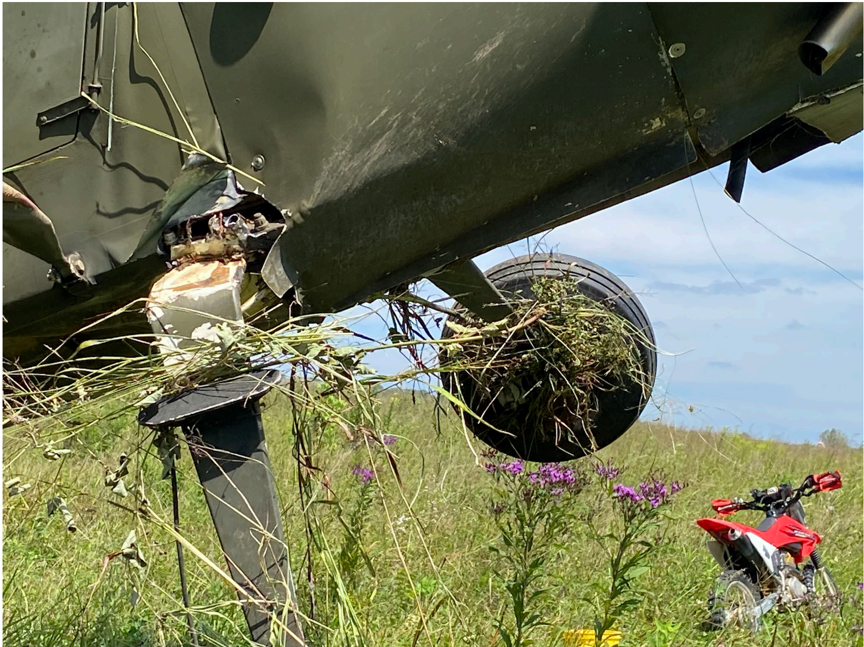
Photo 2 – View of Right Main Landing Gear Structure (FAA)
