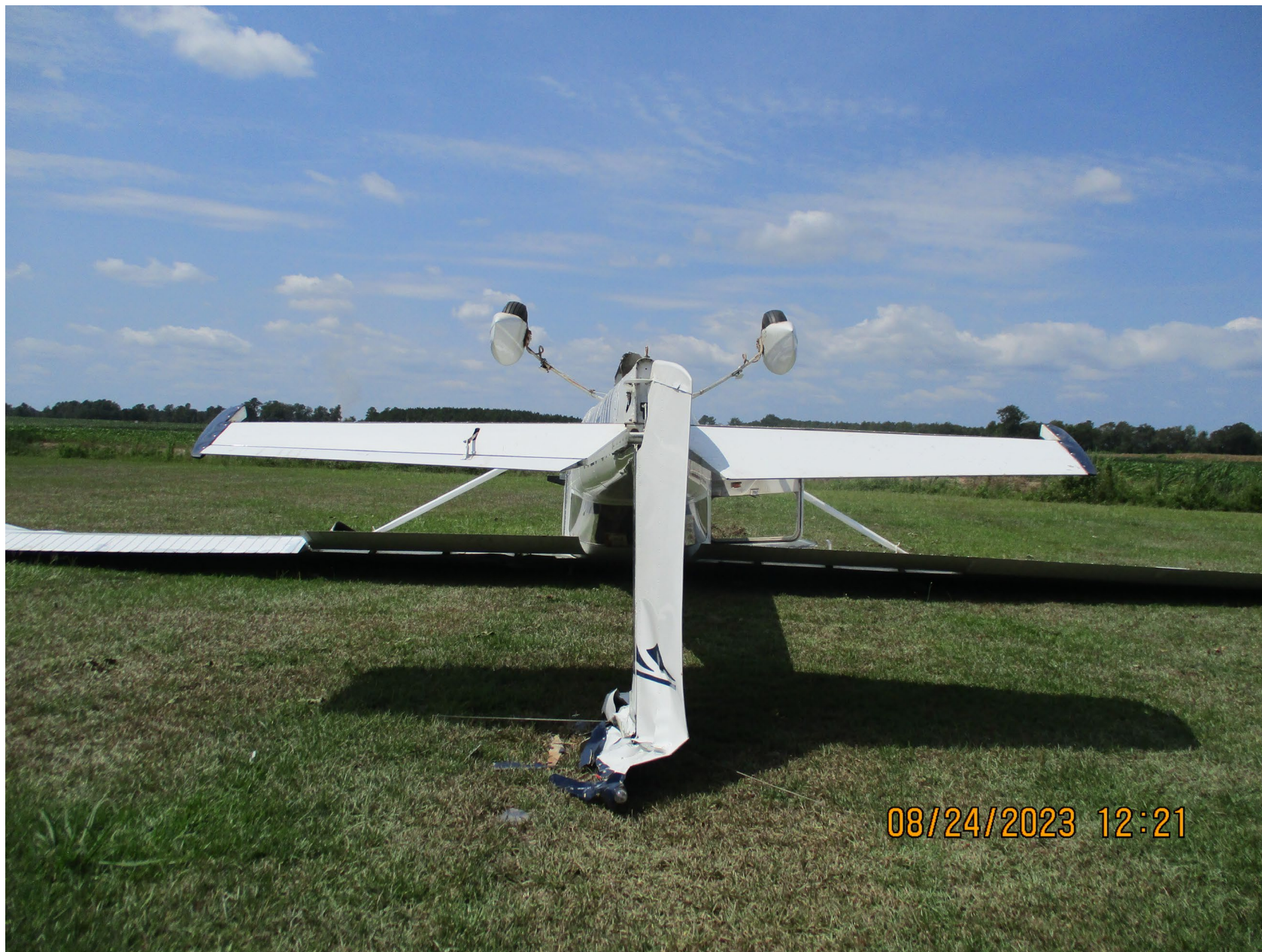
Photo 4 - FAA Digital Photograph. Aft View of the Inverted Airplane. Note the Structural Damage to the Vertical Stabilizer.
