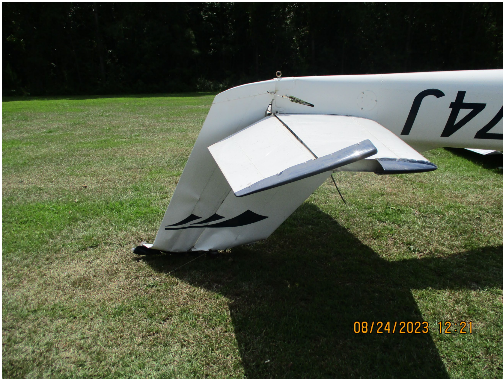
Photo 3 - FAA Digital Photograph. Left Side View of the Aft Empennage of the Inverted Airplane. Note the Structural Damage to the Vertical Stabilizer.
