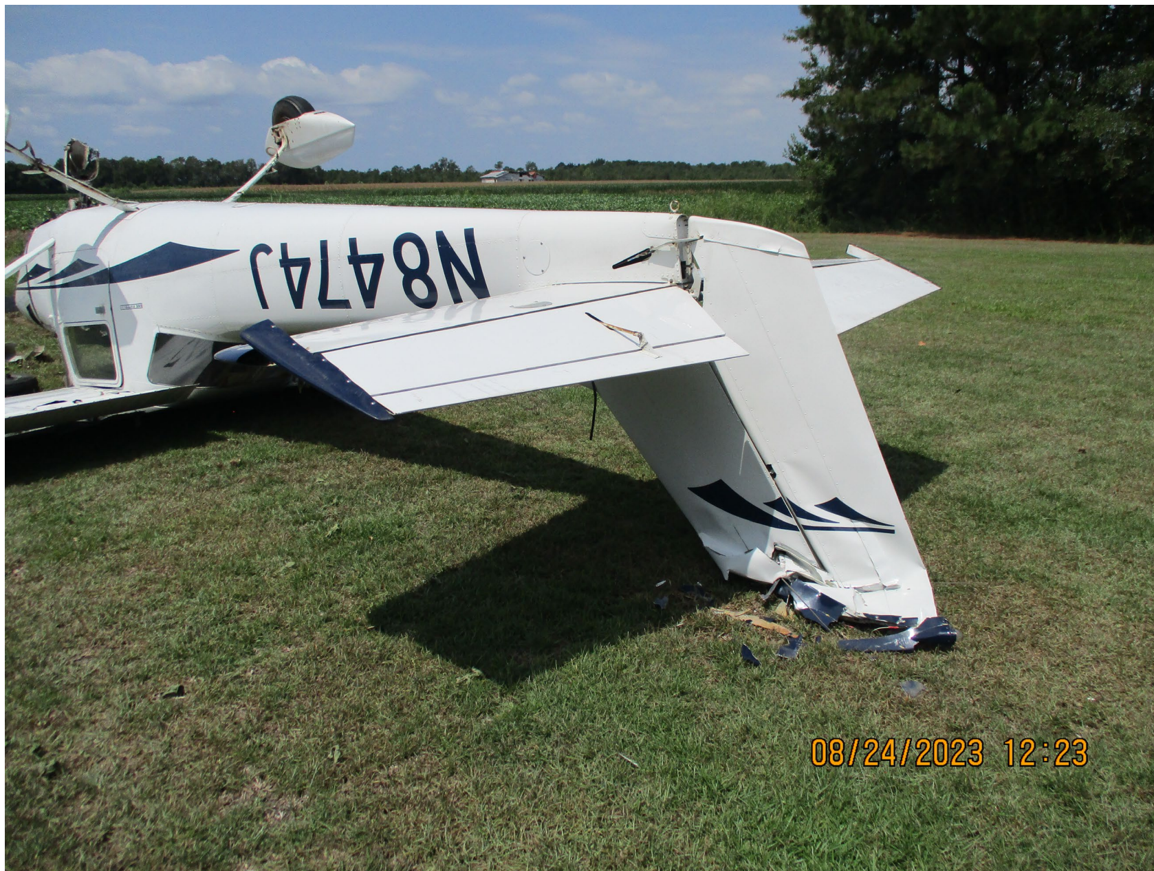
Photo 5 - FAA Digital Photograph. Right Aft Quartering View of the Inverted Airplane Showing the Fuselage, Portion of the Right Wing, Vertical and Horizontal Stabilizers with Control Surfaces. Note the Structural Damage to the Vertical Stabilizer.
