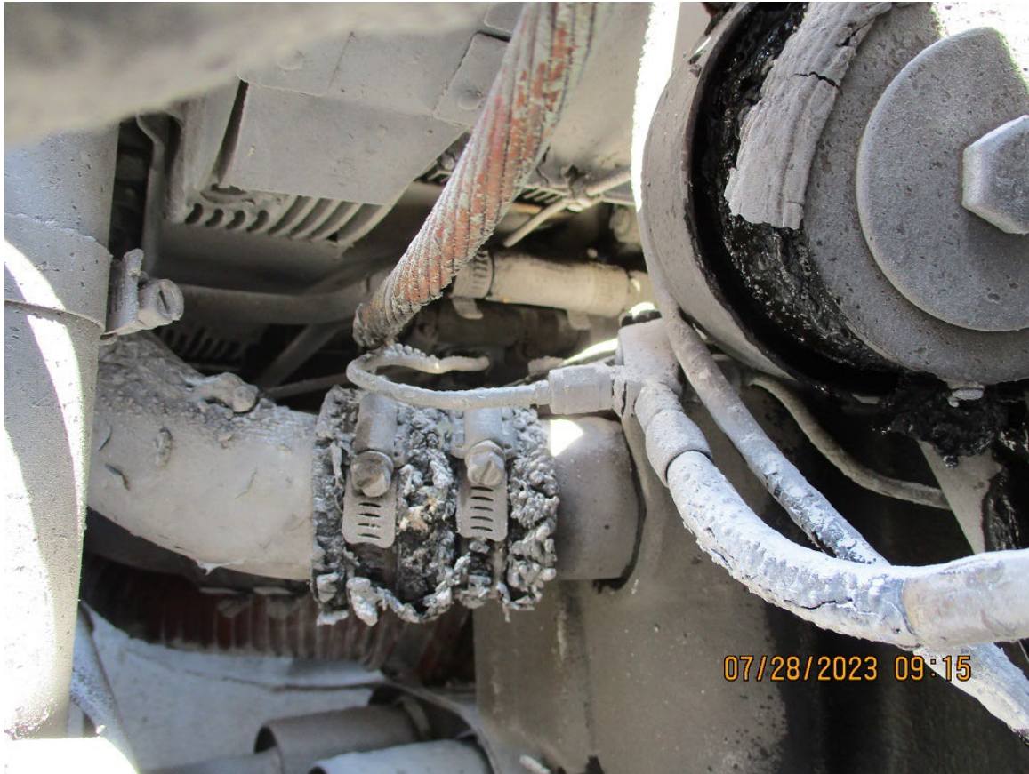
Photograph 2 - Starter Motor Electrical Lead And Fuel Primer Line (Courtesy of FAA)
