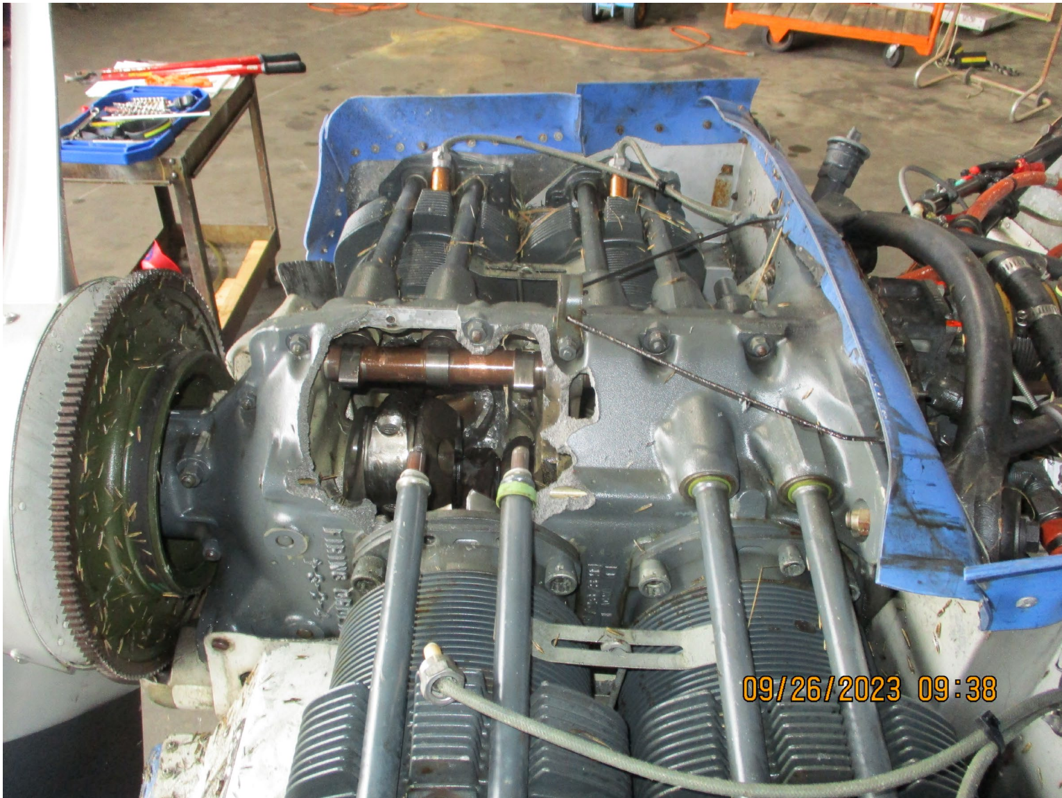
Photograph 2 - Engine, hole in #2 cylinder case
