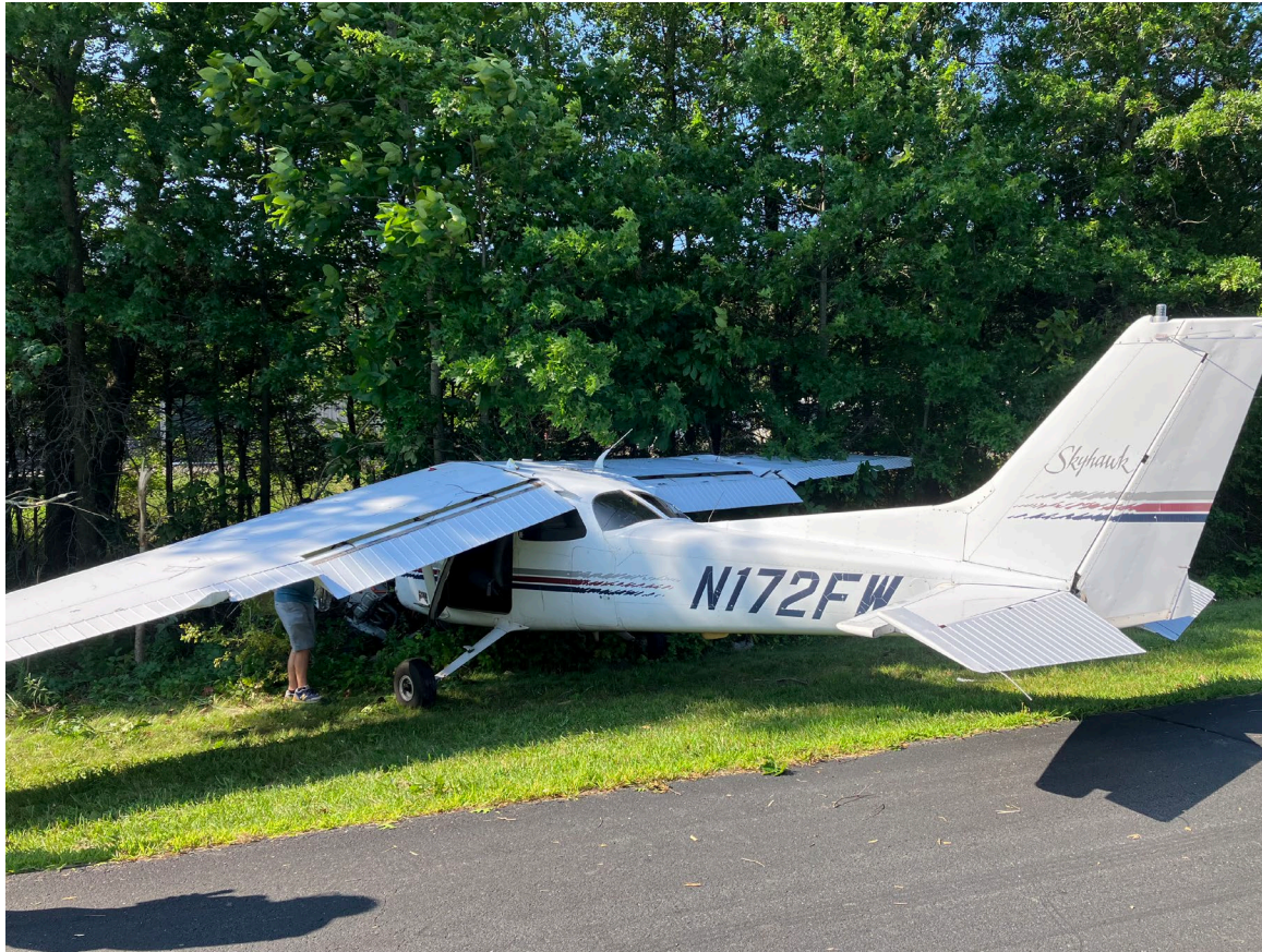
Photograph 1 - Left side of airplane showing damaged left wing. (Courtesy of FAA)
